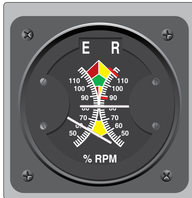
Figure 4-19. A "split" or divided needle condition is a result of a sudden loss of engine power.
