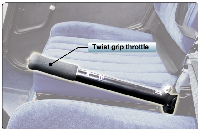
Figure 3-2. A twist grip throttle is usually mounted on the end of the collective lever. The throttles on some turbine helicopters are mounted on the overhead panel or on the floor in the cockpit.
