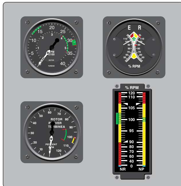
Figure 4-18. Various types of dual-needle tachometers.
