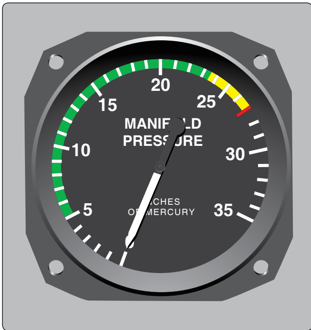
Figure 5-5. The manifold pressure gauge is an engine instrument typically used in piston aircraft engines to measure the pressure inside the induction system of an engine. Manifold pressure is a measurement of vacuum and the measurement is taken at the intake manifold.
