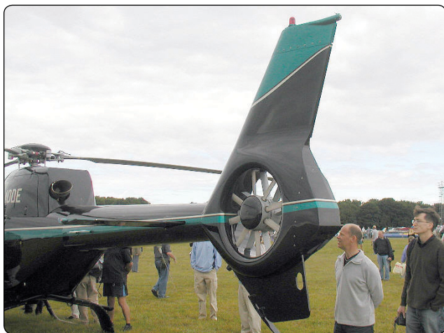
Figure 4-14. Fenestron or “fan-in-tail” antitorque system. This design provides an improved margin of safety during ground operations.
