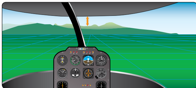
Figure 9-1. Maintain straight-and-level flight by adjusting the rotor tip-path plane forward but adjusting the collective as necessary to maintain a constant airspeed and altitude. The natural horizon line can be used as an aid in maintaining straight-and-level flight. If the horizon line begins to rise, slight power may be required or the nose of the helicopter may be too low. If the horizon line is slowly dropping, some power may need to be taken out or the nose of the helicopter may be too high, requiring a cyclic adjustment.
