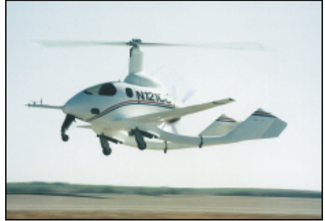
Figure 15-3. The CarterCopter uses wings to enhance performance.
