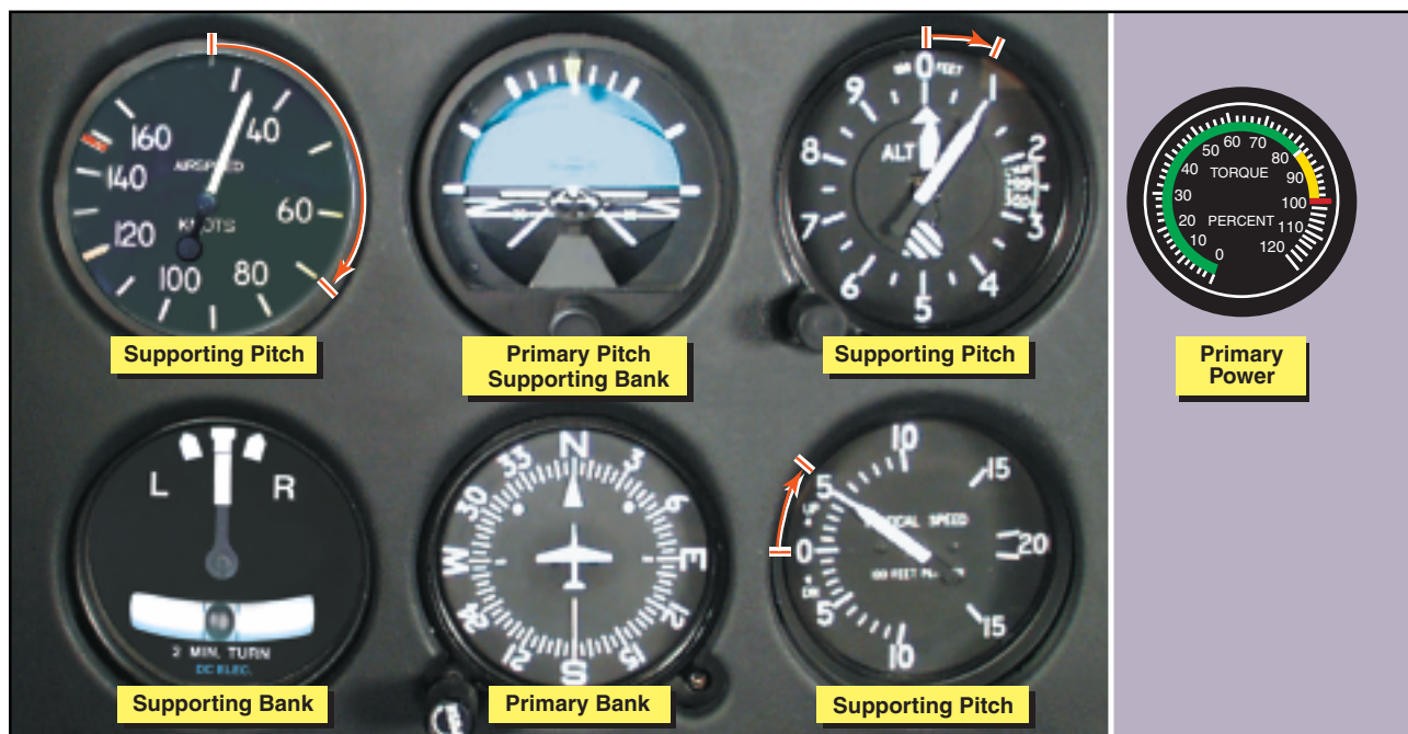
Figure 12-22. Flight instrument indications during an instrument takeoff.
