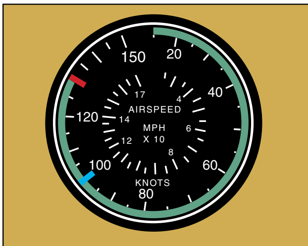
Figure 6-2. Typical airspeed indicator limitations and markings.
