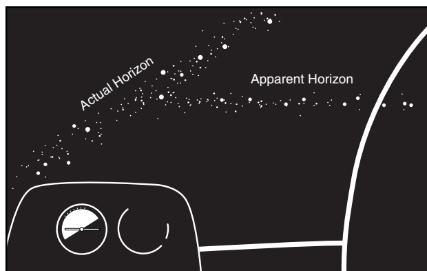
Figure 13-6. You can place your helicopter in an extremely dangerous flight attitude if you align the helicopter with the wrong lights. Here, the helicopter is aligned with a road and not the horizon.
