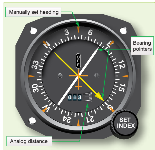
Figure 5-10. Bearing distance heading indicator.
