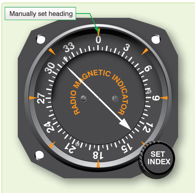
Figure 5-9. Radio magnetic indicator.
