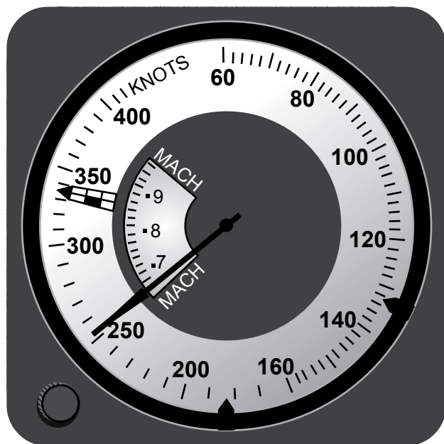
Figure 3-25. Combined airspeed Mach indicator.
