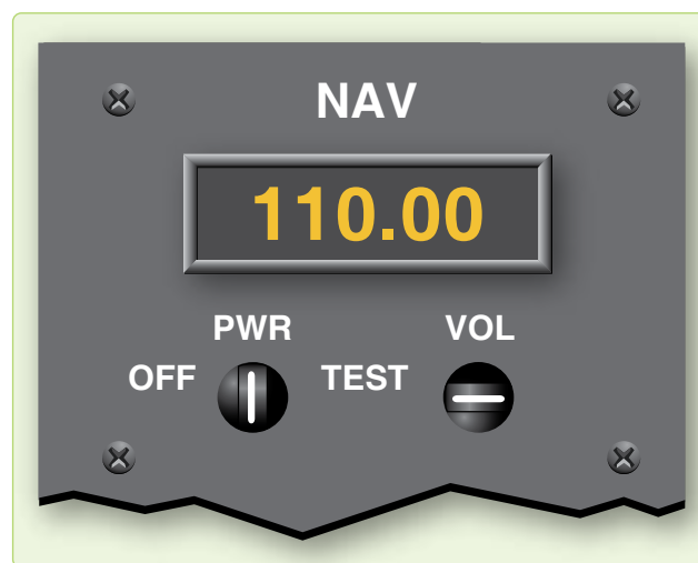
Figure 5-7. VOR navigation control panel.
