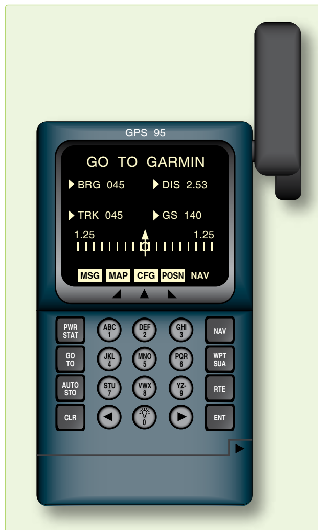
Figure 16-11. Handheld user equipment set.
