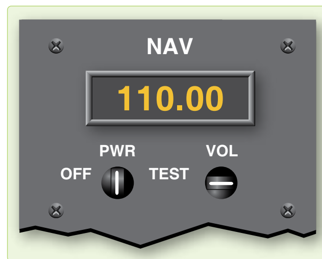
Figure 5-7. VOR navigation control panel.
