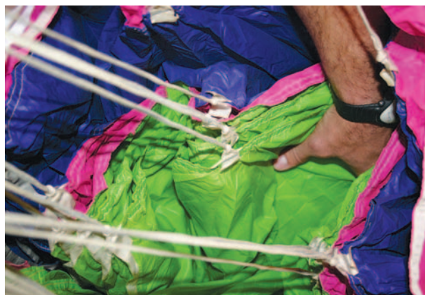
Figure 4-10. Separate and clear material between line groups.
