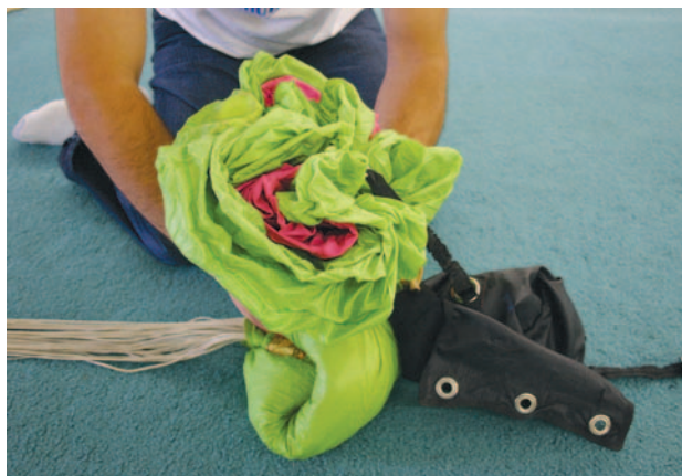
Figure 4-25. Fold the top of the canopy bundle back towards the lines for a second "S" fold.
