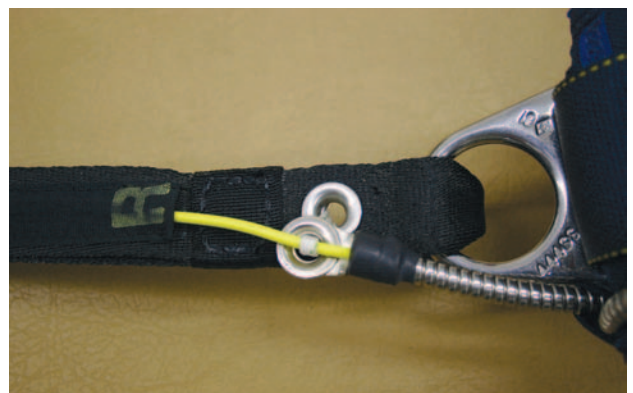
Figure 4-42. 3-ring cable thru loop.
