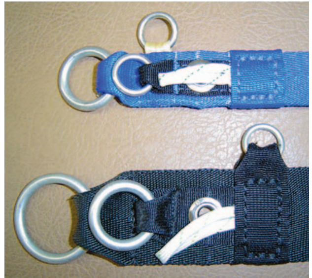
Figure 5-27. RSL/riser attachment.
