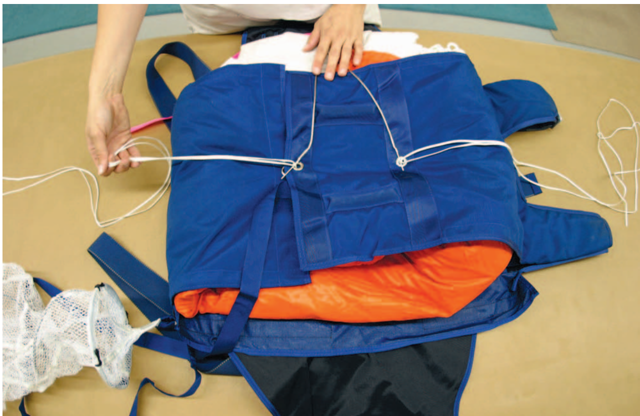
Figure 5-61. Upper temp pin seated.
