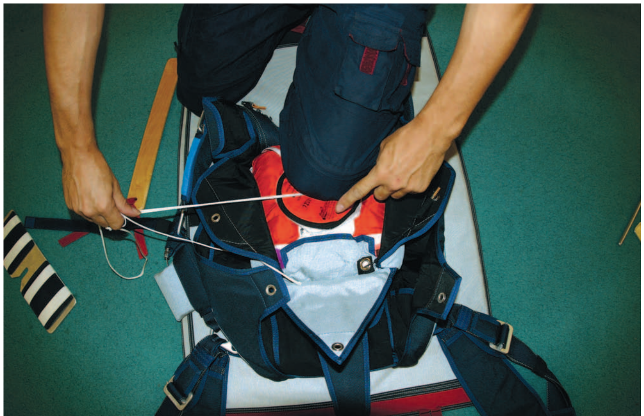
Figure 5-109. Position pilot chute.
