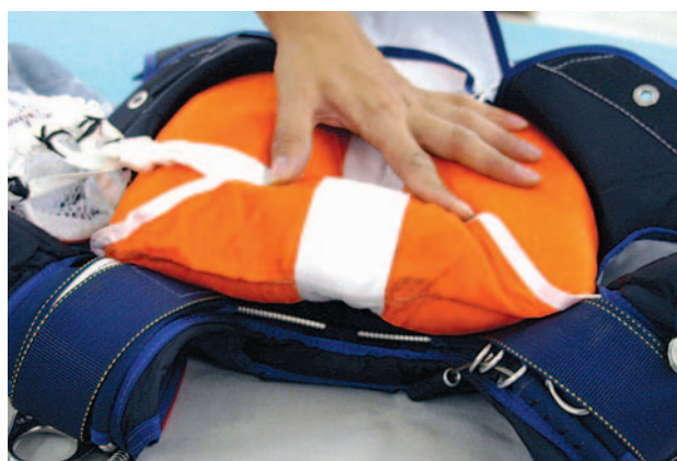
Figure 5-106. Fold the yoke over the bridle.
