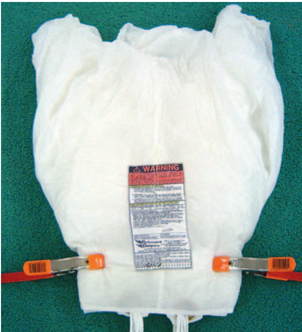
Figure 5-93. Wrap tail, two clamps.
