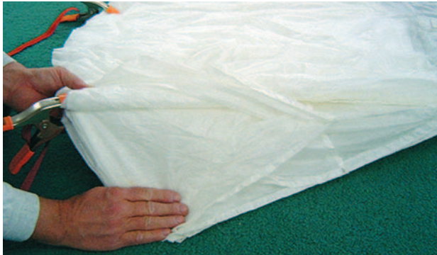
Figure 5-76. Fold half under "A" lines.
