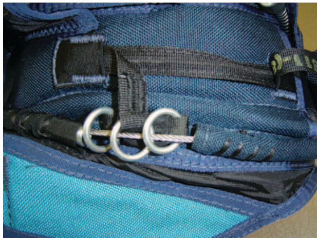
Figure 2-56. Ripcord cable routing thru rings.
