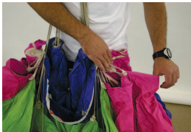
Figure 4-8. Clear the stabilizers on each side.
