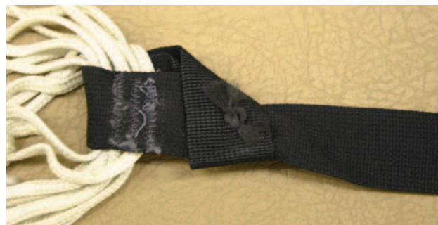
Figure 2-32. Hand tack floating bridle loop.
