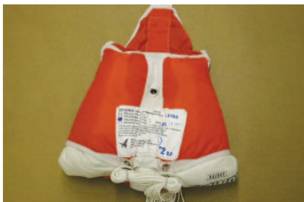
Figure 2-23. Type 5 deployment – Free Bag.
