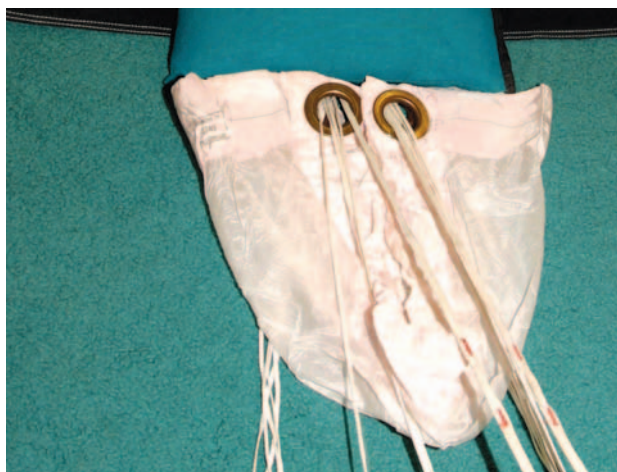
Figure 5-72. Pull slider down.
