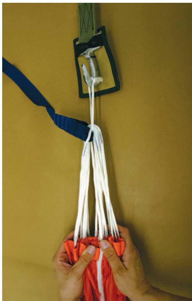
Figure 5-34. Straightening the canopy apex.
