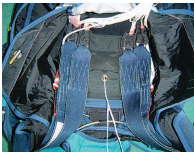
Figure 5-104. Place risers in the pack tray and spread.
