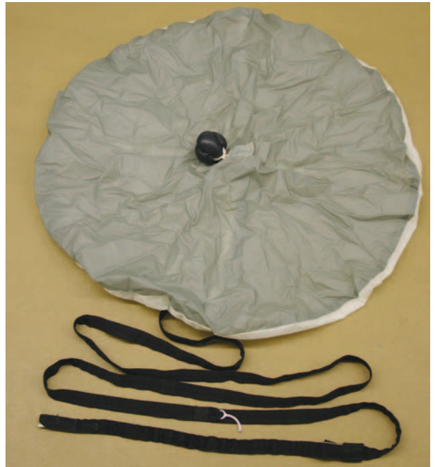
Figure 2-40. TOP bridle/pin configuration.
