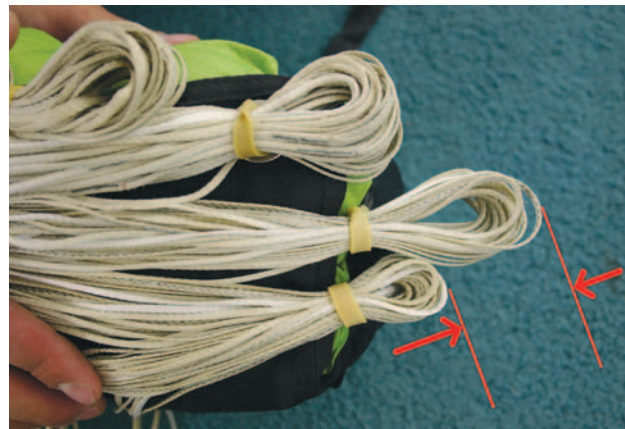
Figure 4-35. Line stow length comparison.
