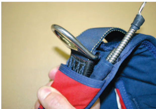
Figure 4-44. Harness 3-ring inspection.
