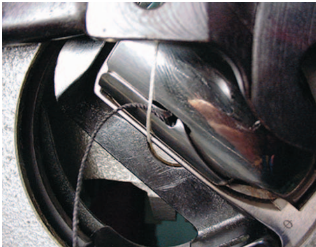
Figure 6-69. Fourth in sequence in forming a stitch.
