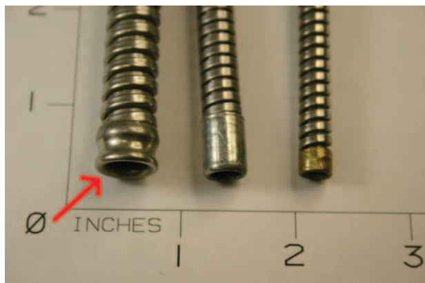
Figure 3-89A. Housing, flexible, ripcord.
