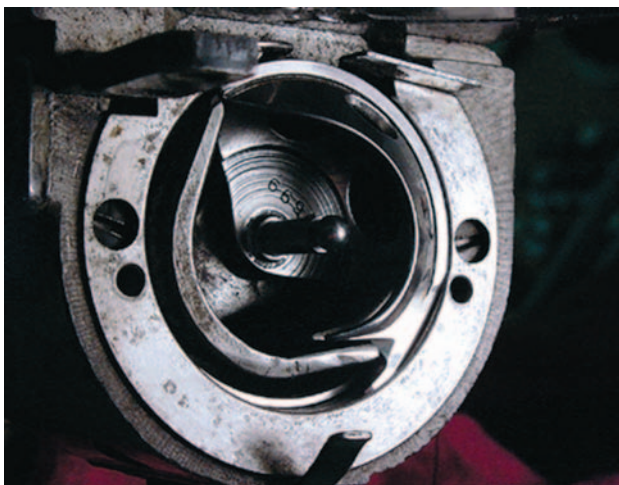
Figure 6-71. Oscillating hook.
