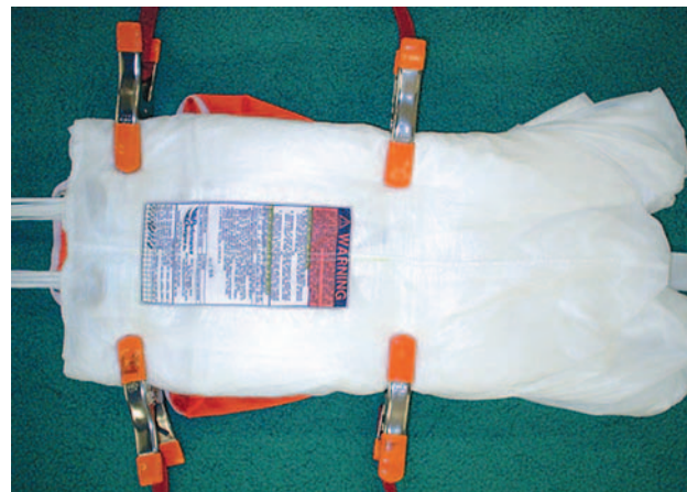
Figure 5-95. Bag positioned under canopy.
