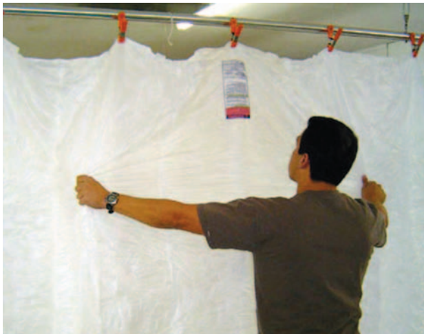
Figure 5-20. Ram-air canopy hanger—top skin inspection.
