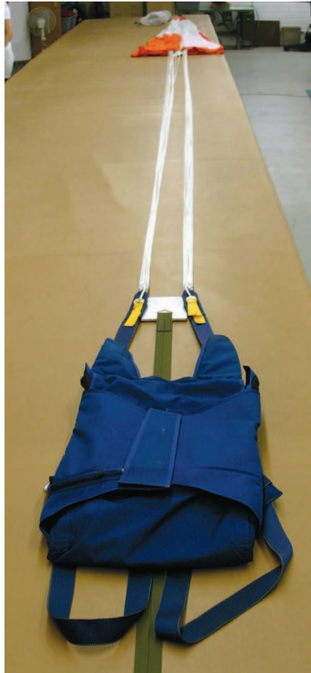
Figure 5-4. Round canopy pilot emergency parachute assembly.
