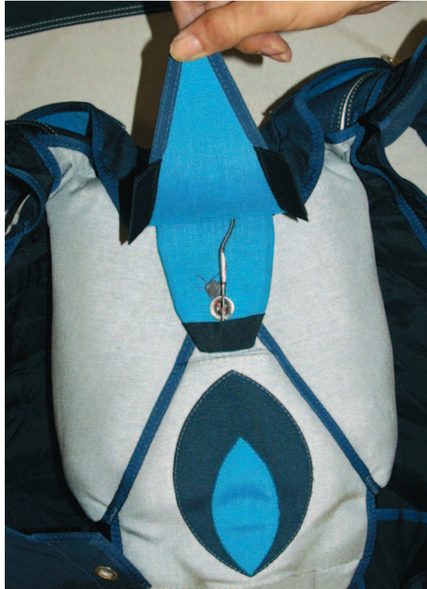
Figure 5-113. Close flap #4 and insert ripcord pin.
