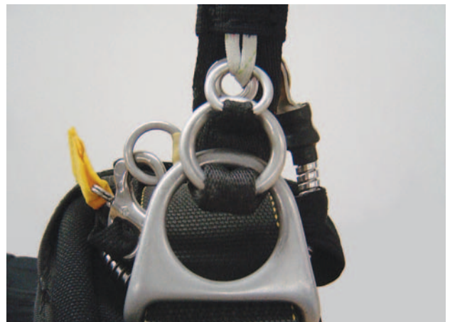
Figure 2-47. Single side RSL configuration.
