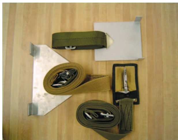
Figure 6-51. Tension board assembly with apex tiedown.
