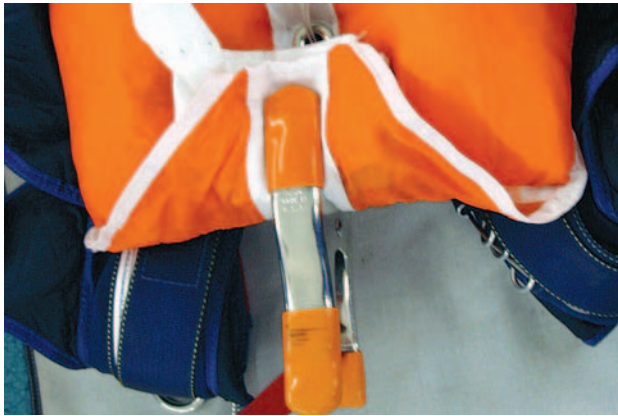
Figure 5-107. Secure yoke/bridle with clamp.
