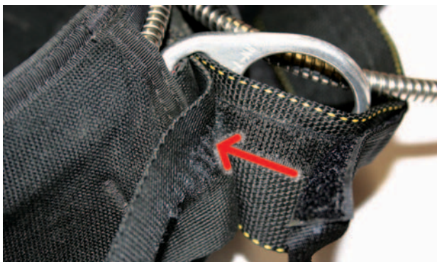
Figure 2-54. RSL Velcro® riser damage.
