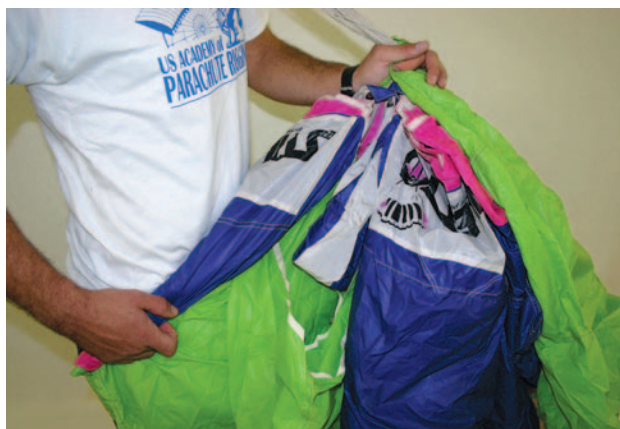
Figure 4-33. Rolling the nose of the canopy.
