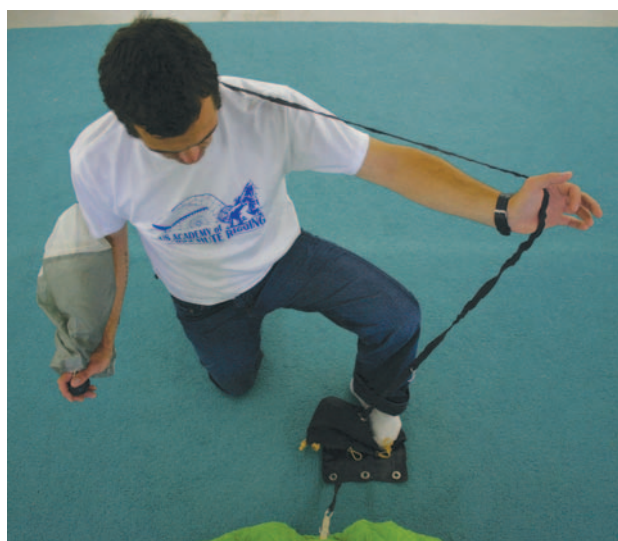
Figure 4-21. If used, cock the kill-line bridle.
