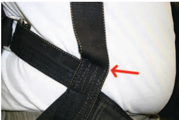
Figure 2-16. Standard harness junction warping.
