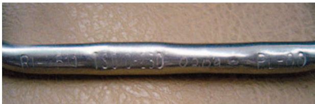
Figure 5-3. Reserve ripcord with TSO markings.
