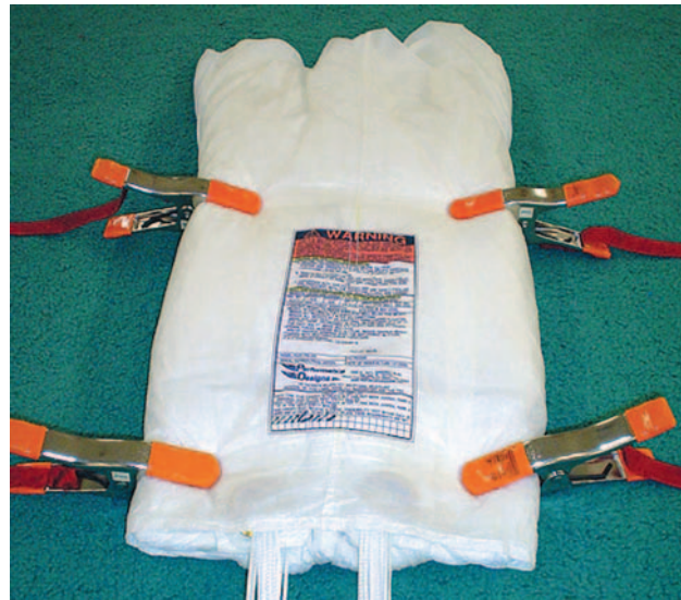
Figure 5-94. Finish wrapping tail, four clamps.
