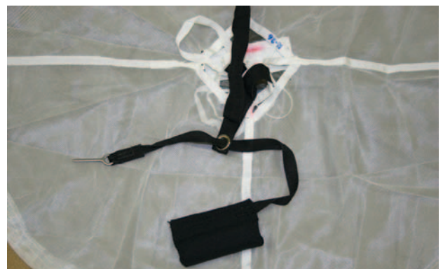
Figure 2-42. POP handle and lanyard.
