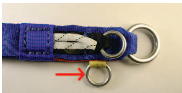
Figure 2-51. Main riser RSL ring attachment.
