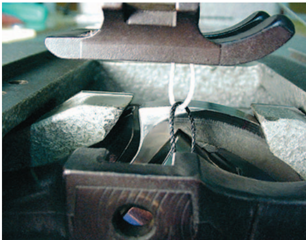
Figure 6-70. Fifth in sequence in forming a stitch.
