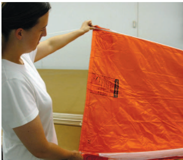
Figure 5-11. Round canopy gore inspection.
