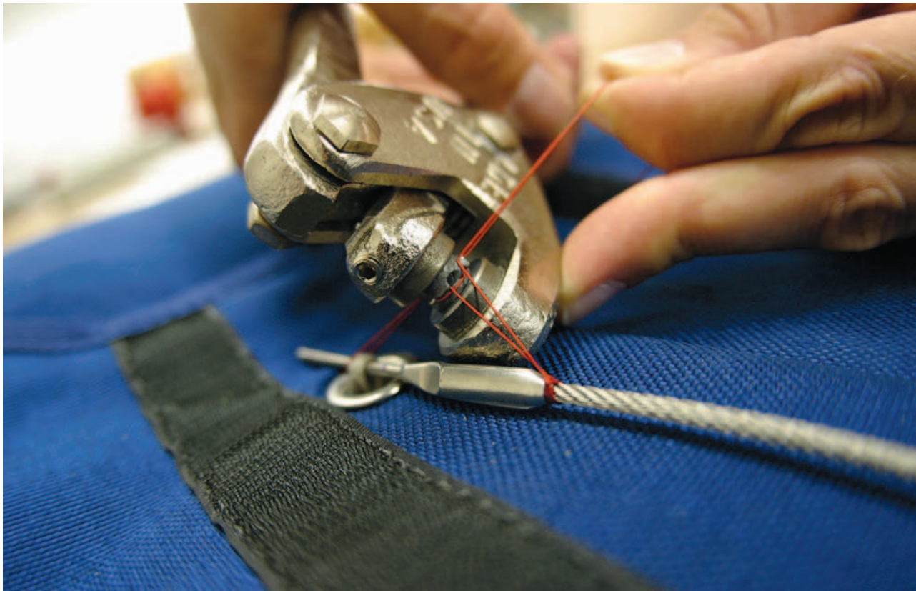
Figure 5-68. Compressing the seal.
