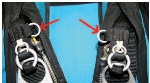
Figure 2-48. Dual side RSL configuration.
