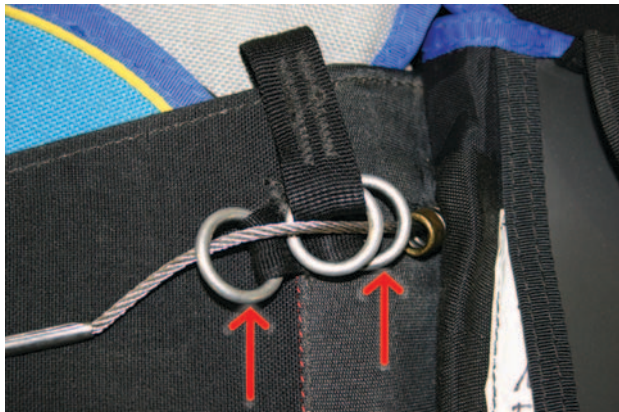
Figure 2-53. Double ring container installation.
