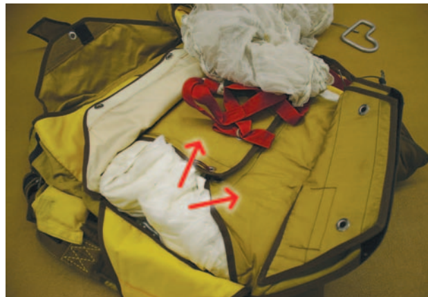
Figure 4-50. Type 1 deployment in a sport piggyback.
