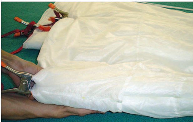
Figure 5-77. Smooth panels under "A" lines.
