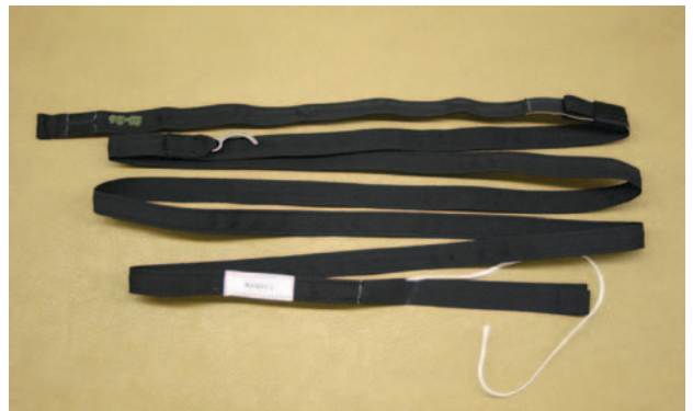
Figure 2-35. Kill-line collapsible bridle.
