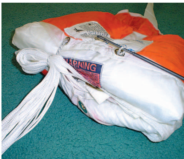
Figure 5-102. Close bag and secure locking stows.
