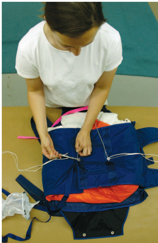
Figure 5-60. Closing bottom flap.
