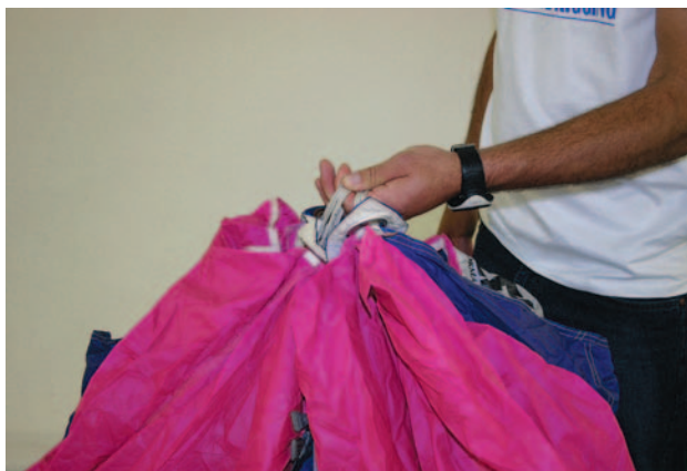
Figure 4-5. Transfer all the lines to one hand.
