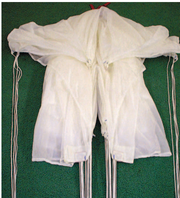
Figure 5-82. Split the trailing edge.
