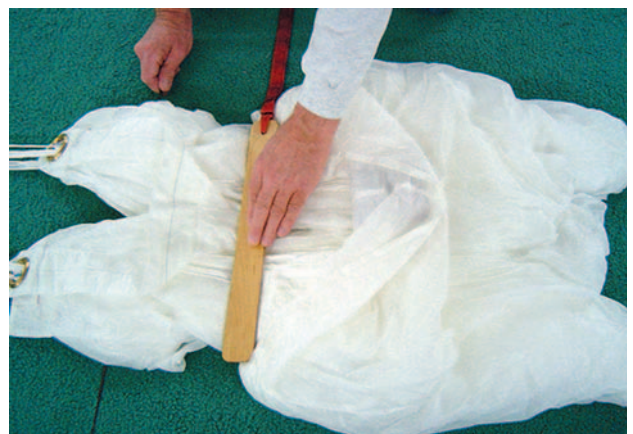
Figure 5-91. Packing paddle at 1/3rd location.
