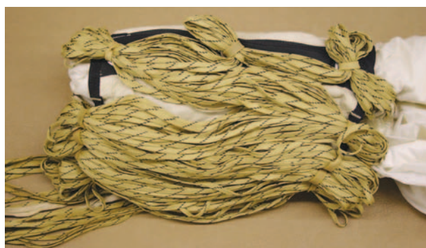
Figure 2-22. Type 4 deployment – Preserve diaper.
