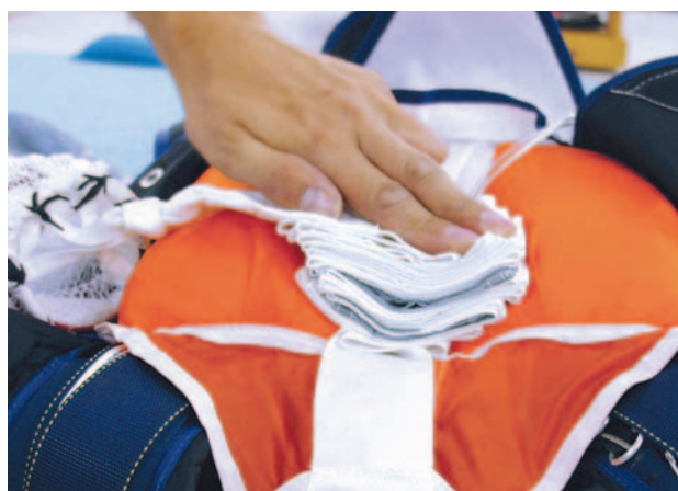
Figure 5-105. "S" fold the bridle on bag.
