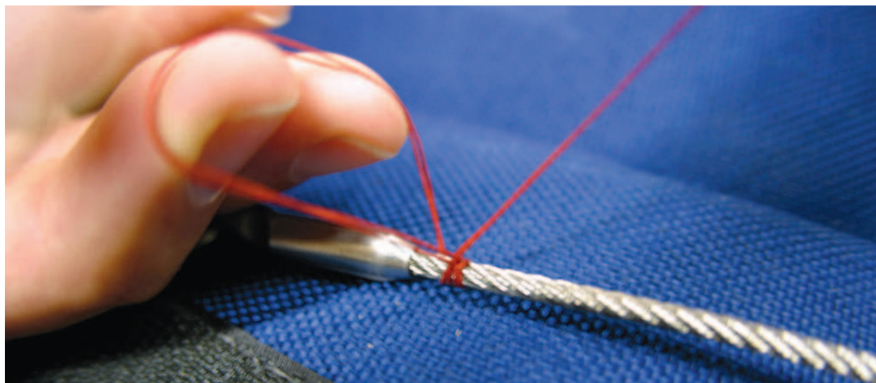
Figure 5-65. Lark’s head the thread on the cable.
