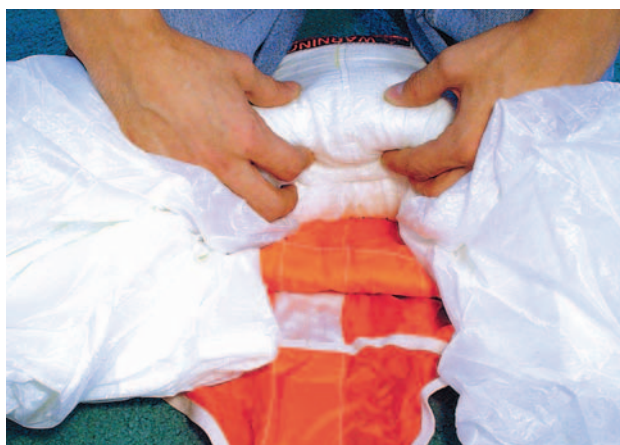
Figure 5-98. Gather and roll center seam fabric.
