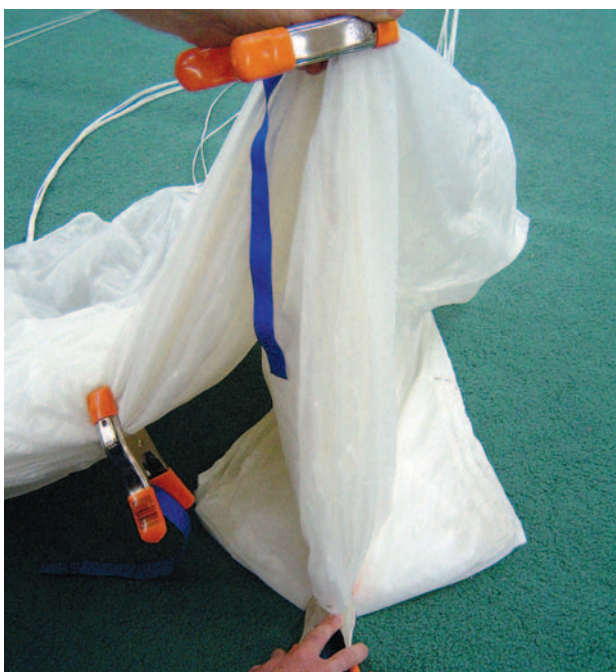
Figure 5-78. Hold "B" clamp vertically over "A" clamp.
