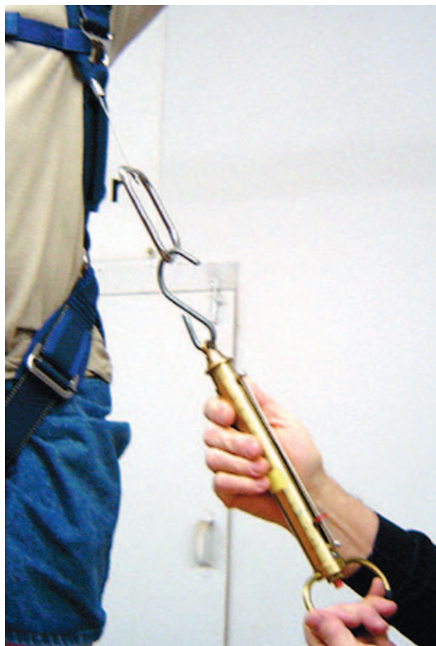
Figure 5-64. Ripcord pull test.
