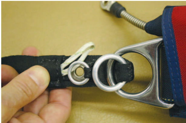
Figure 4-37. 3-ring middle thru large ring.
