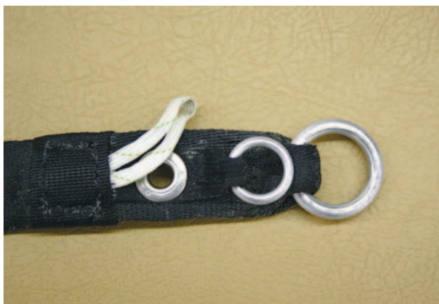
Figure 4-45. Riser release end.
