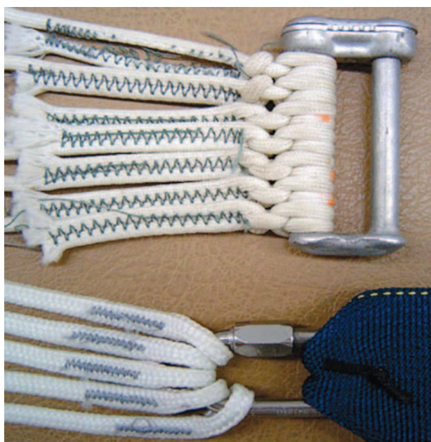
Figure 5-13. Connector link line attachment methods.
