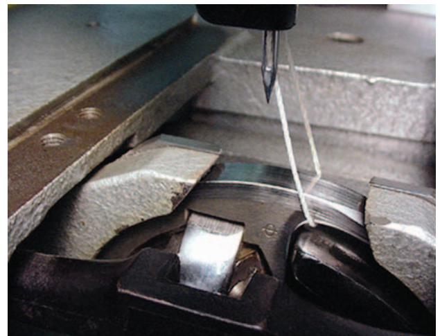
Figure 6-68. Third in sequence in forming a stitch.
