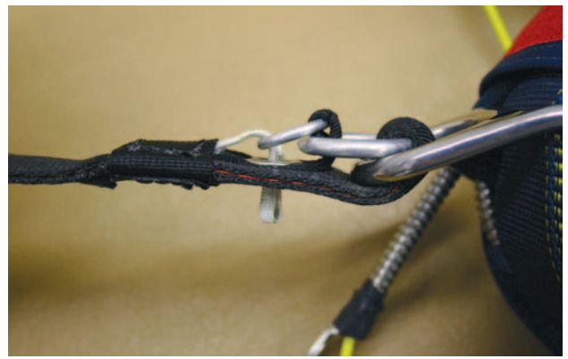
Figure 4-40. 3-ring loop from rear.
