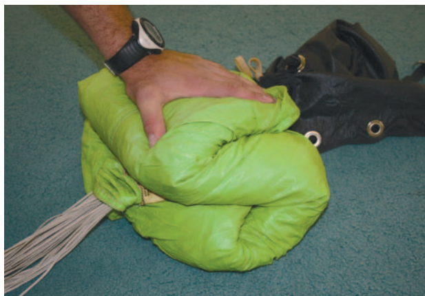
Figure 4-26. Complete the "S" fold.
