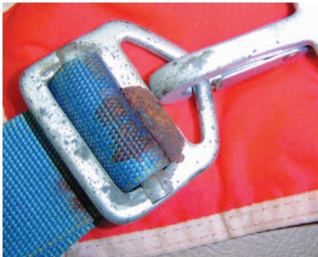
Figure 5-17. Rusty leg snap hardware.
