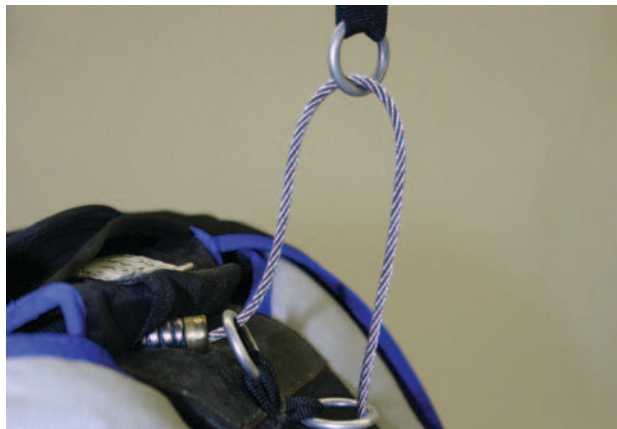
Figure 2-57. RSL lanyard extension.
