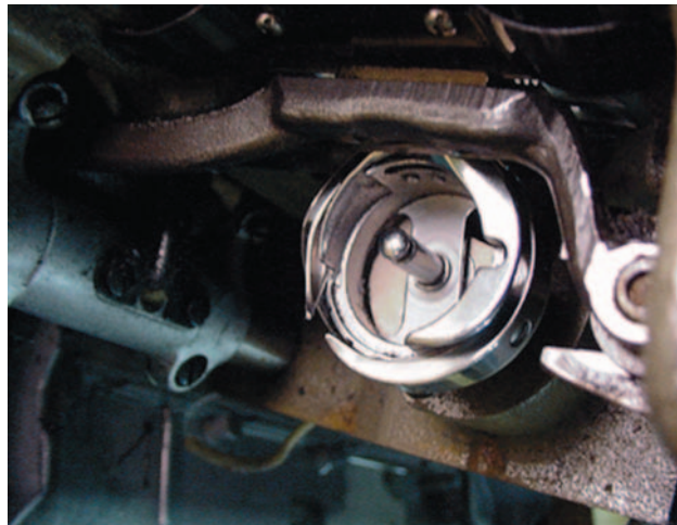
Figure 6-72. Rotary hook.
