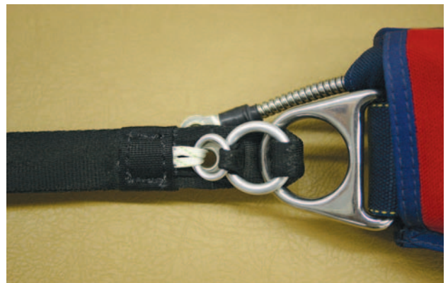
Figure 4-43. 3-ring finished from front.
