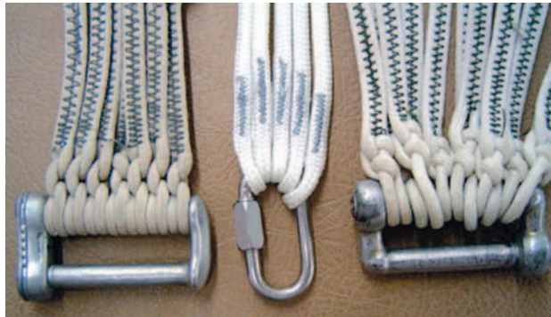
Figure 5-14. Three types of connector links.
