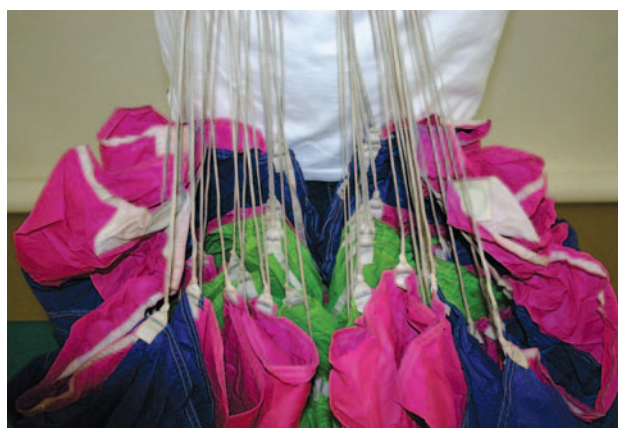
Figure 4-9. View from front with slider moved upward for clarity. Note how the attachment tapes of each line group fall together.
