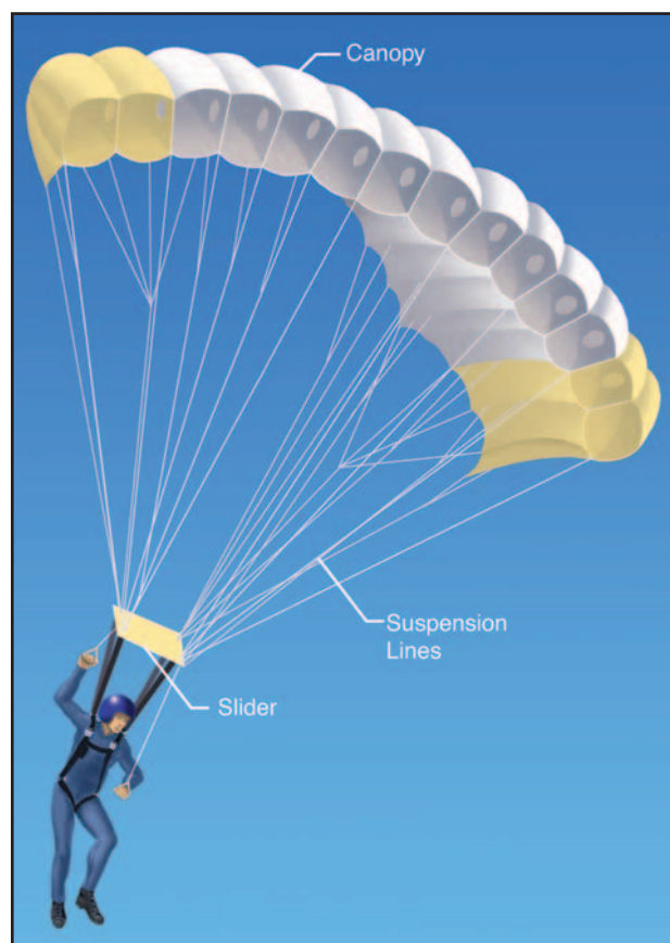
Figure 2-1. Component parts of a main parachute assembly.
