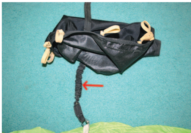
Figure 4-22. Check the collapsed bridle.
