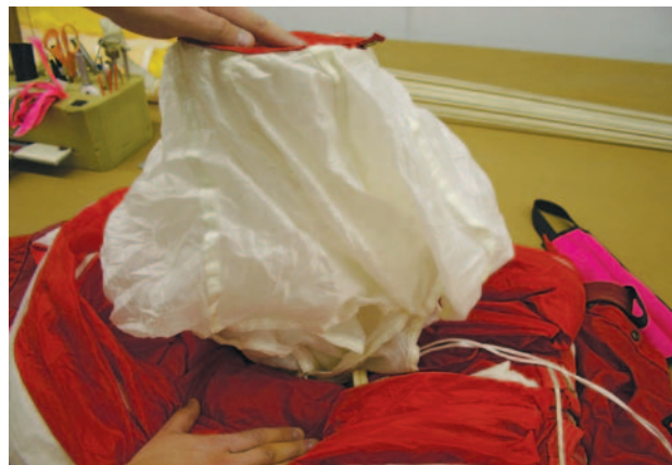
Figure 4-49. Type 1 deployment in a pilot emergency rig.
