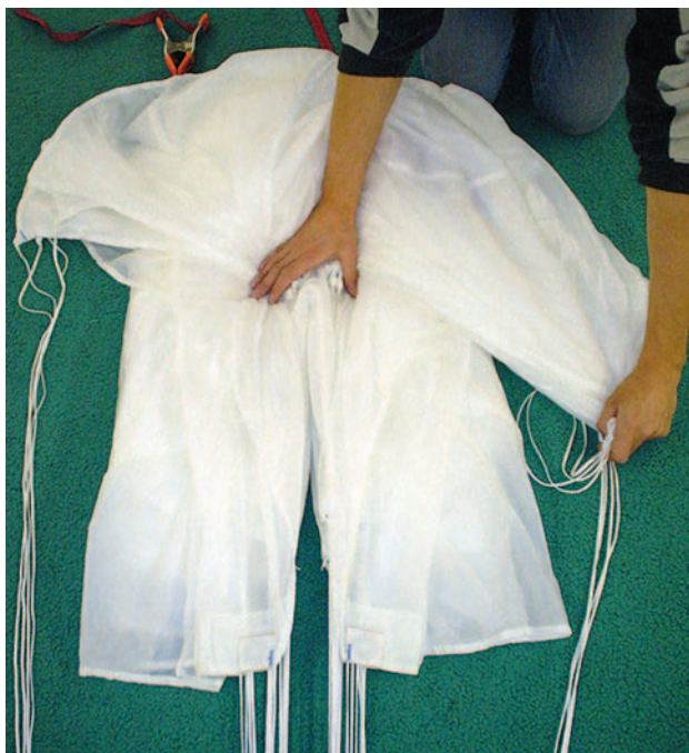
Figure 5-83. Pull down the trailing edge.
