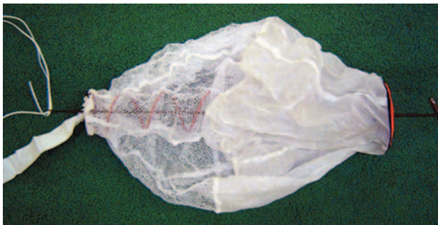
Figure 5-108. Gun rod through the pilot chute.
