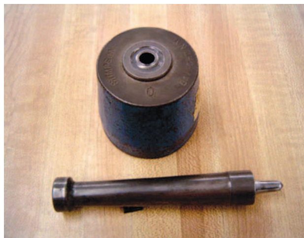
Figure 6-52. Size “O” rolled rim spur grommet handset.
