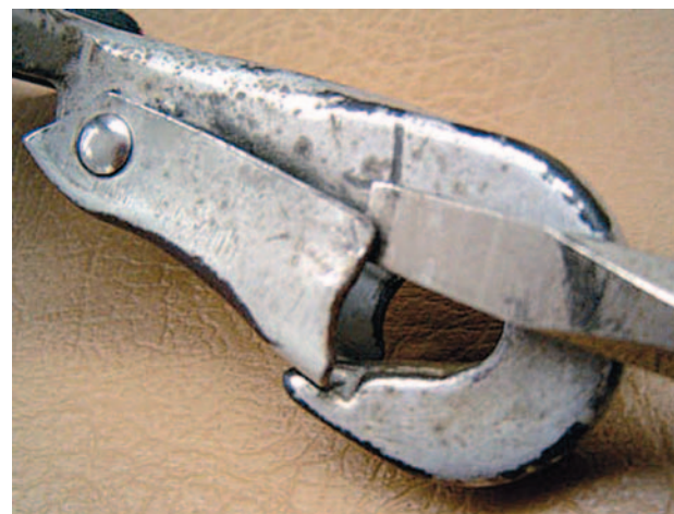
Figure 5-16. B-12 snap gate repair.
