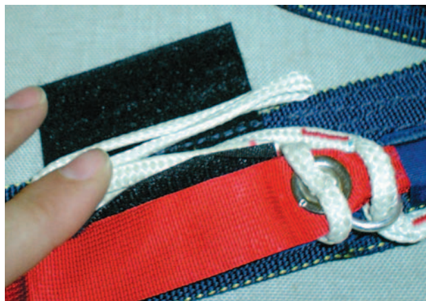
Figure 5-84. Set the deployment brakes.
