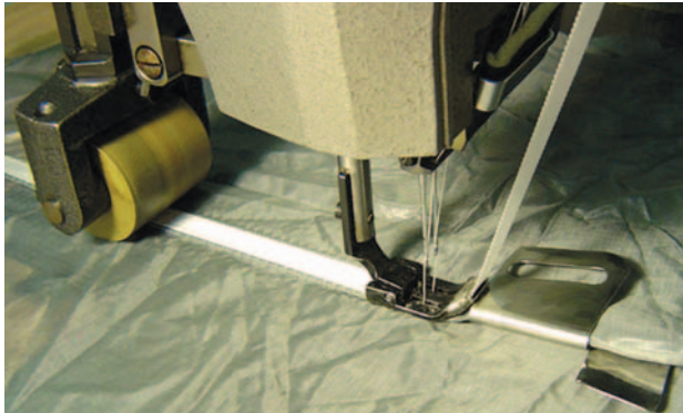
Figure 6-82. Tape feeder and French seam folder.
