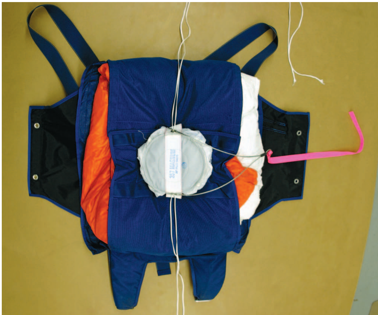
Figure 5-62. Pilot chute seated in position.
