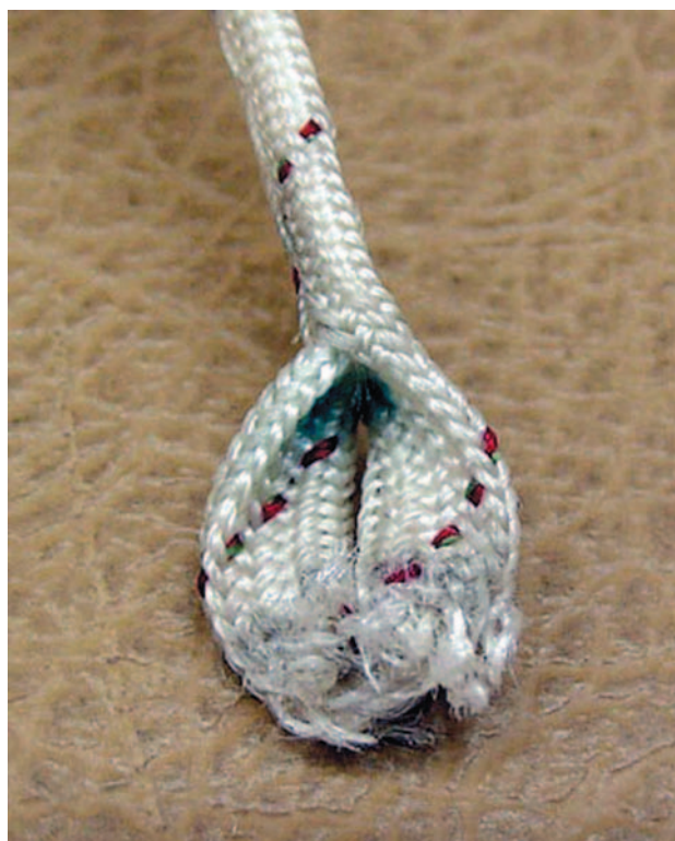
Figure 5-18. Worn closing loop.
