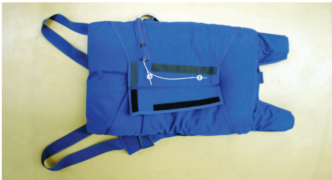
Figure 5-63. Ripcord pins in place.
