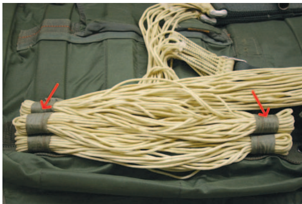
Figure 2-26. Hesitator loops.
