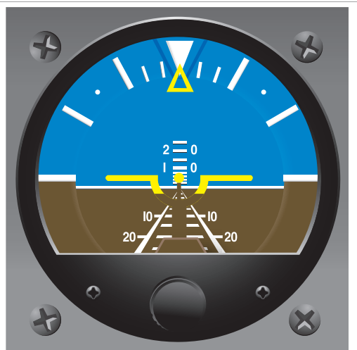
Figure 7-5. Pitch correction for level flight, one bar width.
