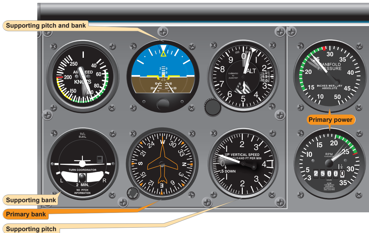
Figure 7-25. Climb entry for constant airspeed climb.
