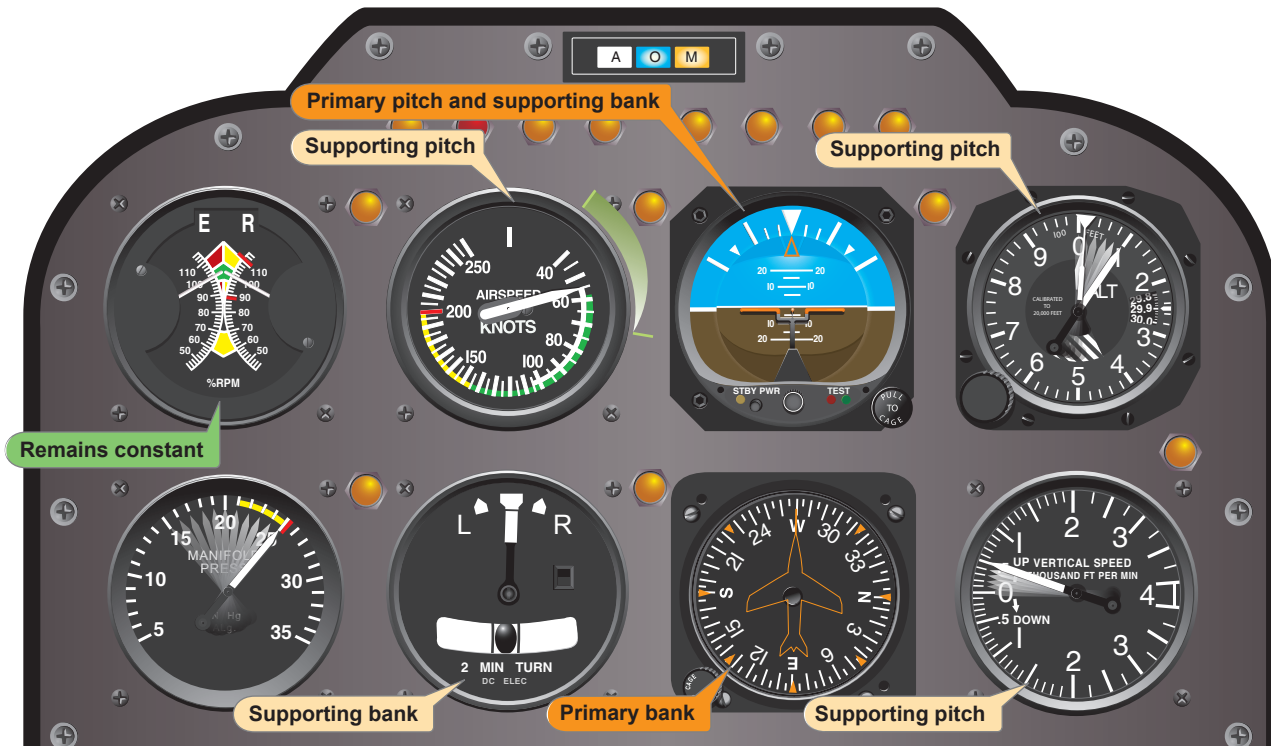
Figure 8-16. Flight instrument indications during an instrument takeoff.
