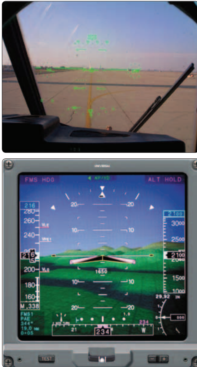
Figure 9-43. Example of a head-up display (top) and a head-down display (bottom). The head-up display presents information in front of the pilot along his/her normal field of view while a head-down display may present information beyond the normal head-up field of view.
