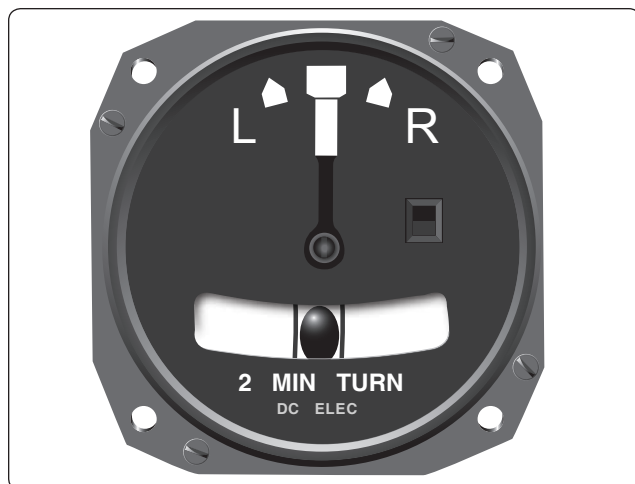
Figure 5-33. Turn-and-slip indicator.
