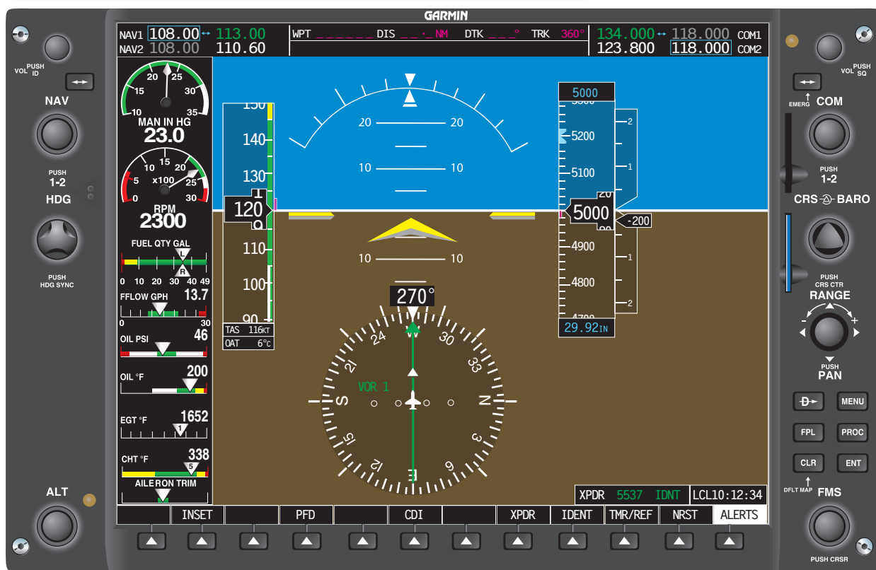
Figure 7-66. The top image illustrates a reduction of power and descending at 500 fpm to an altitude of 5,000 feet. The bottom image illustrates an increase in power and the initiation of leveling off.
