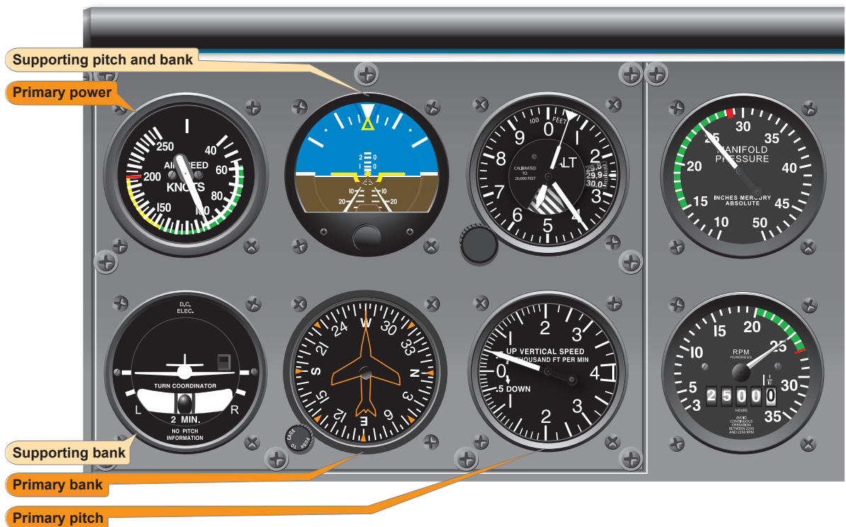
Figure 7-27. Stabilized climb at constant rate.
