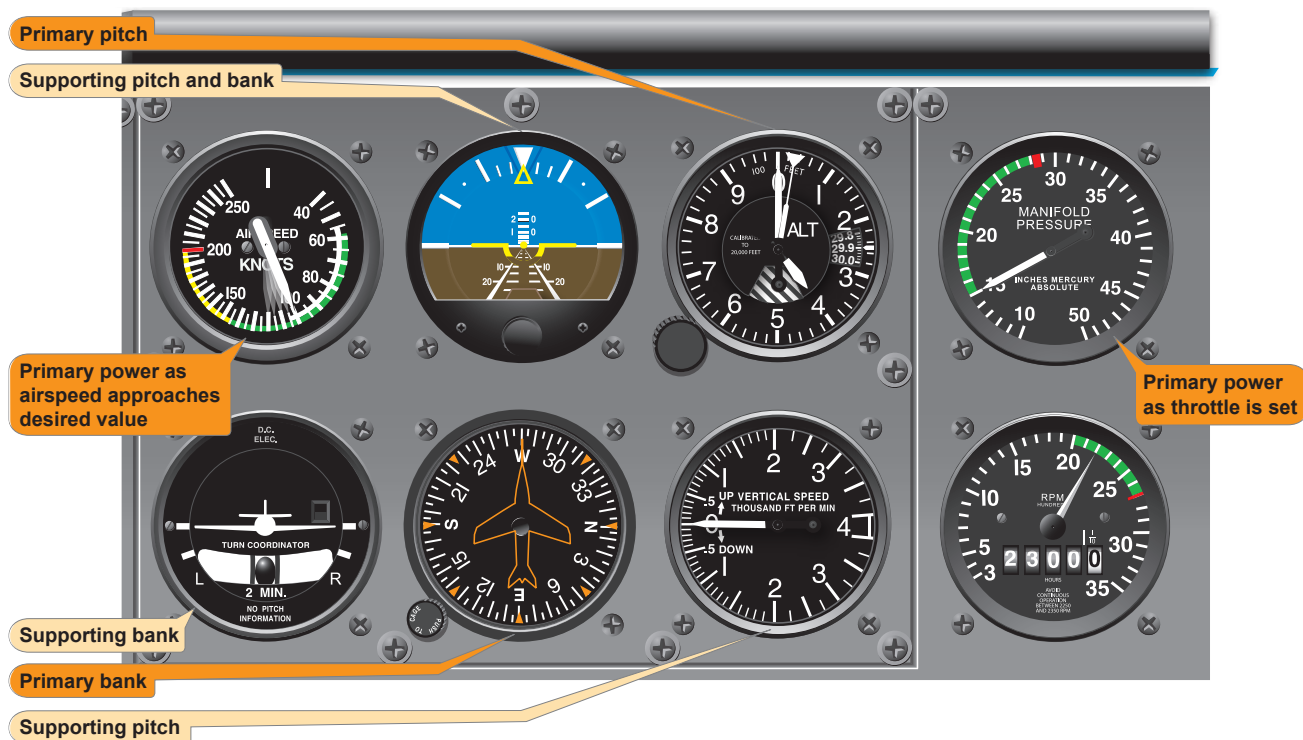
Figure 7-23. Straight-and-level flight (airspeed decreasing).
