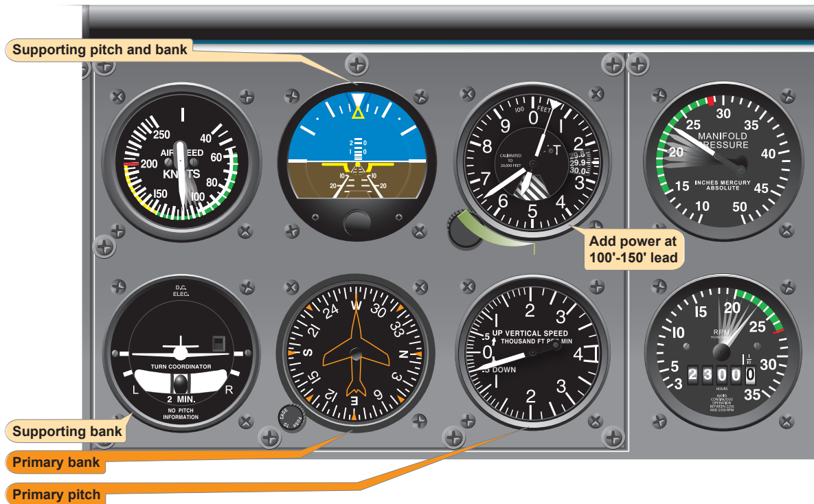
Figure 7-31. Level off airspeed higher than descent airspeed.
