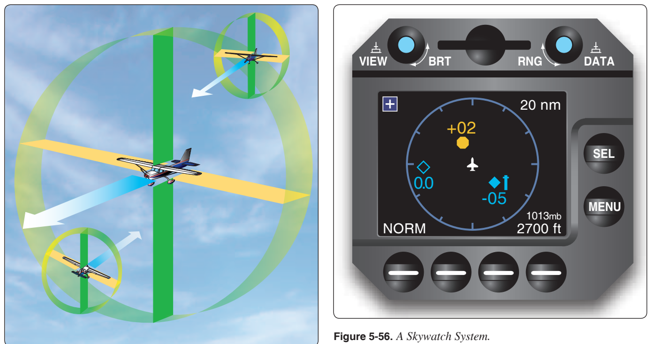
Figure 5-55. Theory of a typical alert system.
