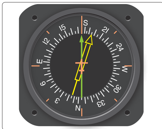
Figure 5-26. Driven by signals from a flux valve, the compass card in this RMI indicates the heading of the aircraft opposite the upper center index mark. The green pointer is driven by the ADF. The yellow pointer is driven by the VOR receiver.
