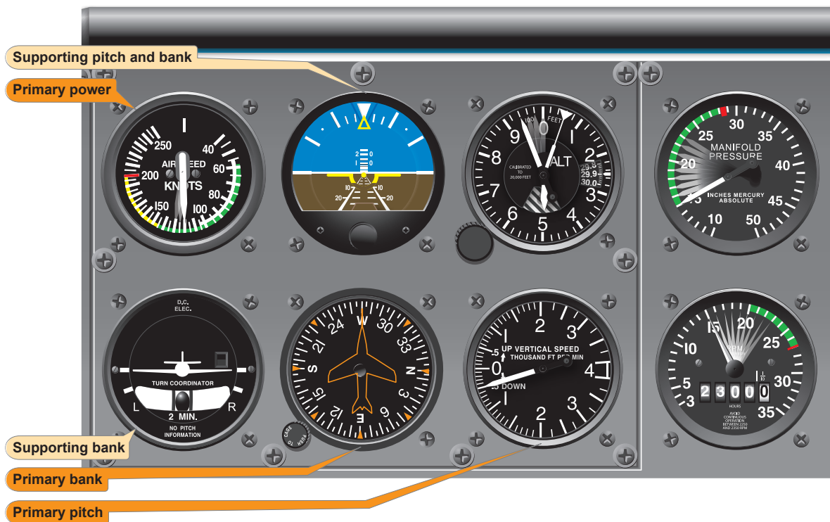
Figure 7-30. Constant airspeed descent, airspeed high—reduce power.
