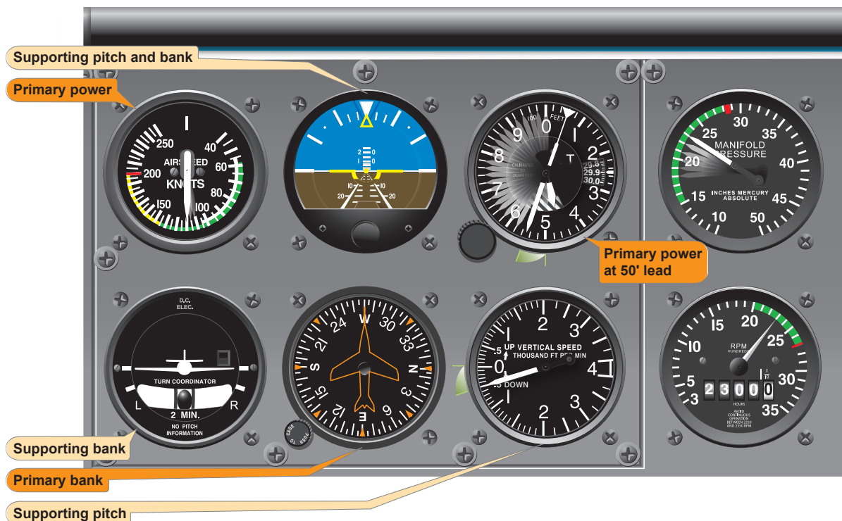
Figure 7-32. Level off at descent airspeed.
