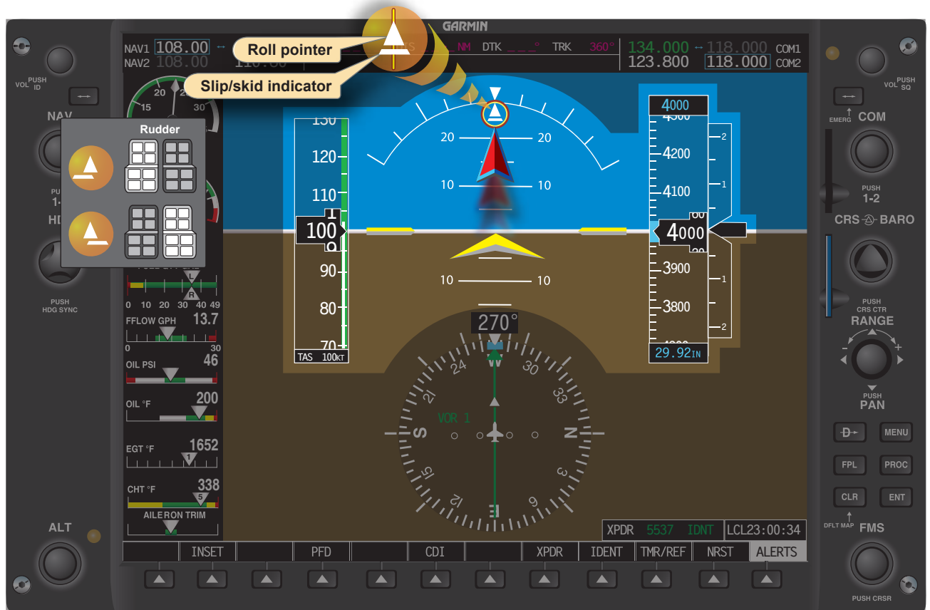
Figure 6-34. Roll pointer and slip/skid indicator.
