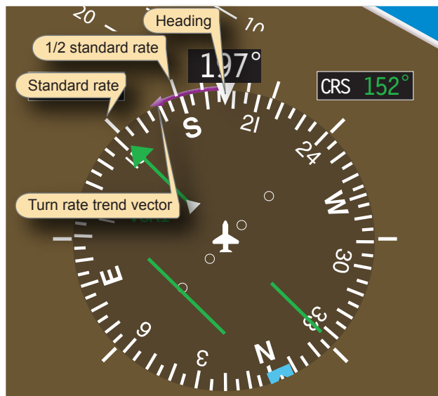
Figure 6-39. HSI indicator (enlargement).
