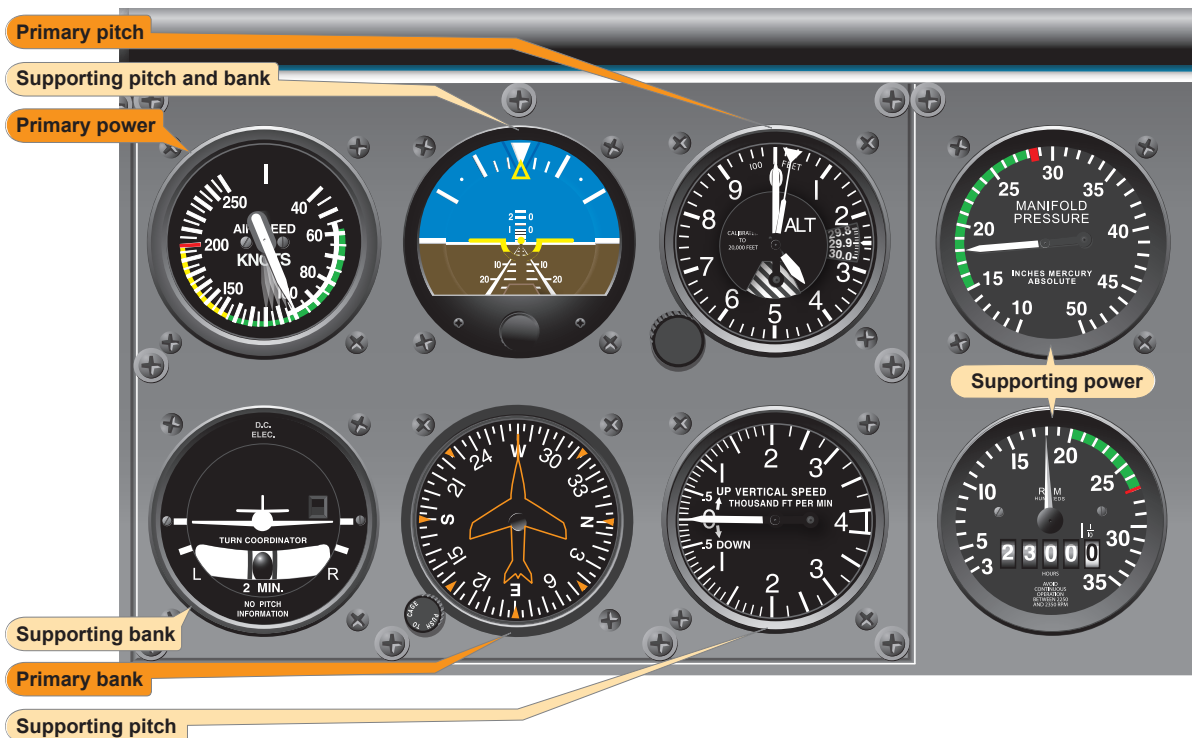
Figure 7-24. Straight-and-level flight (reduced airspeed stabilized).
