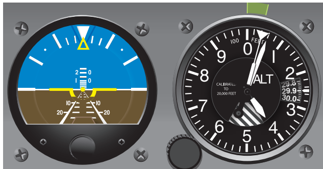
Figure 7-9. Altitude error, less than 100 feet.
