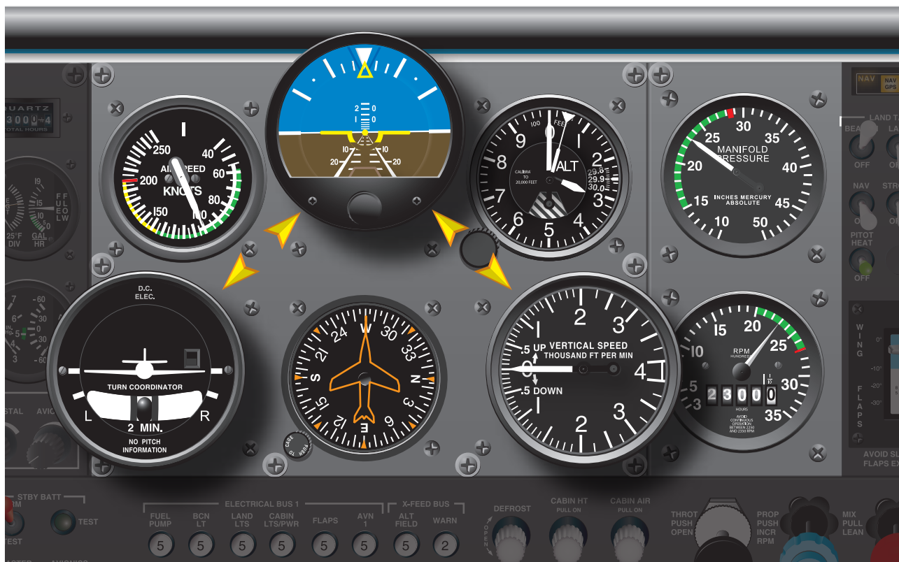
Figure 6-18. Inverted-V cross-check.
