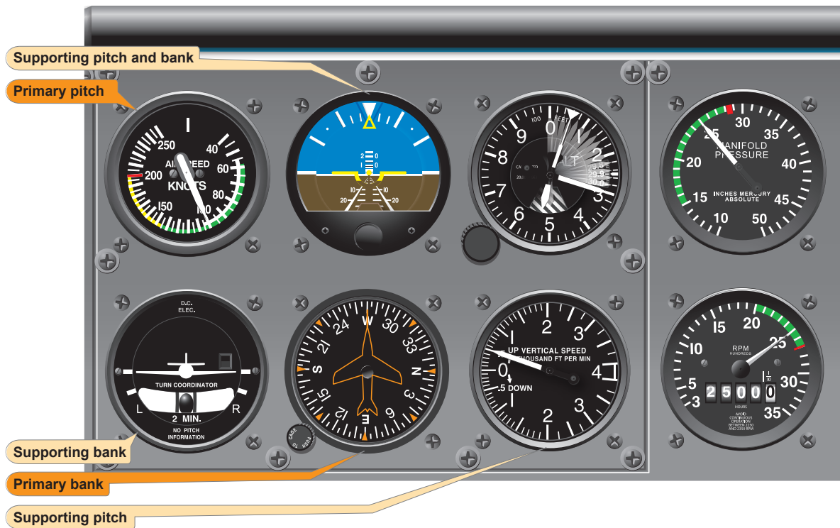
Figure 7-26. Stabilized climb at constant airspeed.
