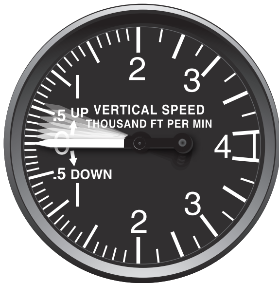
Figure 6-8. Vertical speed indicator.
