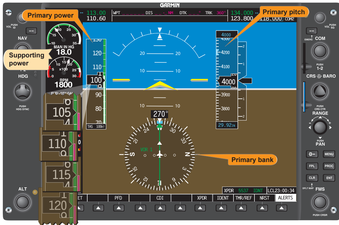
Figure 7-59. Straight-and-level flight (reduced airspeed stabilized).
