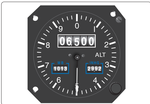
Figure 5-5. Drum-type altimeter.
