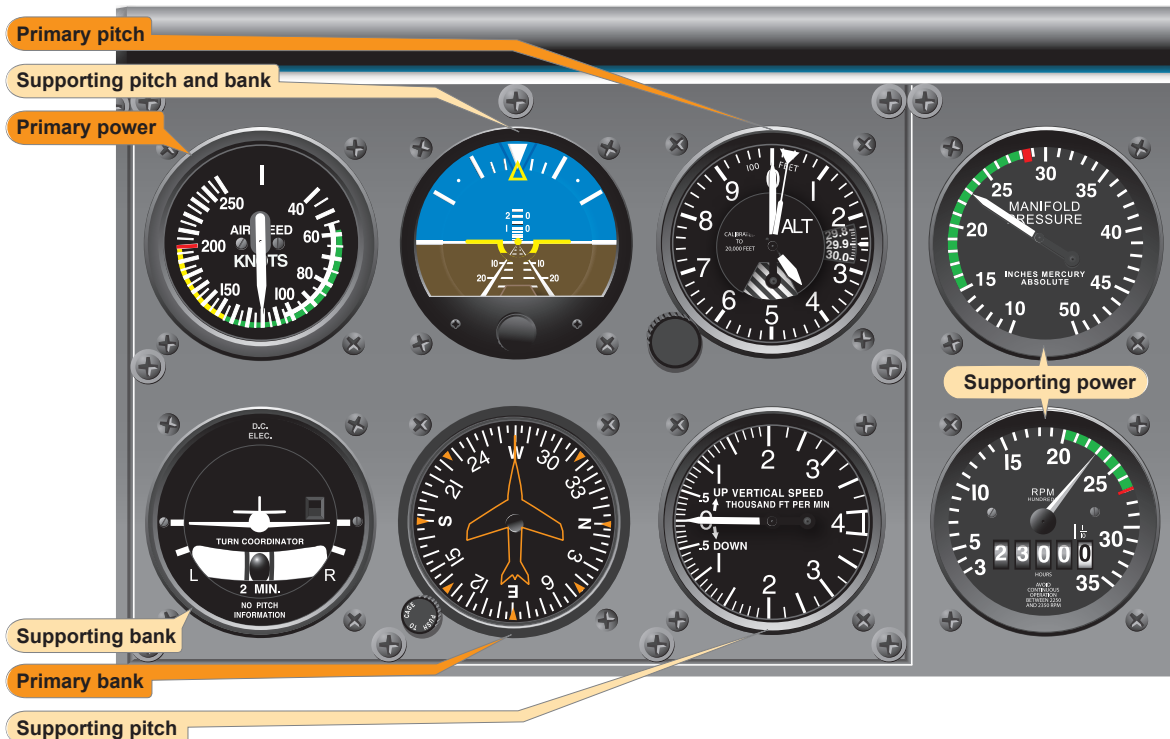
Figure 7-22. Straight-and-level flight (normal cruising speed).
