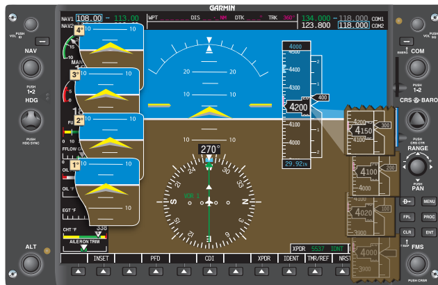
Figure 7-50. Pitch indications for various attitudes (1° through 5°).
