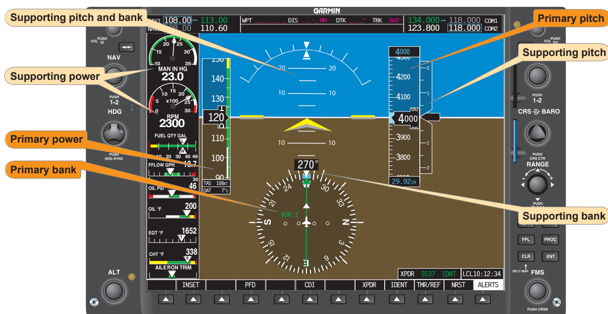
Figure 7-57. Straight-and-level flight (normal cruising speed).
