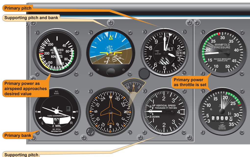
Figure 7-38. Change of airspeed during turn.
