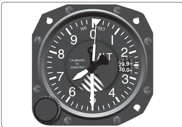
Figure 5-4. Three-pointer altimeter.
