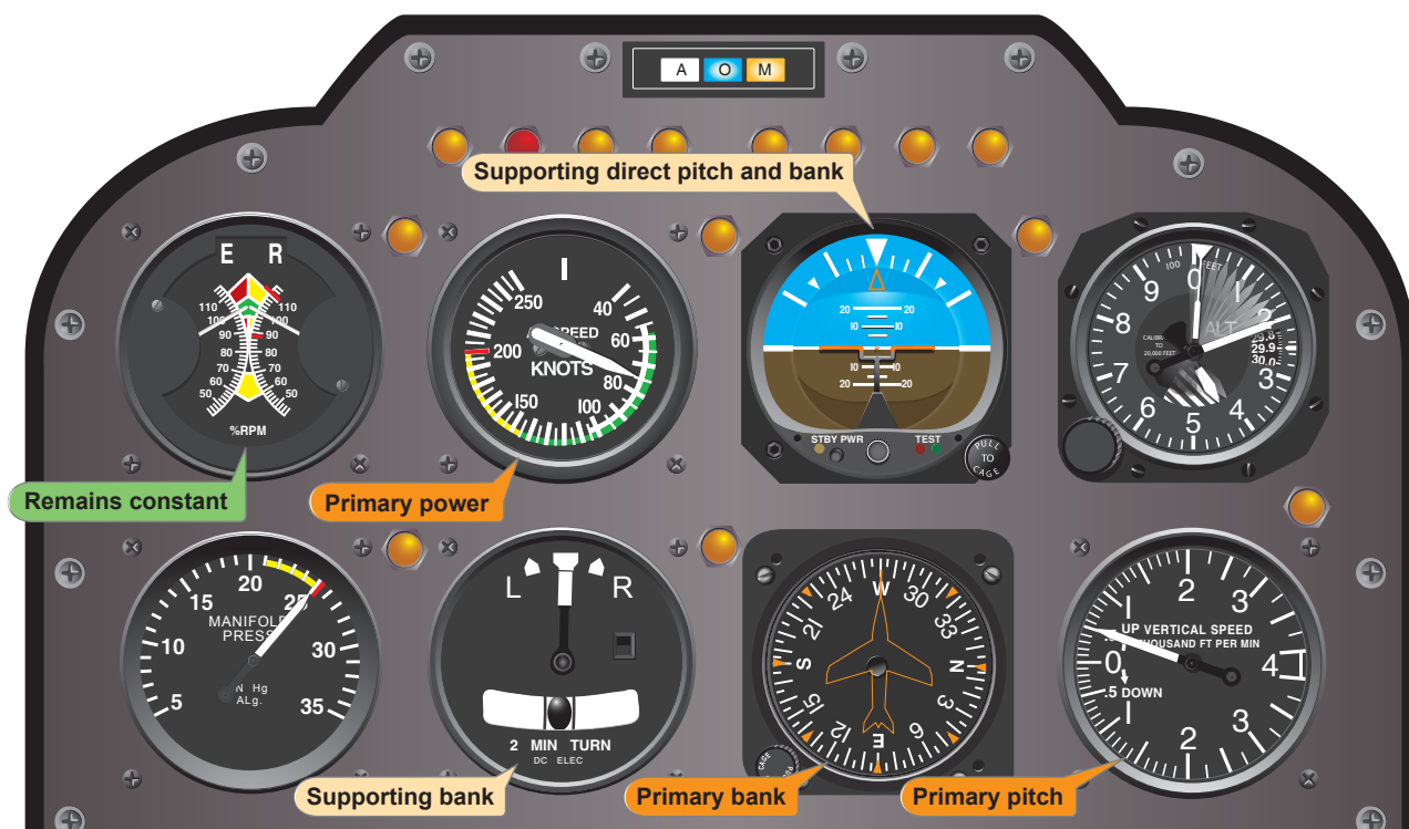
Figure 8-13. Flight instrument indications in a stabilized constant-rate climb.
