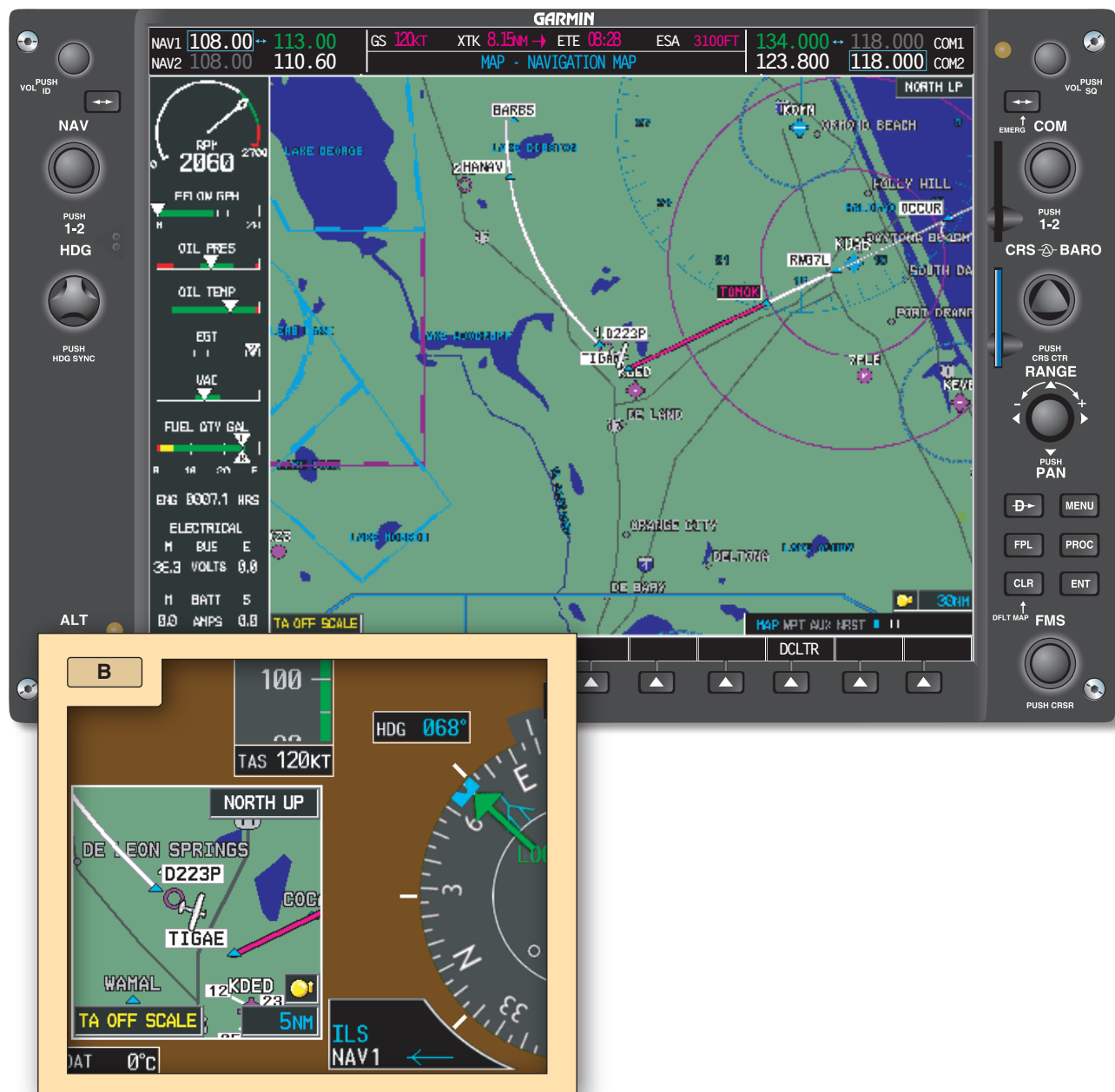
Figure 9-20. The same aircraft illustrated in Figure 9-19 shown on the ORM radial near TIGAE intersection turning inbound for the localizer.
