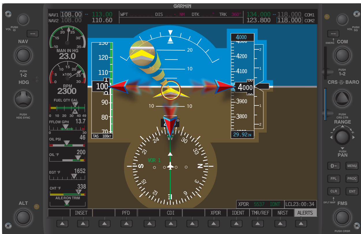
Figure 7-60. Cross-check supporting instruments.
