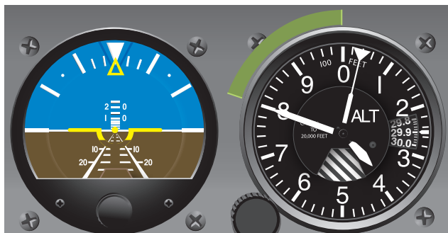
Figure 7-11. Altitude error, greater than 100 feet.
