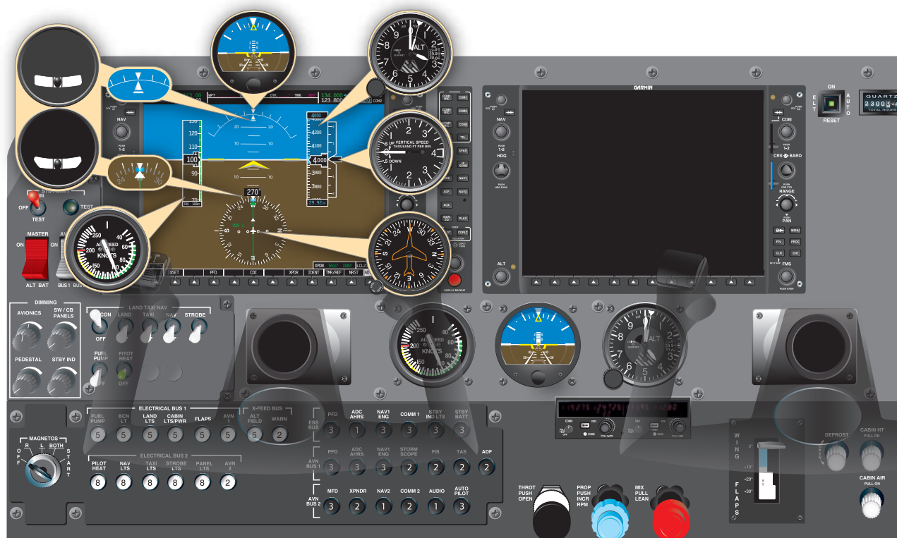
Figure 6-21. Primary flight display (PFD) and analog counterparts.
