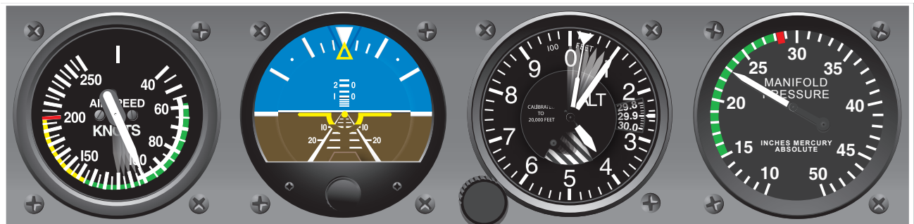
Figure 7-20. Airspeed low and altitude high—lower pitch.
