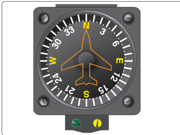
Figure 5-22. Vertical card magnetic compass.
