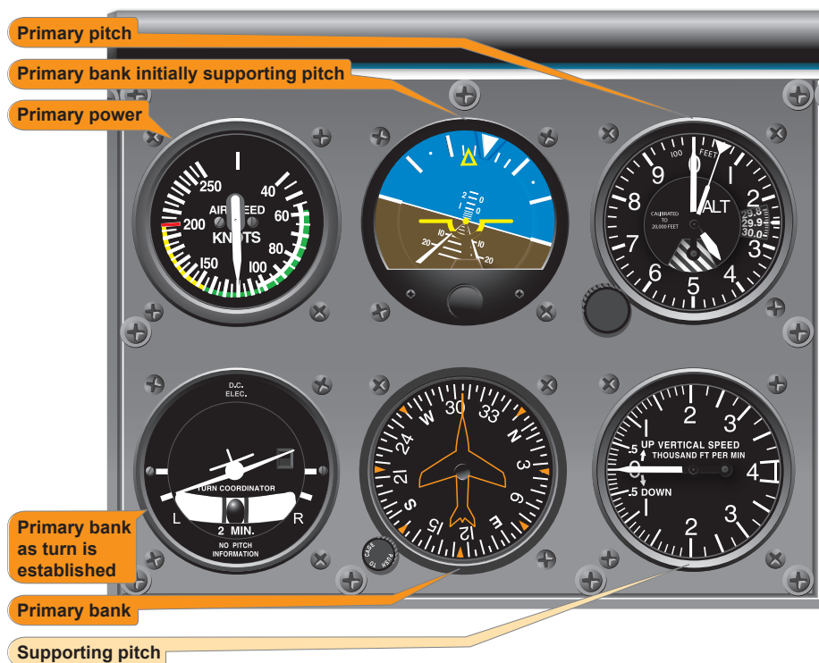
Figure 7-33. Standard rate turn, constant airspeed.
