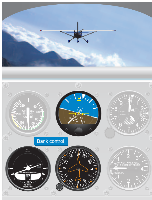
Figure 7-16. Instruments used for bank control.
