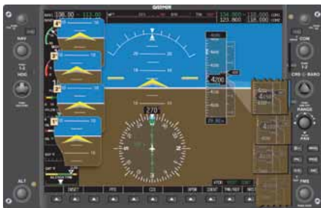
Figure 5-50. Pitch Indications for Various Attitudes ( 1^\circ through 5^\circ ).
