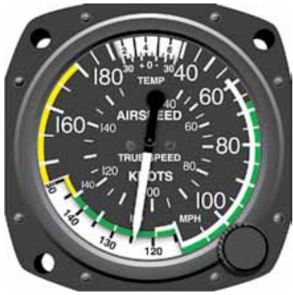
Figure 3-12. A true airspeed indicator allows the pilot to correct IAS for nonstandard temperature and pressure.
