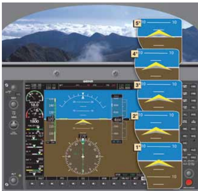
Figure 5-49. Various Pitch Attitudes (Right), Aircraft Shown in Level Flight.
