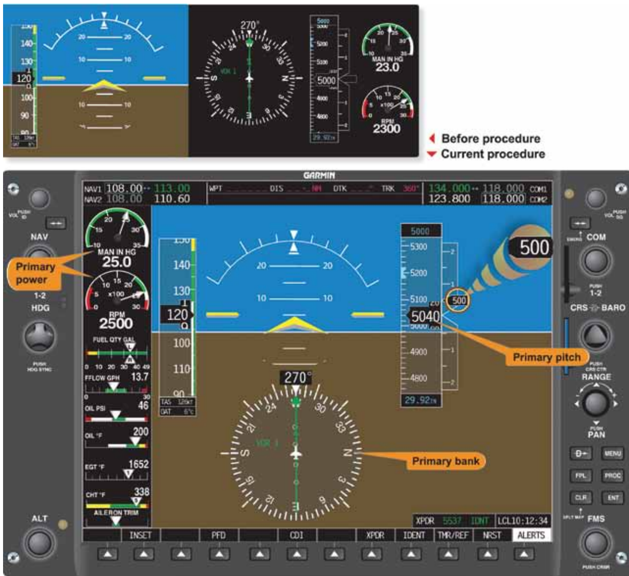
Figure 5-63. Constant Airspeed Climb From Cruise Airspeed.
