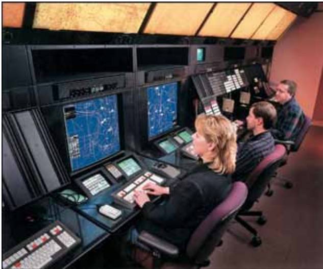
Figure 9-11. Center Radar Displays.
