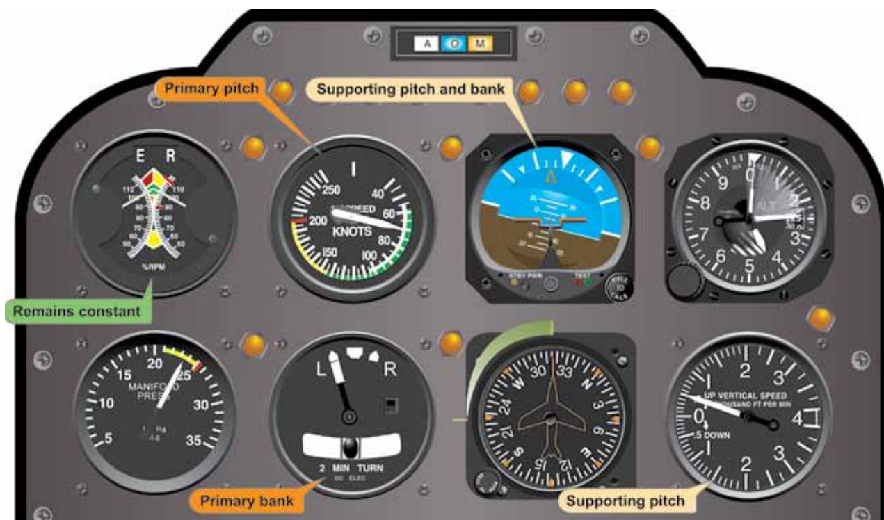
Figure 6-15. Flight Instrument Indications for a Stabilized Left Climbing Turn at a Constant Airspeed.
