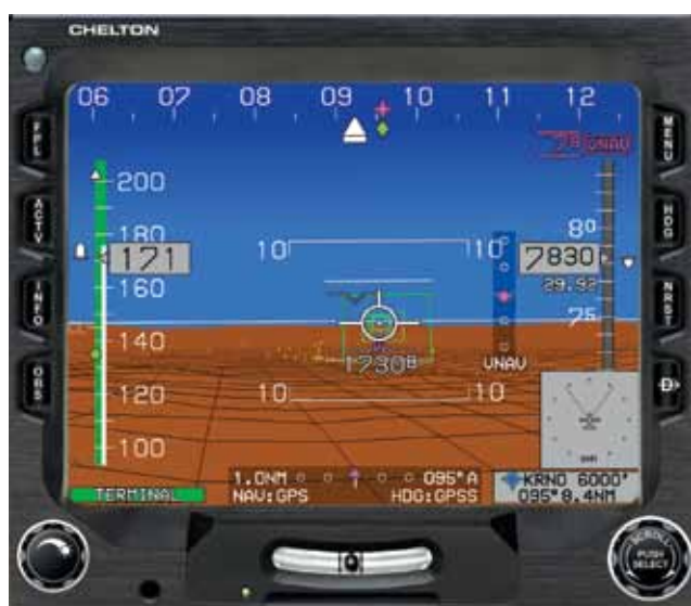
Figure 3-46. The benefits of realistic visualization imagery, as illustrated by Synthetic Vision manufactured by Chelton Flight Systems. The system provides the pilot a realistic, real-time, three-dimensional depiction of the aircraft and its relation to terrain around it.
