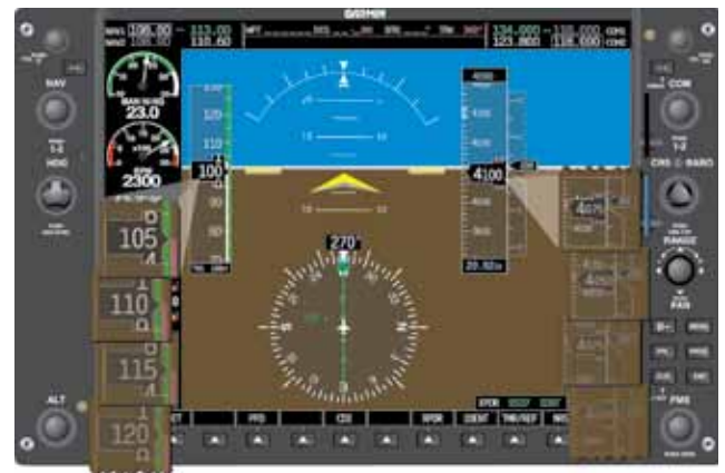
Figure 5-55. An aircraft decreasing in airspeed while gaining altitude. In this case, the pilot has decreased pitch.
