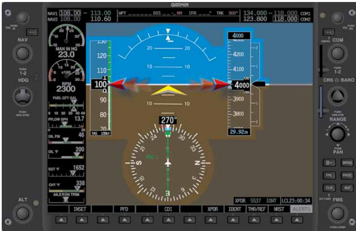
Figure 5-62. The pilot has fixated on pitch and altitude, leaving bank indications unattended. Note the trend line to the left.
