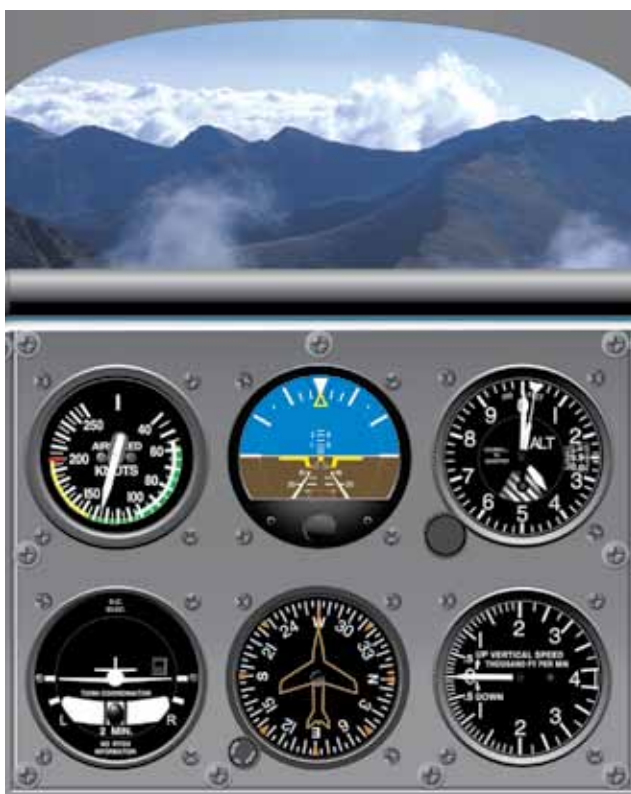
Figure 5-2. Pitch Attitude and Airspeed in Level Flight, Fast Cruise Speed.
