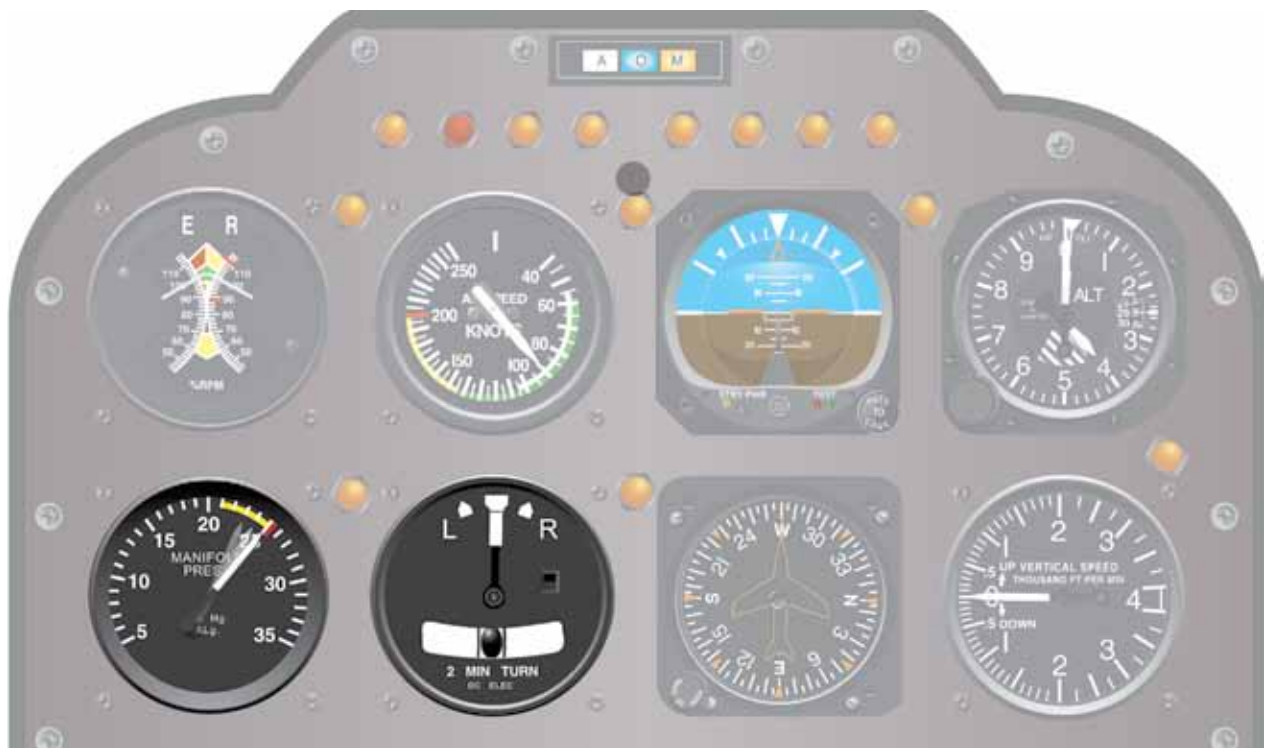
Figure 6-6. Coordinated flight is indicated by centering of the ball.
