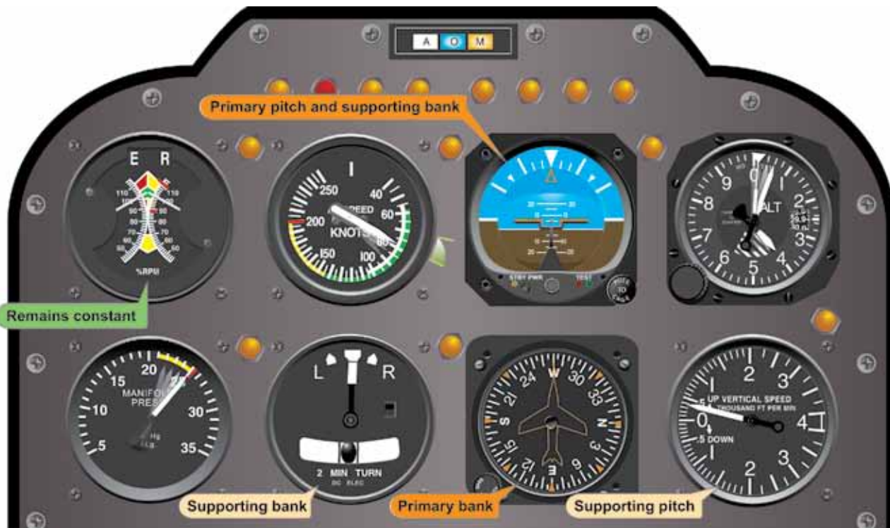
Figure 6-11. Flight instrument indications during climb entry for a constant-air-speed climb.
