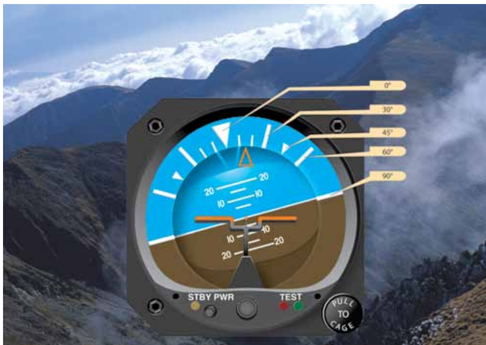
Figure 6-5. The banking scale at the top of the attitude indicator indicates varying degrees of bank. In this example, the helicopter is banked approximately 15^\circ to the right.
