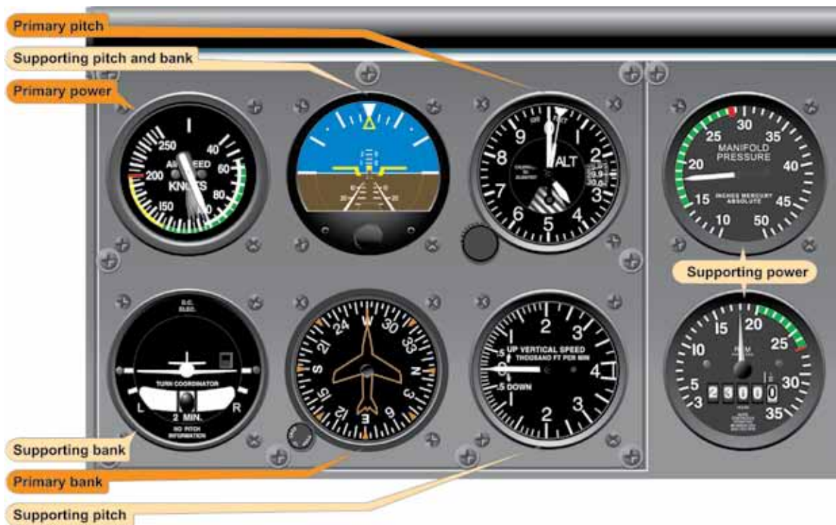
Figure 5-24. Straight-and-Level Flight (Reduced Airspeed Stabilized).
