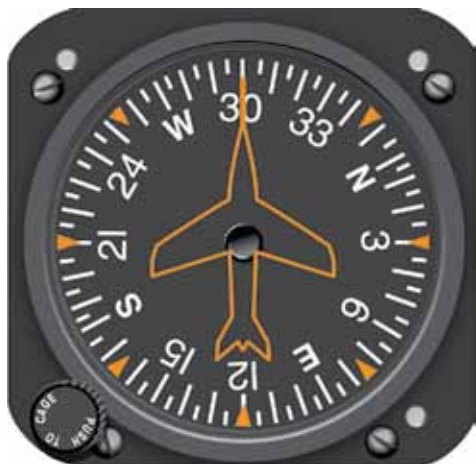
Figure 3-31. The heading indicator is not north seeking, but must be set periodically (about every 15 minutes) to agree with the magnetic compass.
