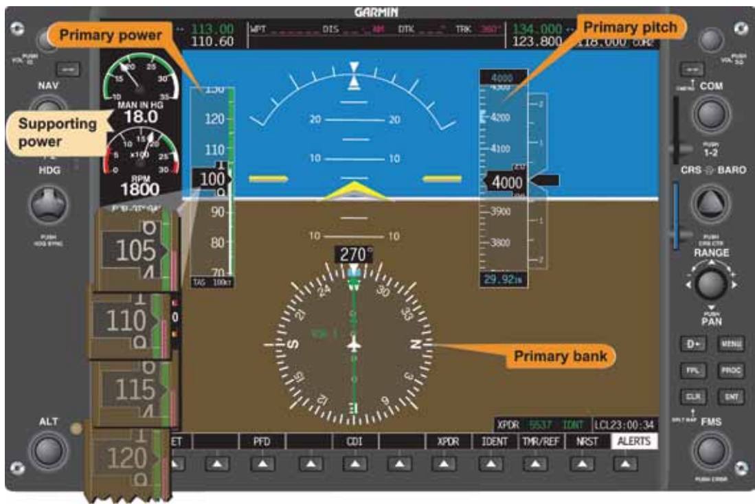
Figure 5-59. Straight-and-Level Flight (Reduced Airspeed Stabilized).
