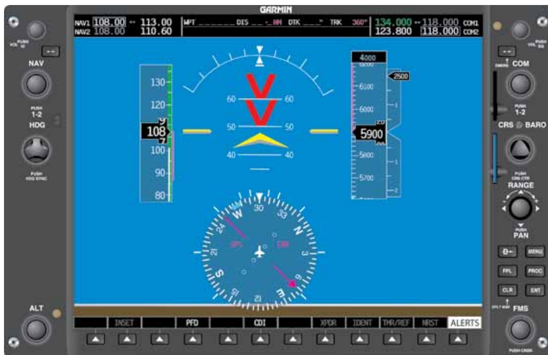
Figure 5-69. Unusual Attitude Recovery Protection. Note the brown horizon line is visible at the bottom.
