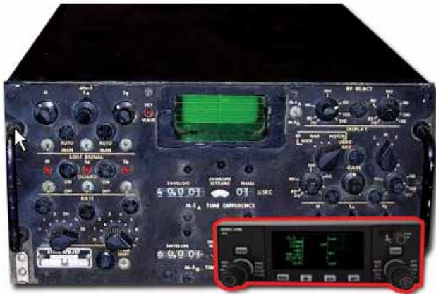
Figure 7-26. A control panel from a military aircraft after LORAN was first put into use. The receiver is remotely mounted and weighs over 25 pounds. Its size is about six times that of the LORAN fully integrated receiver.
