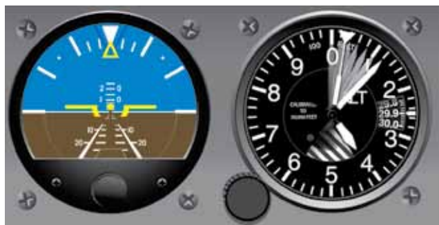
Figure 5-7. Using the Altimeter for Pitch Interpretation, a High Altitude Means a Nose-High Pitch Attitude.
