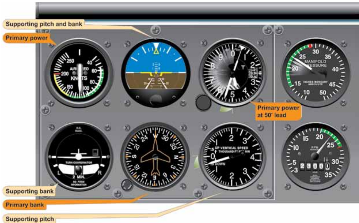
Figure 5-32. Level Off at Descent Airspeed.
