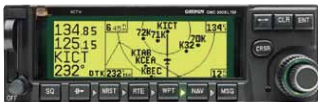
Figure 7-23. Onboard RNAV receivers have changed significantly. Originally, RNAV receivers typically computed combined data from VOR, VORTAC, and/or DME. That is generally not the case now. Today, GPS such as the GNC 300 and the Bendix King KLS 88 LORAN receivers compute waypoints based upon embedded databases and aircraft positional information.
