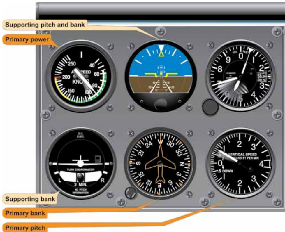
Figure 5-28. Airspeed Low and Vertical Speed High—Reduce Pitch.
