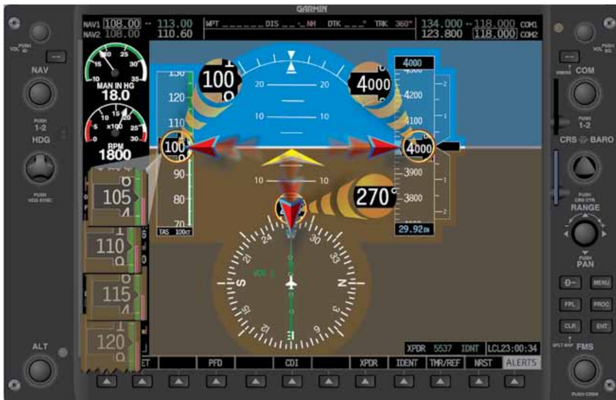
Figure 5-61. Insufficient cross-check. The problem is power and not nose-high. In this case, the pilot decreased pitch inappropriately.
