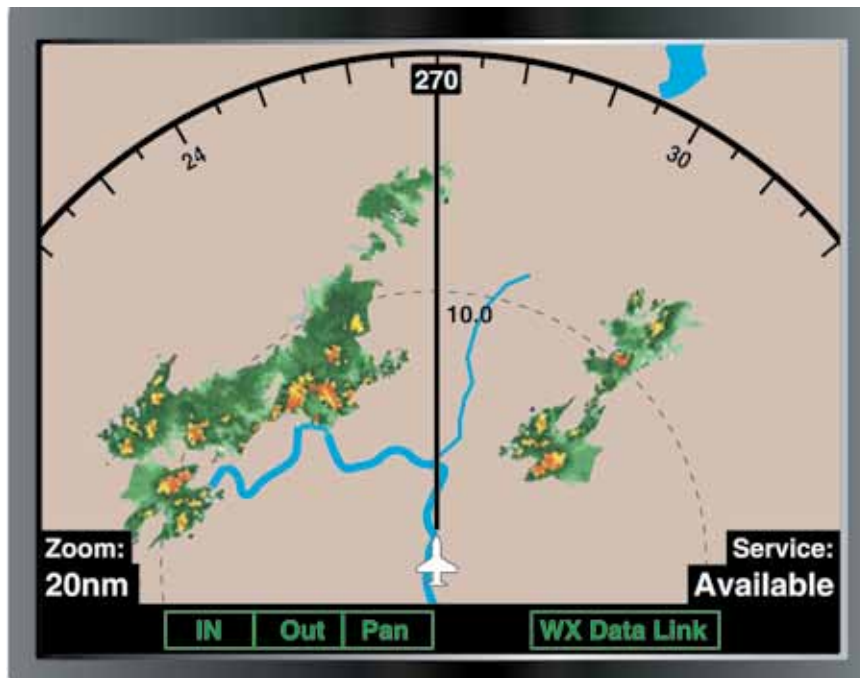
Figure 3-50. An aircraft equipped with ADS has the ability to upload and display weather.
