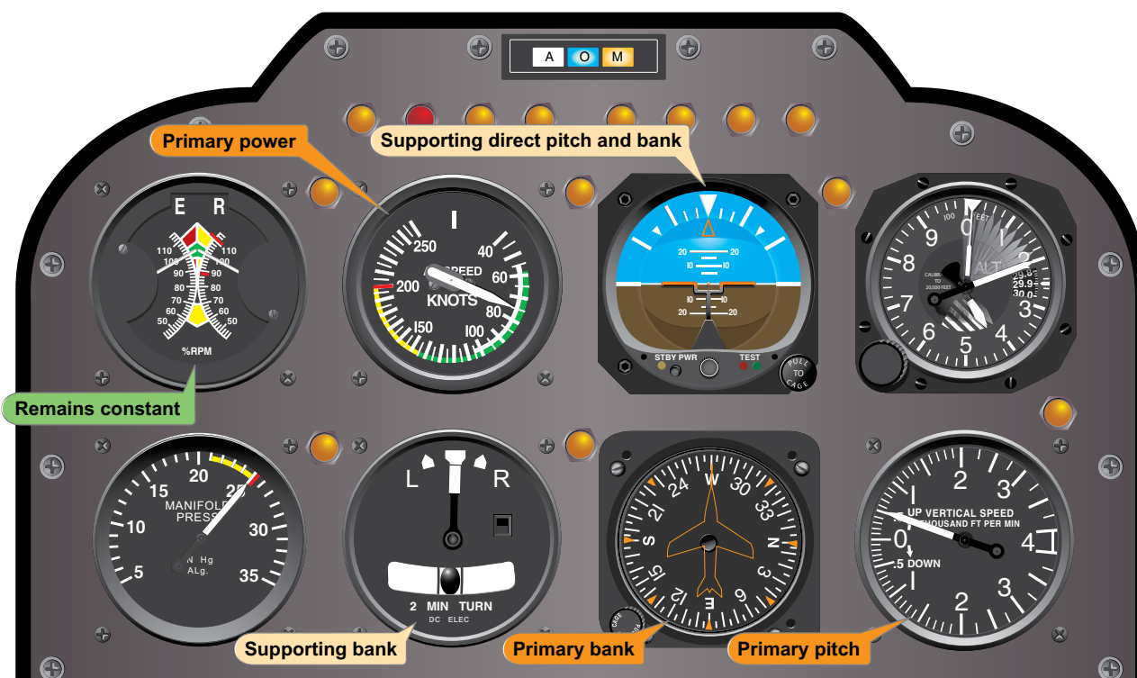
Figure 6-13. Flight Instrument Indications in a Stabilized Constant-Rate Climb.
