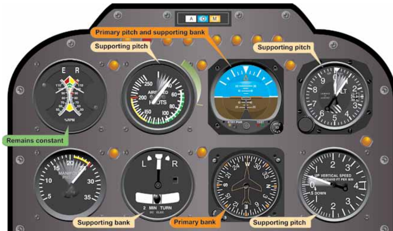
Figure 6-16. Flight Instrument Indications During an Instrument Takeoff.
