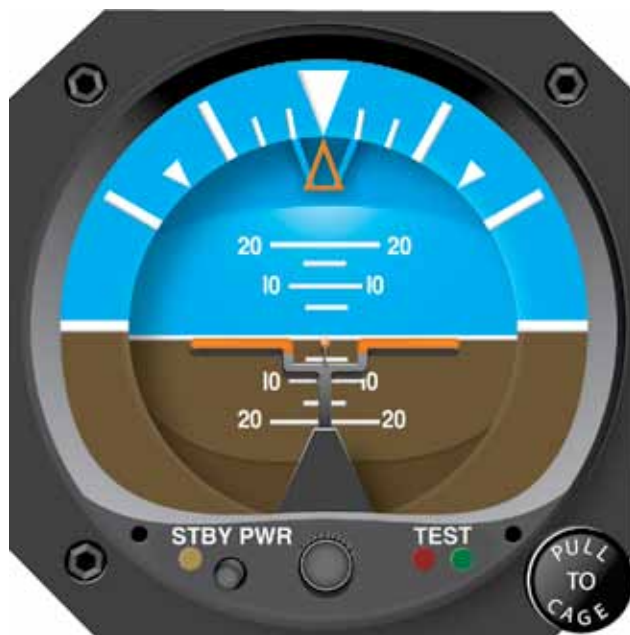
Figure 6-3. The initial pitch correction at normal cruise is one bar width or less.
