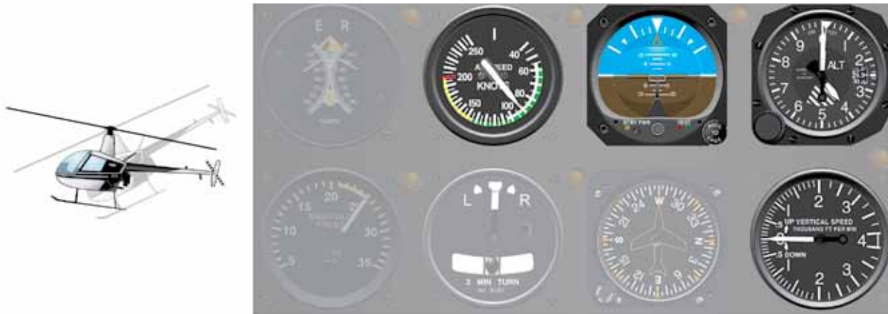
Figure 6-2. The flight instruments for pitch control are the airspeed indicator, attitude indicator, altimeter, and vertical speed indicator.
