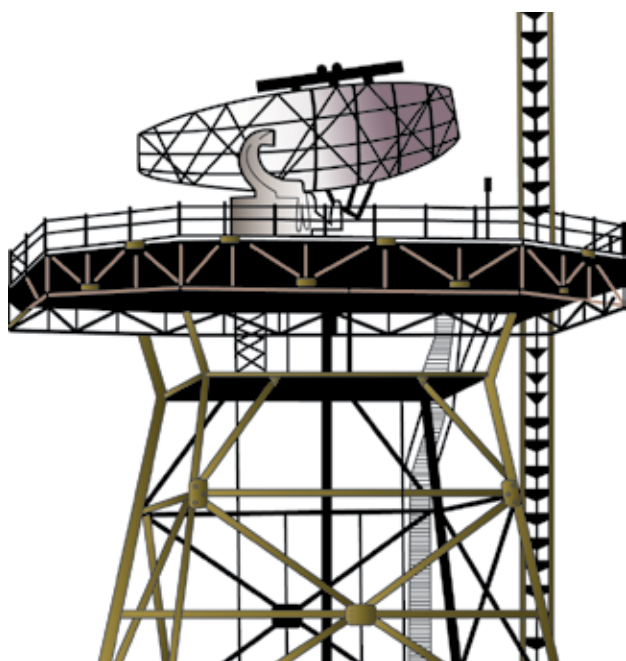
Figure 9-7. Combined Radar and Beacon Antenna.
