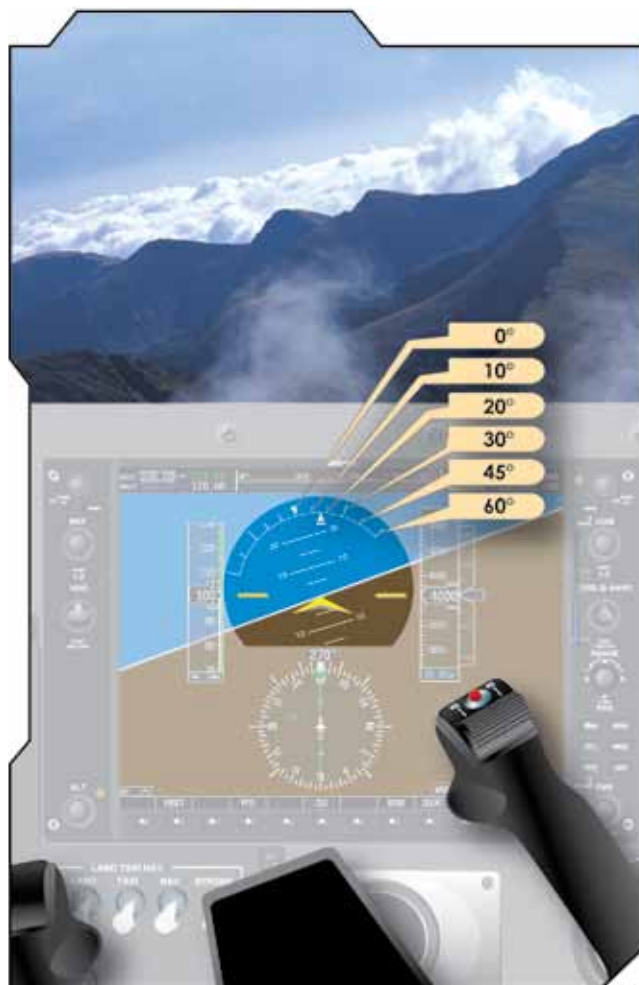
Figure 4-29. Bank Control Index Lines.
