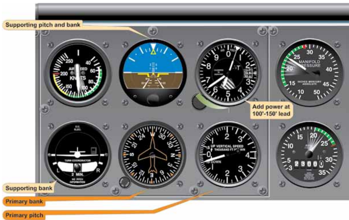
Figure 5-31. Level Off Airspeed Higher Than Descent Airspeed.
