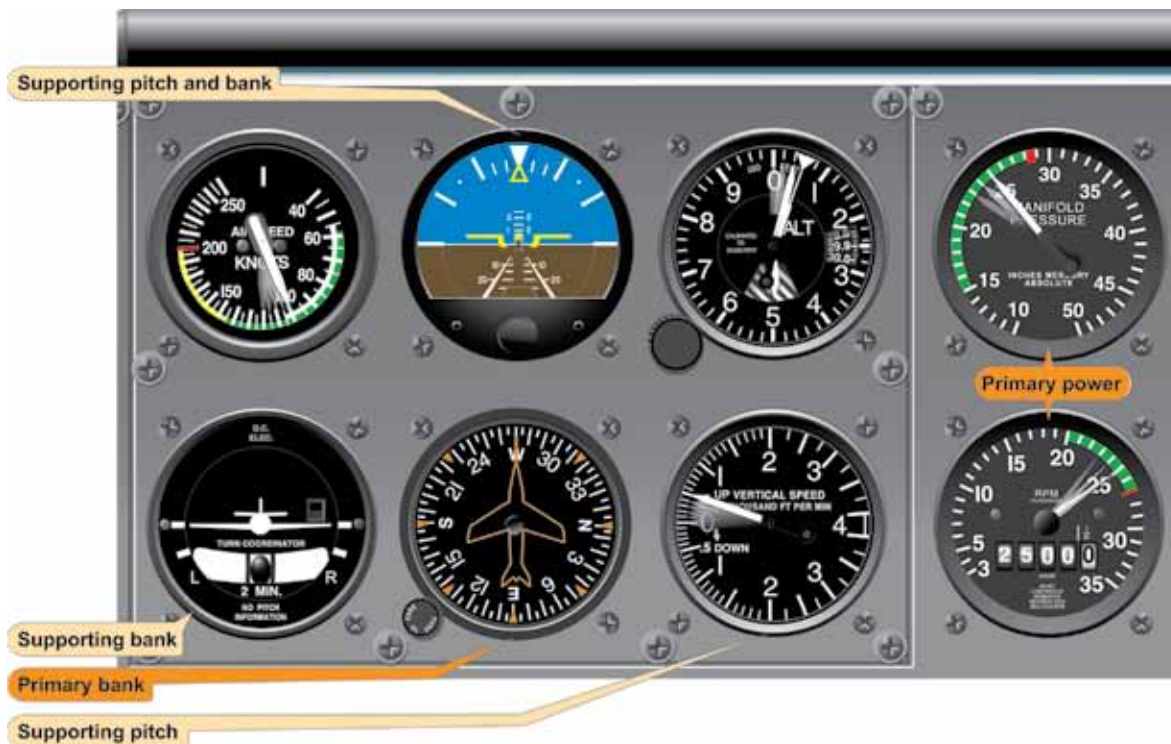
Figure 5-25. Climb Entry for Constant Airspeed Climb.
