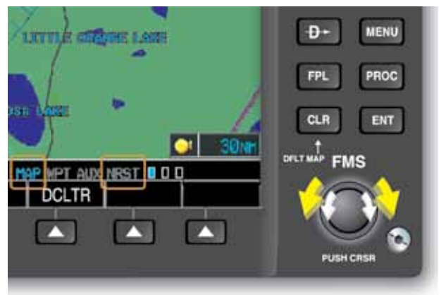
Figure 11-14. Page Groups. As the FMS outer knob is rotated, the current page group is indicated by highlighting the specific group indicator. Notice that the MAP page group is highlighted.
