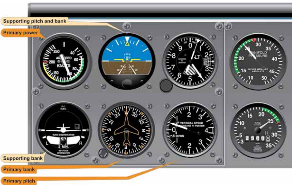
Figure 5-27. Stabilized Climb at Constant Rate.
