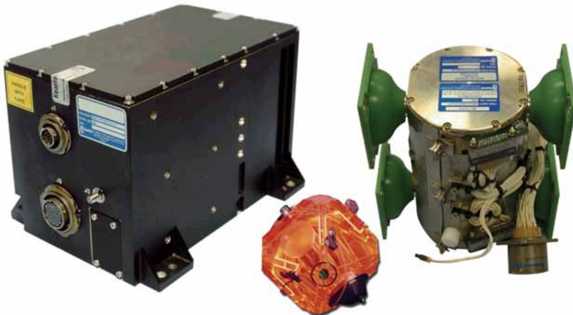
Figure 3-36. The Kearfott Attitude Heading Reference System (AHRS) on the left incorporates a Monolithic Ring Laser Gyro (MRLG) (center), which is housed in an Inertial Sensor Assembly (ISA) on the right.
