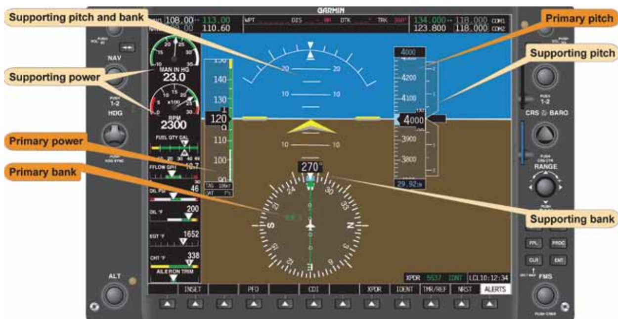
Figure 5-57. Straight-and-Level Flight (Normal Cruising Speed).
