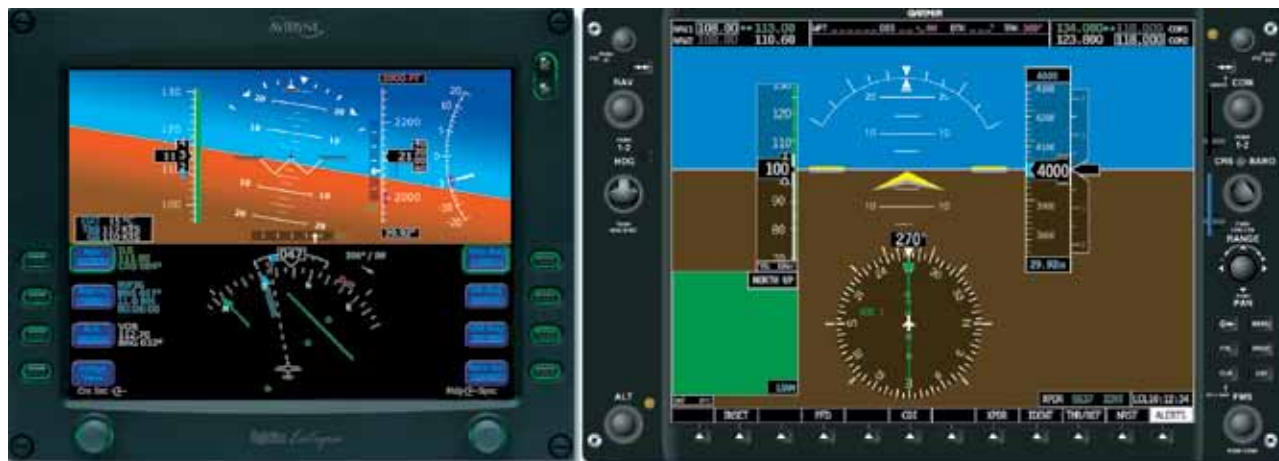
Figure 3-45. Two Primary Flight Displays (Avidyne on the Left and Garmin on the Right).
