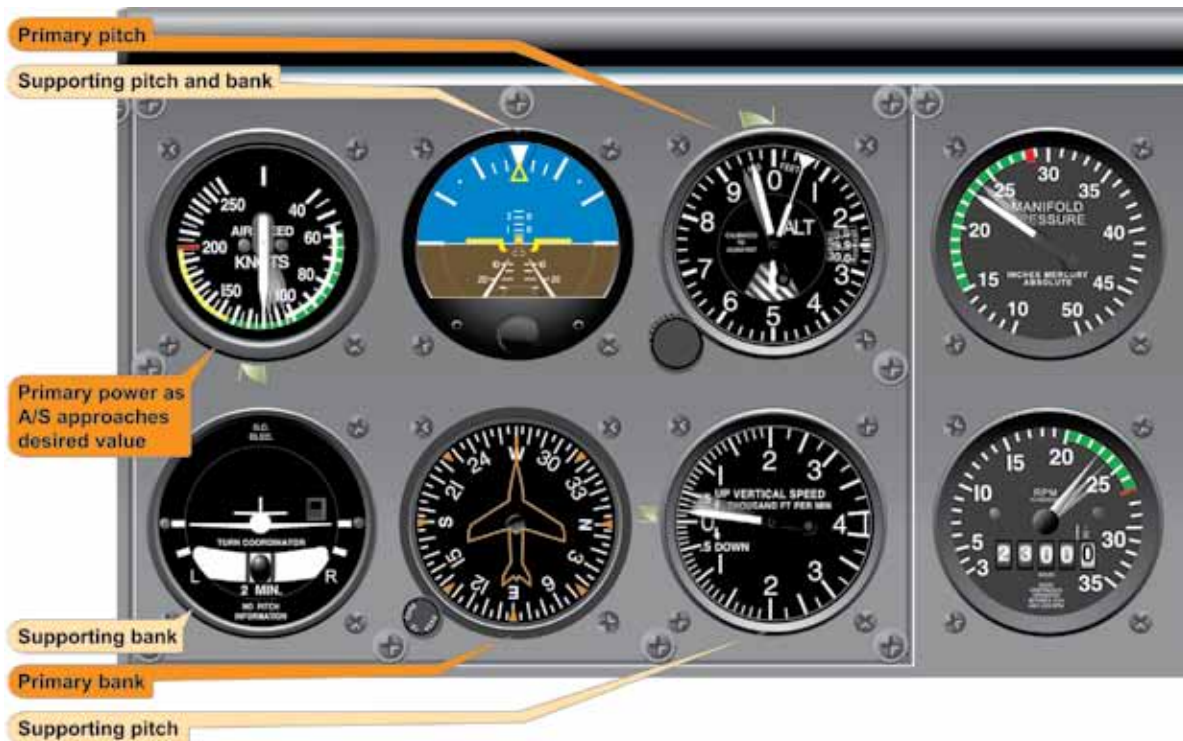
Figure 5-29. Level Off at Cruising Speed.
