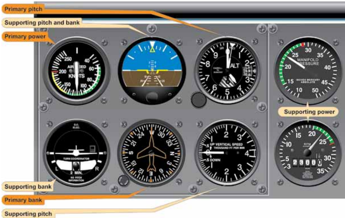
Figure 5-22. Straight-and-Level Flight (Normal Cruising Speed).
