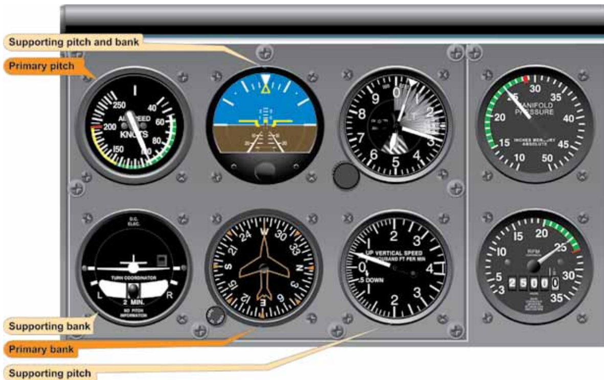
Figure 5-26. Stabilized Climb at Constant Airspeed.
