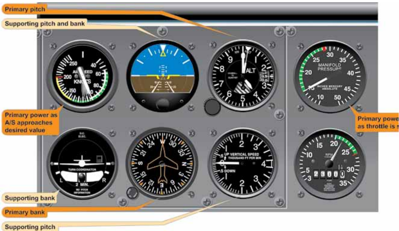
Figure 5-23. Straight-and-Level Flight (Airspeed Decreasing).
