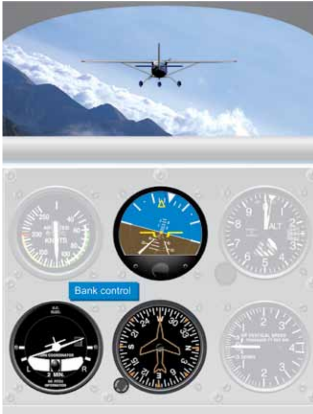
Figure 5-16. Instruments Used for Bank Control.
