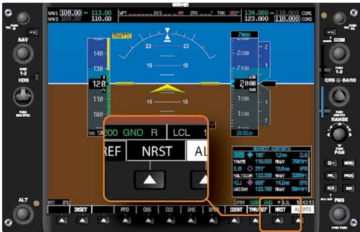
Figure 11-9. The default soft key menu that is displayed on the PFD contains a “NRST” (Nearest Airport) soft key. Pressing this soft key opens a text box which displays the nearest 25 airports.
