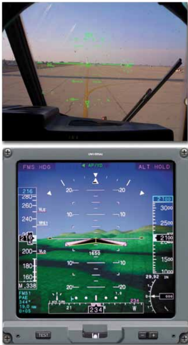
Figure 7-44. Example of a Head-Up Display (top) and a Head-Down Display (bottom). The head-up display presents information in front of the pilot along his/her normal field of view while a head-down display may present information beyond the normal head-up field of view.
