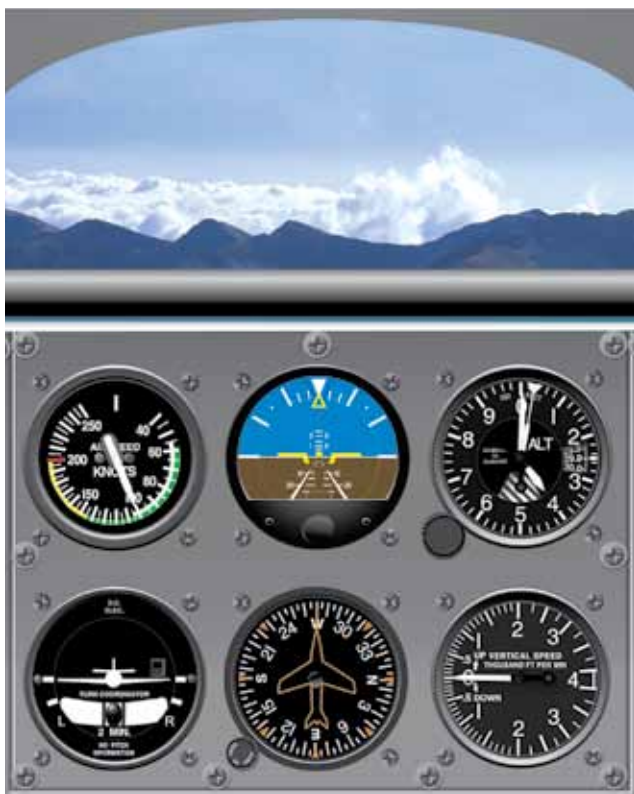
Figure 5-1. Pitch Attitude and Airspeed in Level Flight, Slow Cruise Speed.
