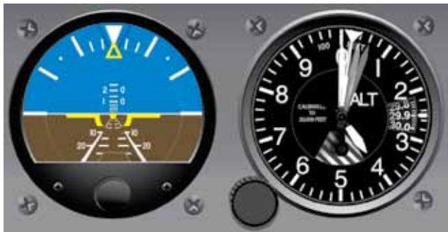
Figure 5-10. Pitch Correction, Less Than 100 Feet—One-Half Bar Low to Correct Altitude Error.
