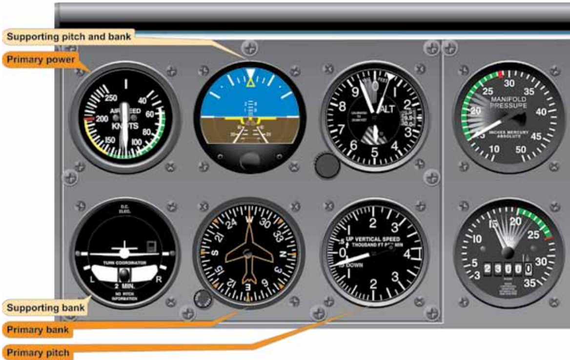
Figure 5-30. Constant Airspeed Descent, Airspeed High—Reduce Power.
