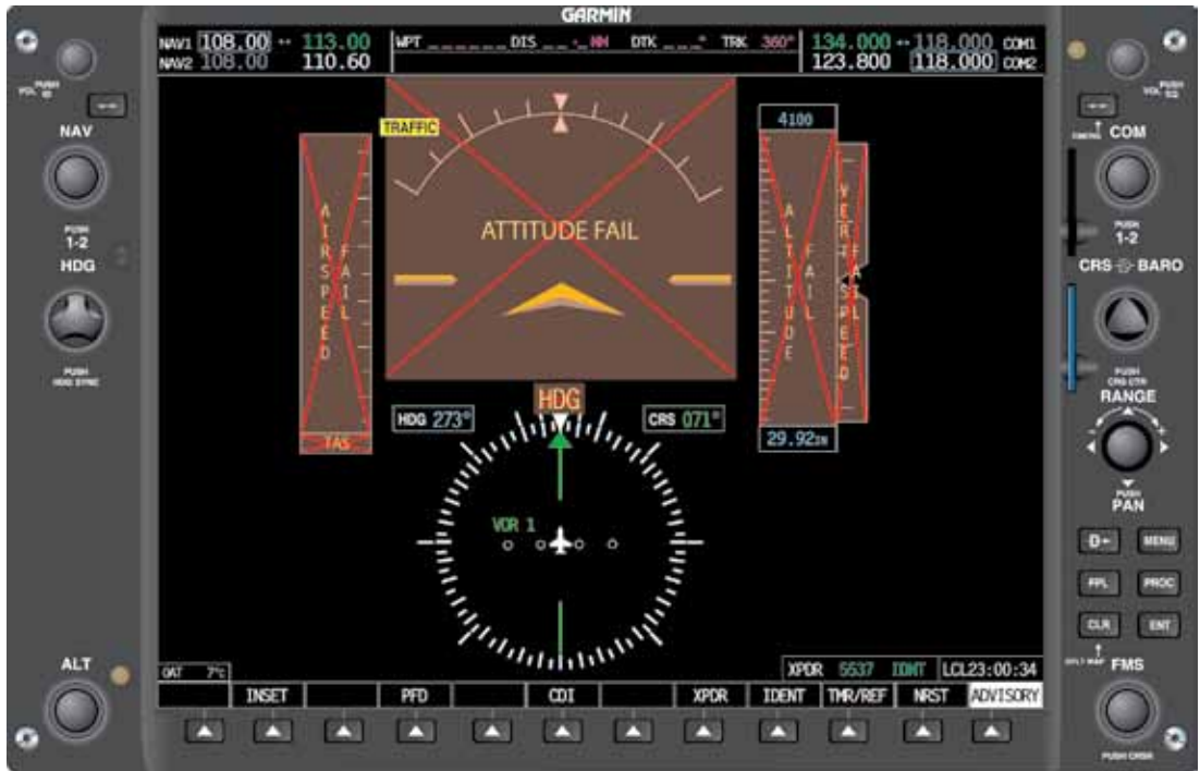
Figure 5-74. AHRS ADC Failure.
