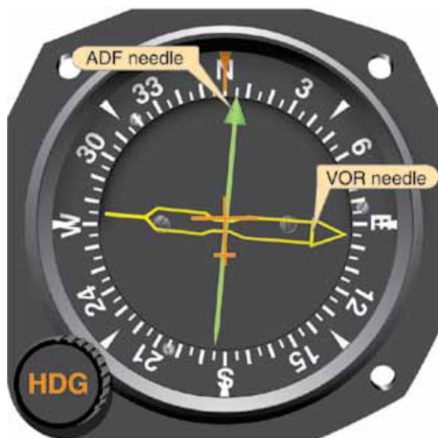
Figure 7-5. Radio magnetic indicator (RMI). Because the aircraft's magnetic heading is automatically changed, the relative bearing (RB), in this case 095°, will indicate the magnetic bearing (095°) to the station (no wind conditions) and the magnetic heading that will take you there.
