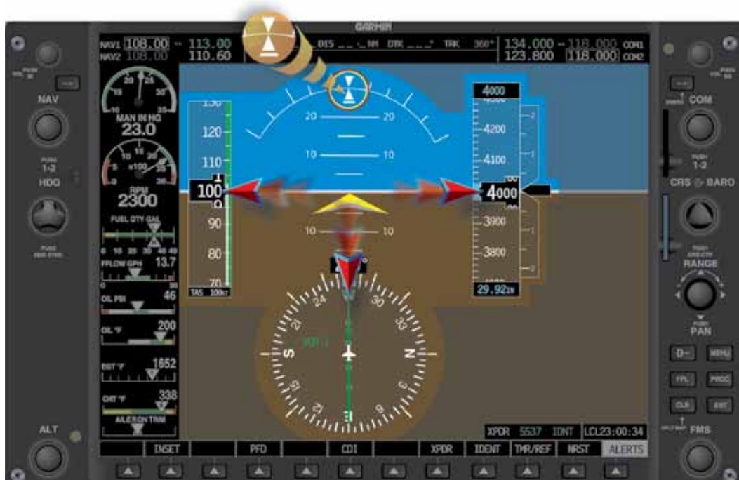
Figure 4-34. Selected Radial Cross-Check.
