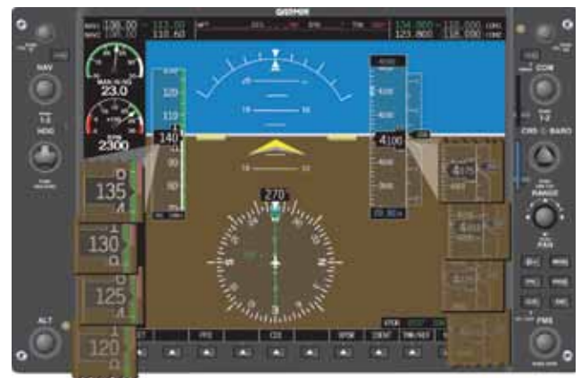
Figure 5-56. Figure shows both an increase in speed and altitude where pitch adjustment alone is insufficient. In this situation, a reduction of power is also necessary.
