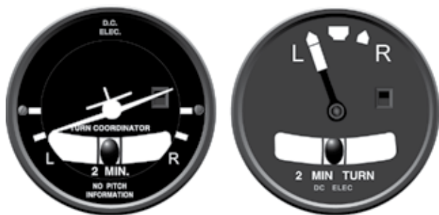
Figure 4-12. Turn Coordinator and Turn-and-Slip Indicator.
