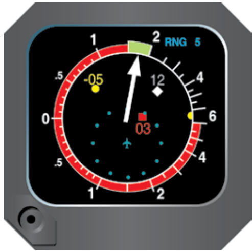
Figure 3-58. An example of a resolution advisory being provided the pilot. In this case, the pilot is requested to climb, with 1,750 feet being the appropriate rate of ascent to avoid traffic conflict. This visual indication plus the aural warning provide the pilot with excellent traffic awareness that augments see and avoid practices.
