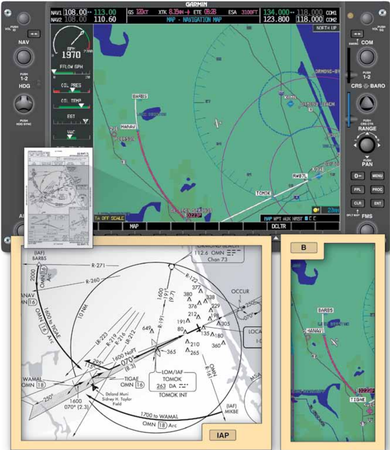
Figure 7-19. An aircraft is displayed heading southwest to intercept the localizer approach, using the 16 NM DME Arc off of ORM.
