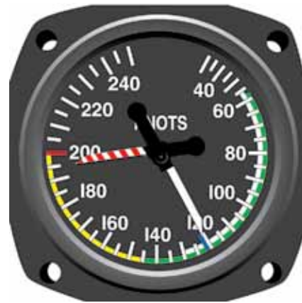
Figure 3-14. A maximum allowable airspeed indicator has a movable pointer that indicates the never-exceed speed, which changes with altitude to avoid the onset of transonic shock waves.
