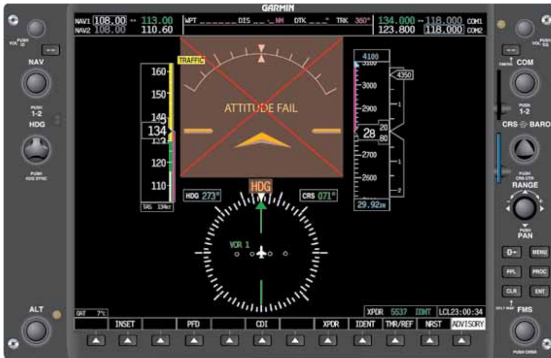
Figure 5-73. AHRS Unit Failed.
