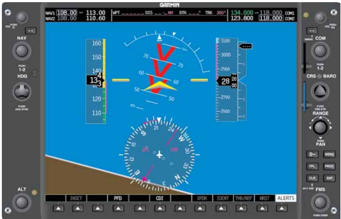
Figure 5-72. Unusual Attitude Protection With Valid AHRS.
