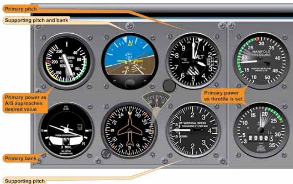
Figure 5-38. Change of Airspeed During Turn.
