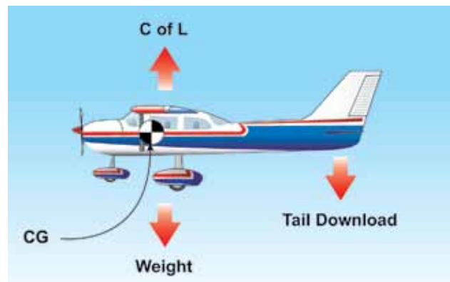
Figure 2-21. Downward Force on the Tailplane.
