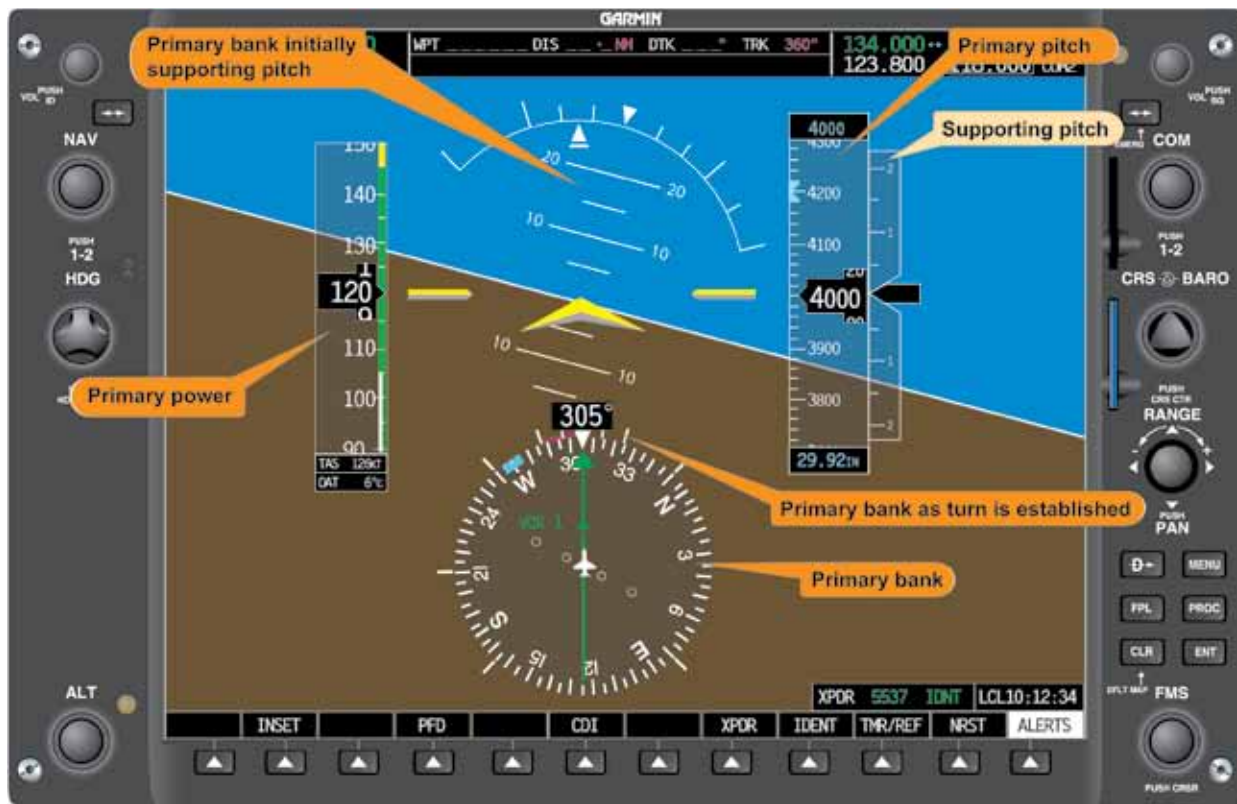
Figure 5-67. Standard Rate Turn—Constant Airspeed.
