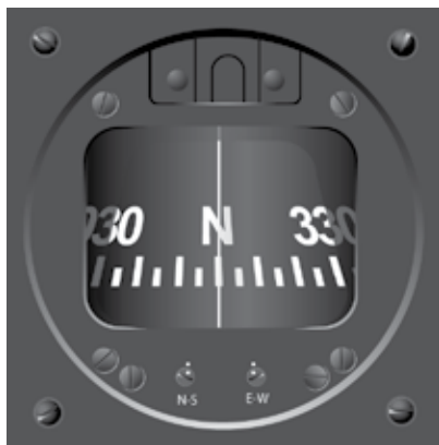
Figure 3-16. A Magnetic Compass. The vertical line is called the lubber line.
