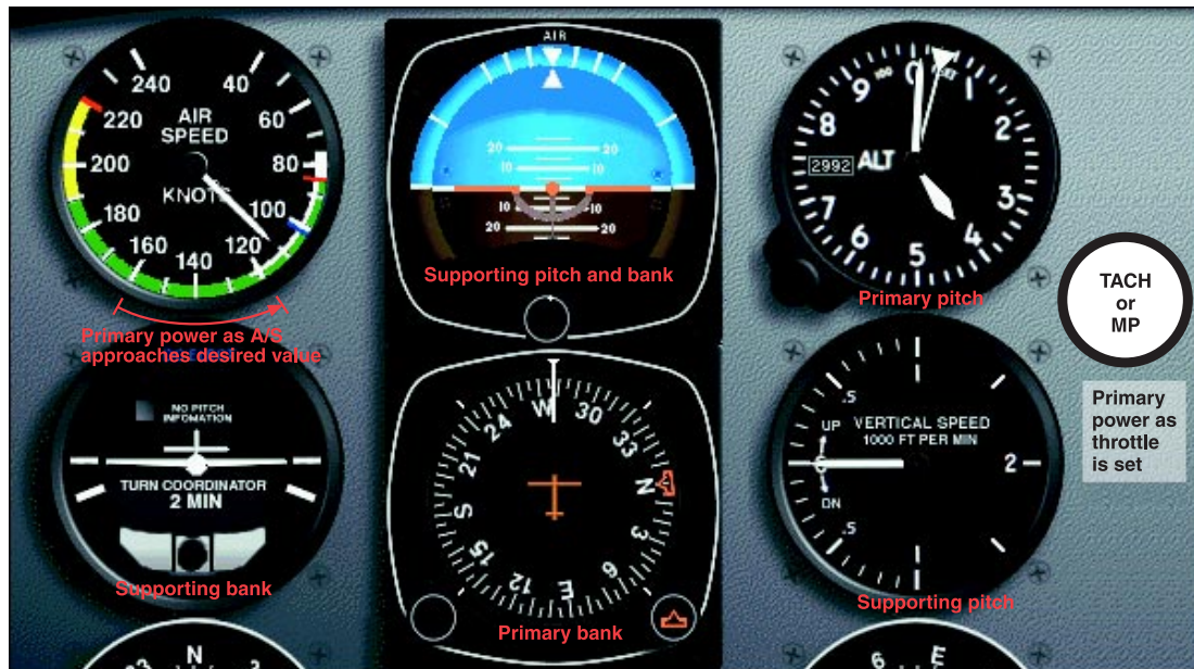
Figure 5-23. Straight-and-level flight (airspeed decreasing).
