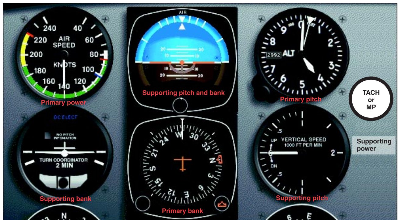
Figure 5-22. Straight-and-level flight (normal cruising speed).
