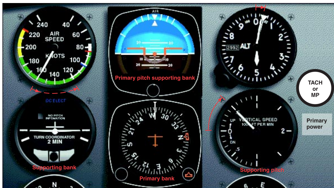
Figure 5-25. Climb entry for constant-airspeed climb.
