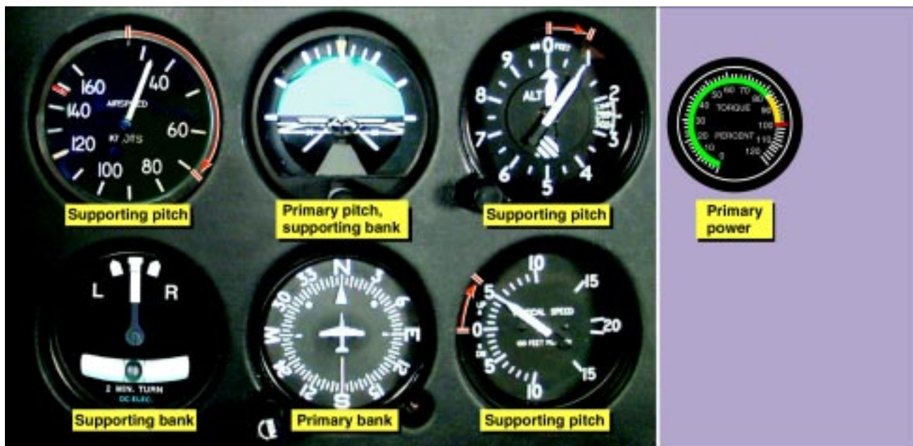
Figure 6-13. Flight instrument indications during an instrument takeoff.
