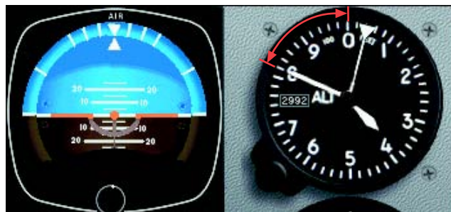
Figure 5-11. Altitude error, greater than 100 feet.
