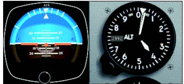
Figure 5-10. Pitch correction, less than 100 feet—1/2 bar low to correct altitude error.
