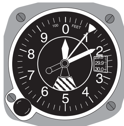
Figure 3-4. Three-pointer altimeter.
