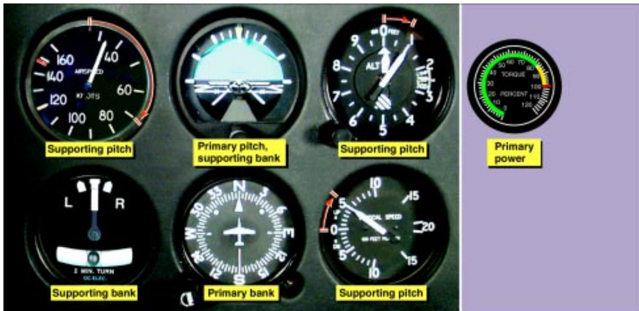
Figure 6-13. Flight instrument indications during an instrument takeoff.
