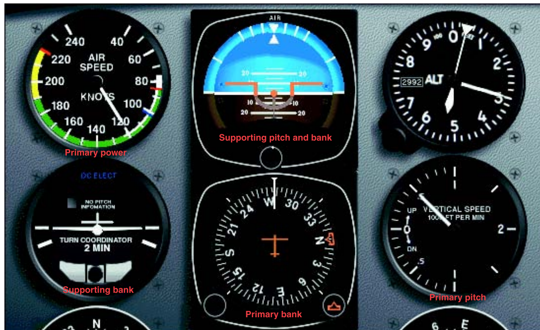
Figure 5-27. Stabilized climb at constant rate.
