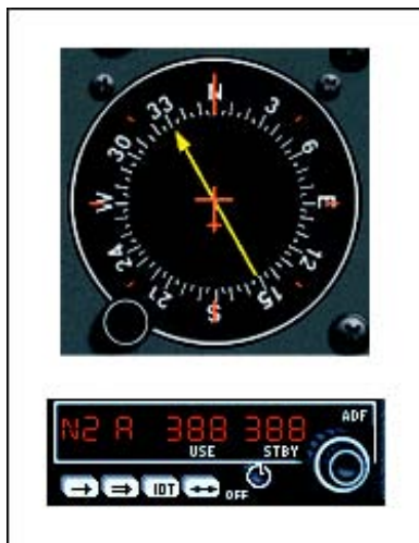
Figure 7-2. ADF indicator instrument and receiver.
