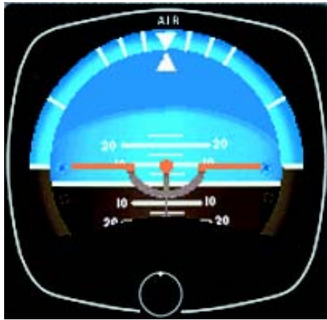
Figure 3-29. The dial of this attitude indicator has reference lines to show pitch and roll.
