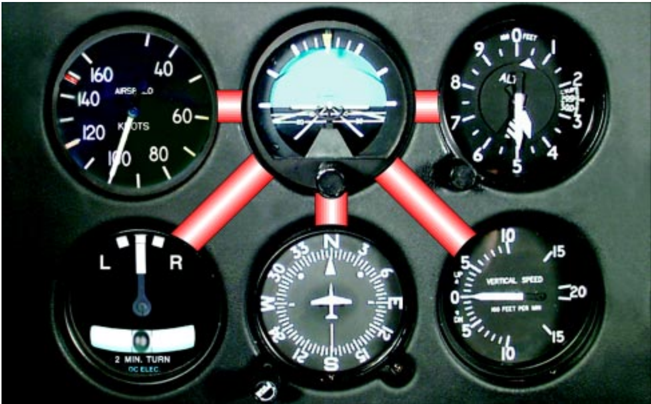
Figure 6-1. In most situations, the cross-check pattern includes the attitude indicator between the cross-check of each of the other instruments. A typical cross-check might progress as follows: attitude indicator; altimeter; attitude indicator; vertical speed indicator; attitude indicator; heading indicator; attitude indicator; and so on.
