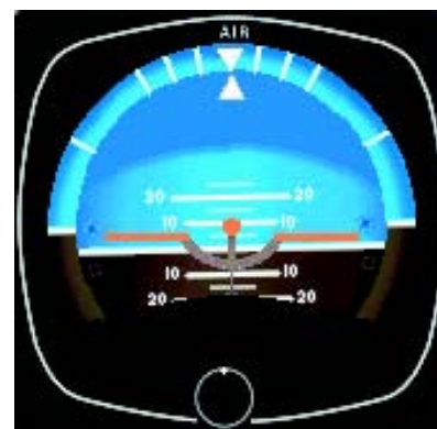
Figure 5-5. Pitch correction for level flight, two-bar width.
