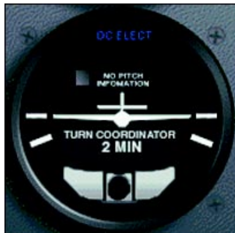
Figure 3-34. A turn coordinator senses rotation about both the roll and yaw axes.
