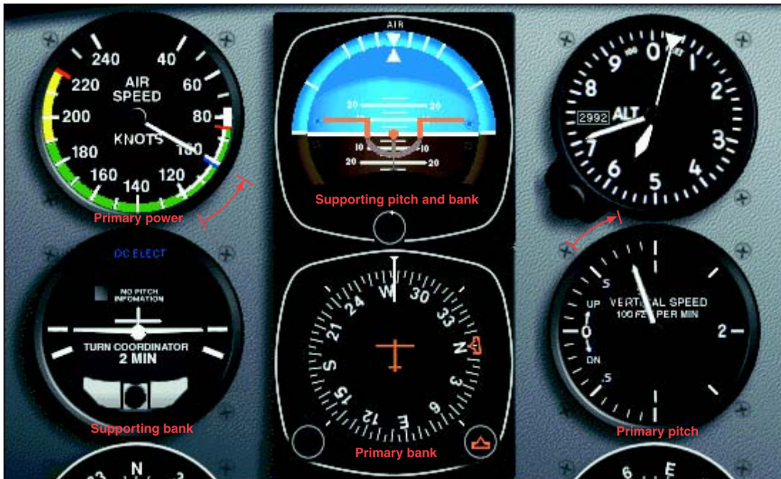
Figure 5-28. Airspeed low and vertical speed high—reduce pitch.
