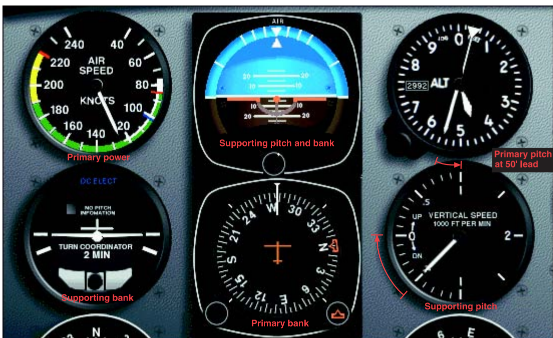
Figure 5-32. Level-off at descent airspeed.
