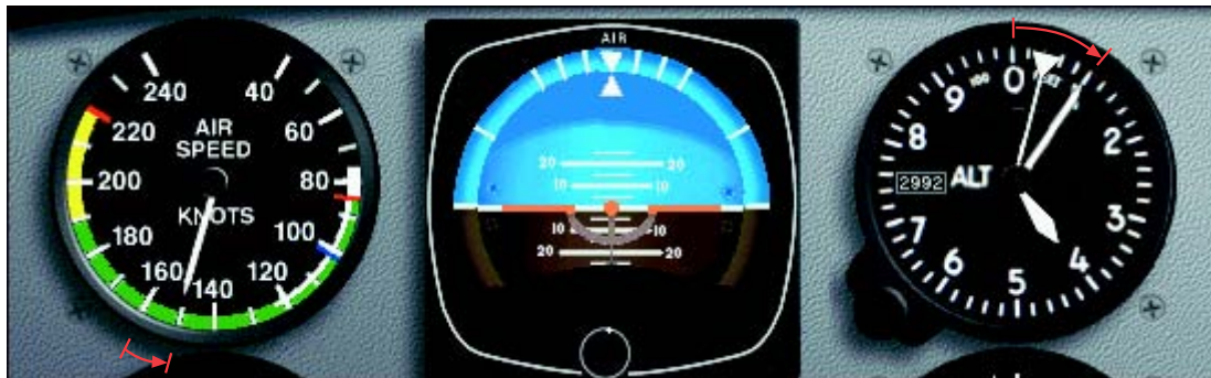
Figure 5-20. Airspeed low and altitude high (lower pitch).
