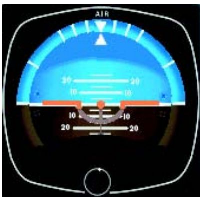
Figure 5-4. Pitch correction for level flight, half-bar width.
