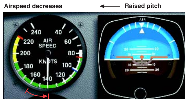
Figure 5-15. Constant power plus increased pitch equals decreased airspeed.
