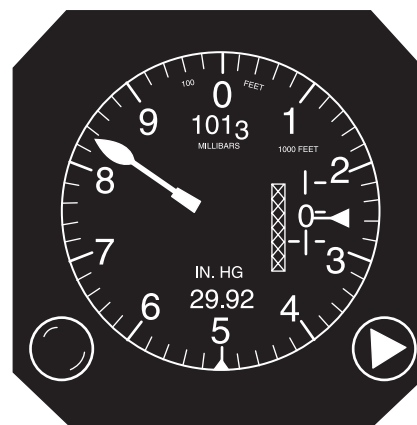
Figure 3-5. Drum-type altimeter.
