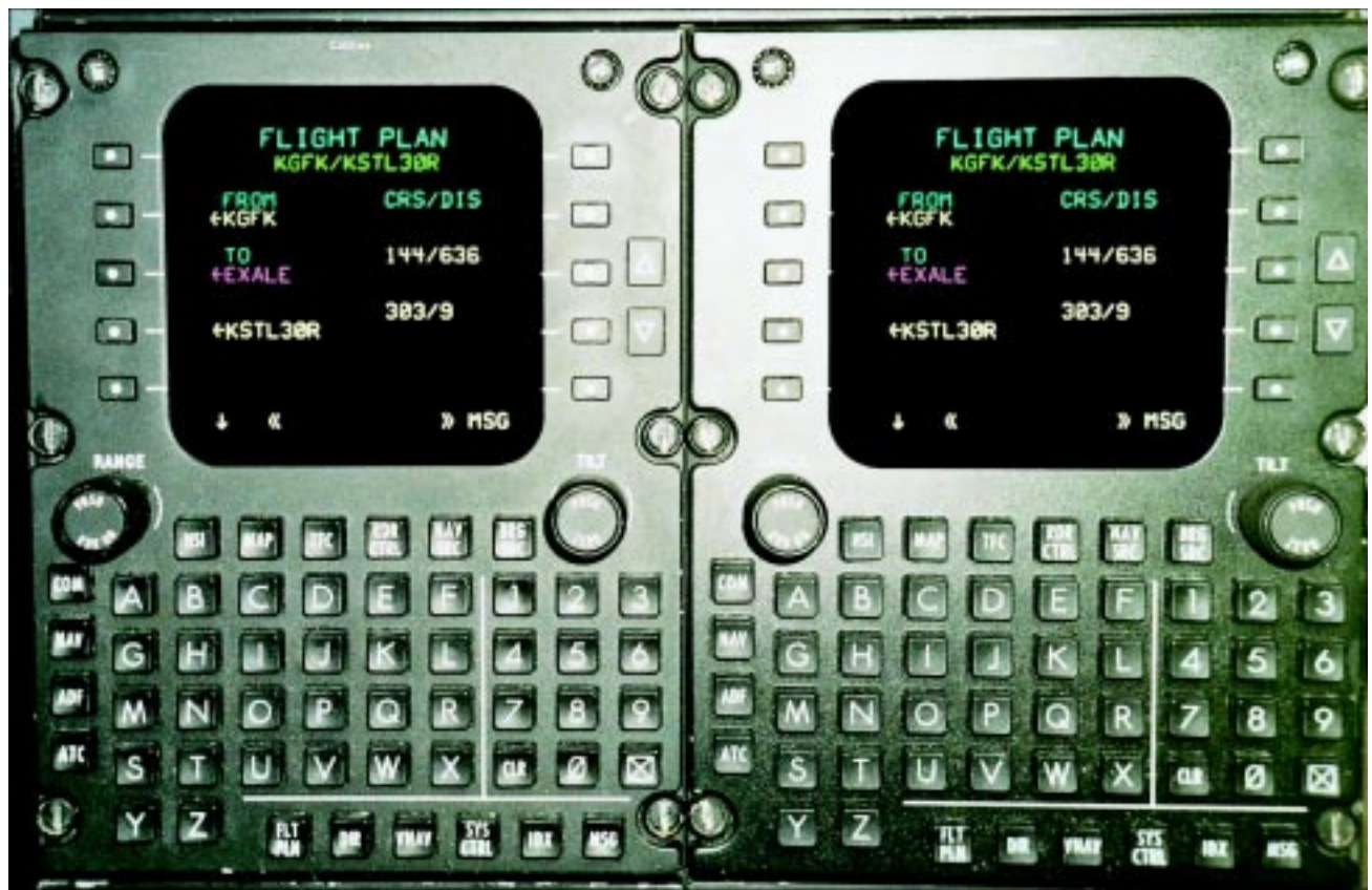
Figure 7-31. FMS CDU in flight plan mode.
