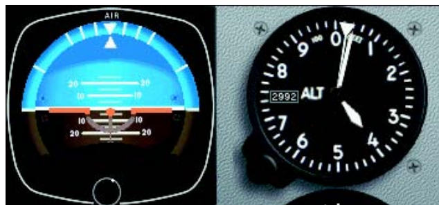
Figure 5-10. Pitch correction, less than 100 feet—1/2 bar low to correct altitude error.
