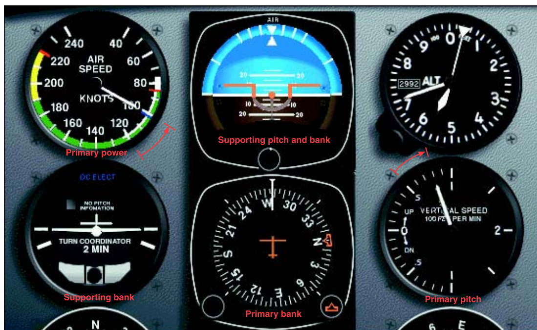
Figure 5-28. Airspeed low and vertical speed high—reduce pitch.
