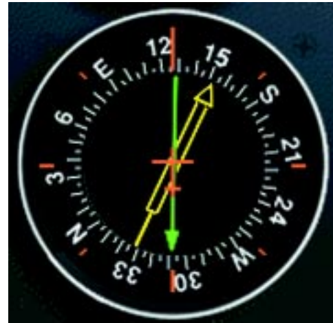
Figure 3-25. The compass card in this RMI is driven by signals from a flux valve and it indicates the heading of the aircraft opposite the upper center index mark.
