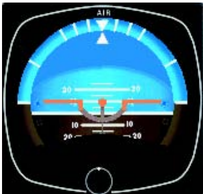
Figure 5-6. Pitch correction for level flight, three-bar width.
