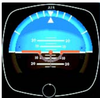
Figure 5-4. Pitch correction for level flight, half-bar width.
