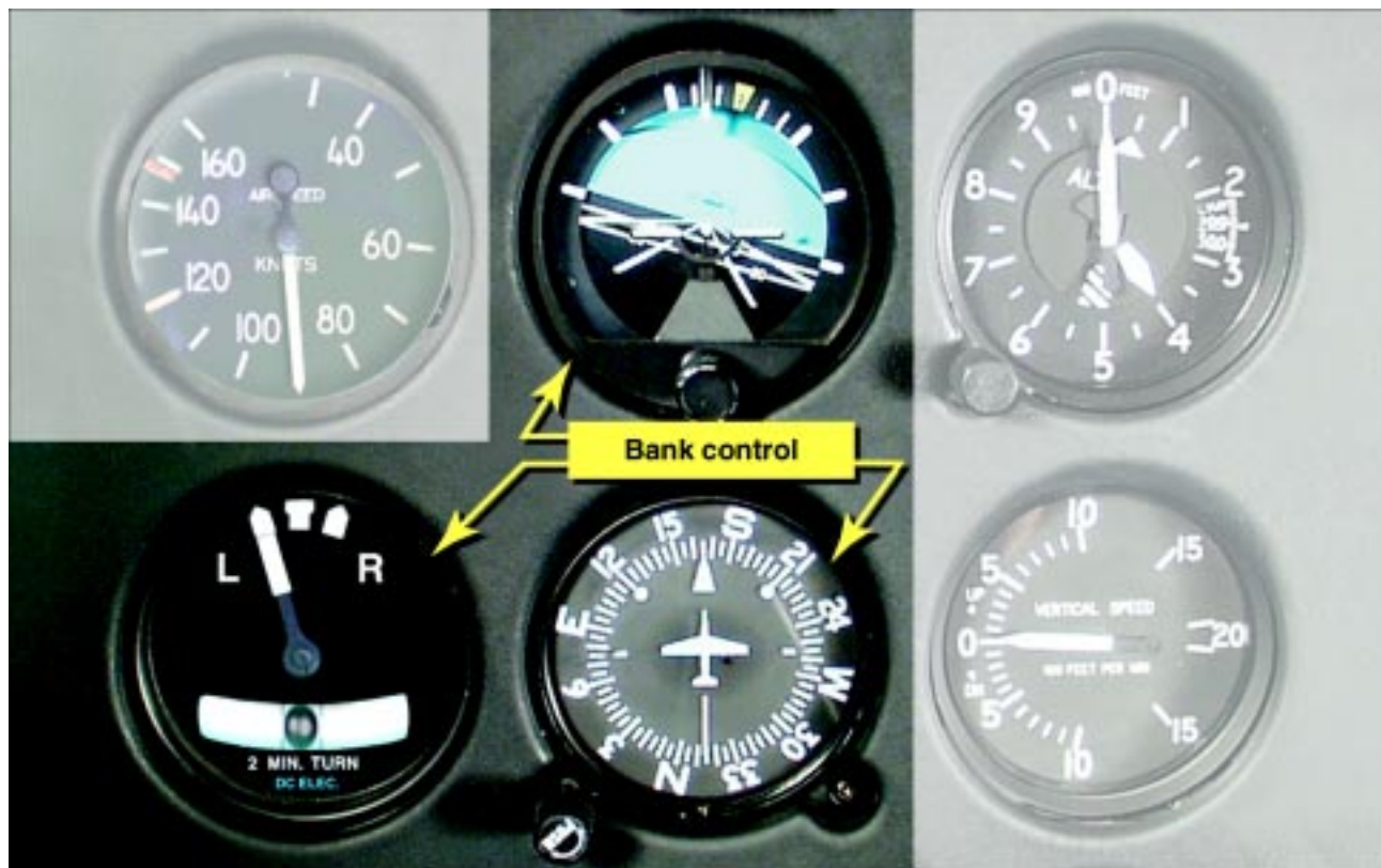
Figure 6-4. The flight instruments used for bank control are the attitude, heading, and turn indicators.
