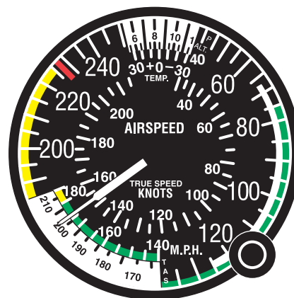
Figure 3-10. A true airspeed indicator allows the pilot to correct indicated airspeed for nonstandard temperature and pressure.
