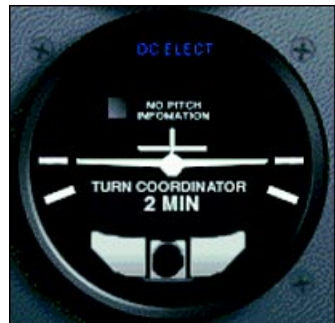
Figure 3-34. A turn coordinator senses rotation about both the roll and yaw axes.
