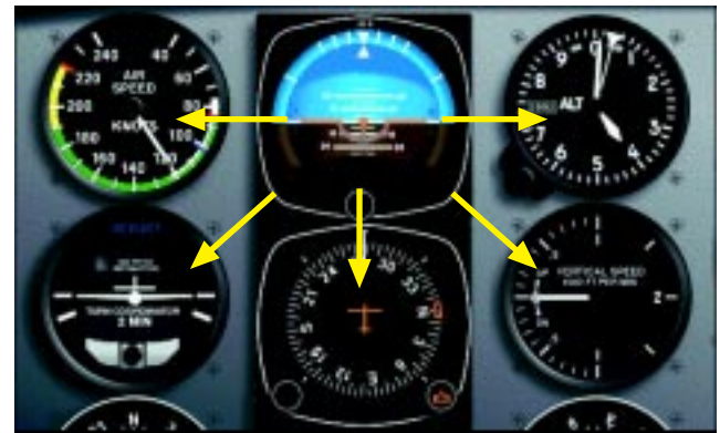
Figure 4-3. Selected radial cross-check pattern.
