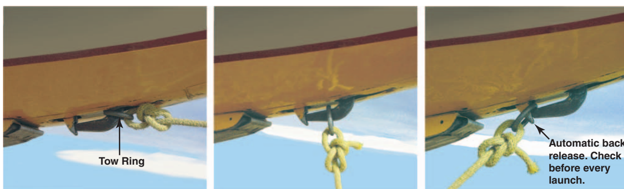
Figure 7-13. Testing the towhook.
