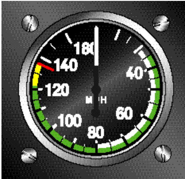
Figure 4-3. Airspeed indicator with color markings.
