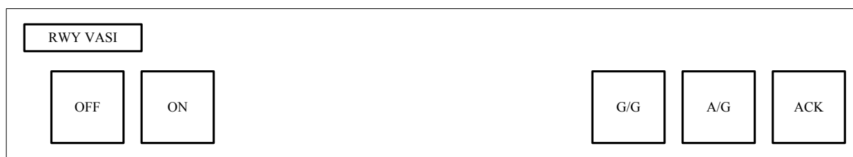
Figure 18. Conceptual VASI ribbon display
