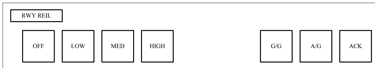
Figure 17. Conceptual REIL ribbon display
