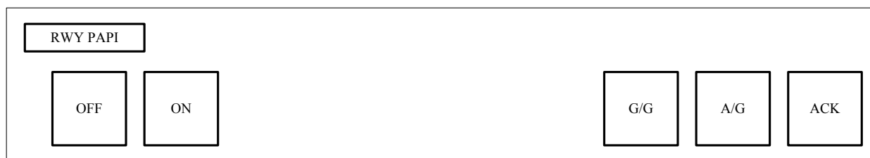
Figure 16. Conceptual PAPI ribbon display
