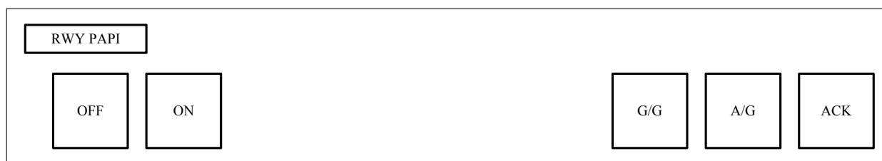
Figure 21. Conceptual TCU PAPI ribbon display
