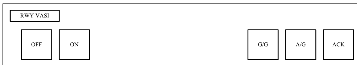
Figure 23. Conceptual TCU VASI ribbon display
