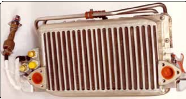
Figure 6-42. Air oil cooler.
