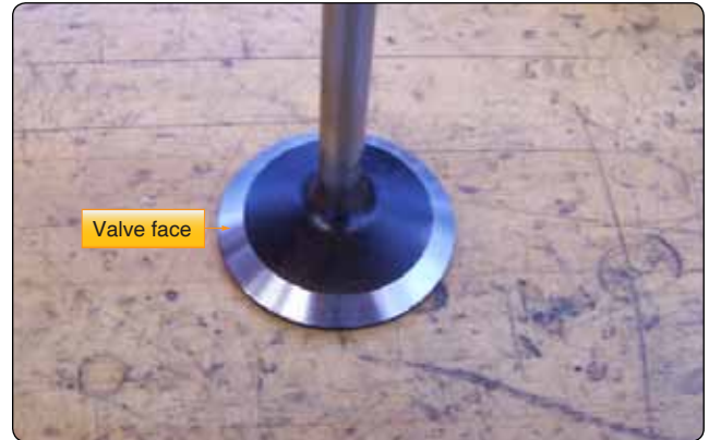
Figure 10-15. Valve face surface.
