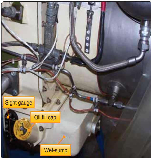
Figure 6-47. Typical turbine wet sump system.
