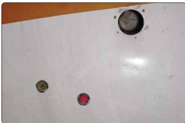
Figure 9-11. Discharge indicators.
