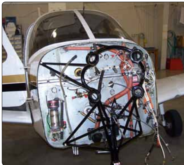
Figure 8-2. Typical firewall with components mounted on it.
