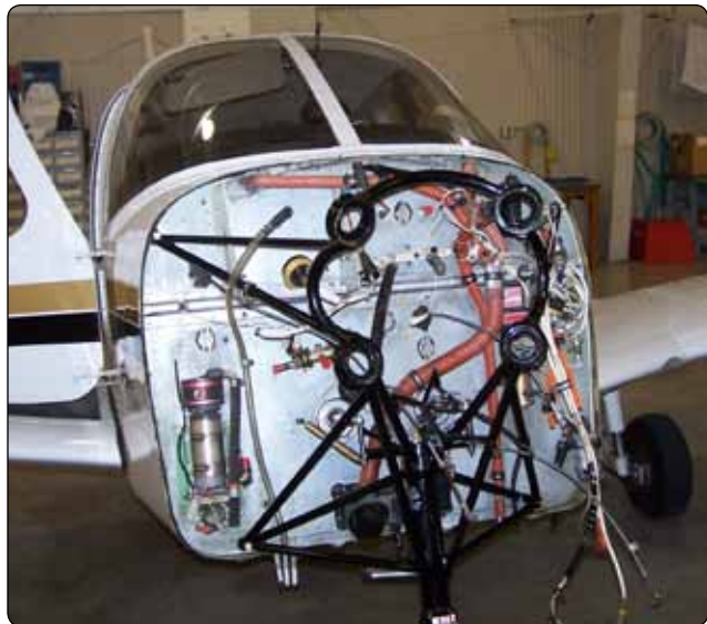
Figure 8-2. Typical firewall with components mounted on it.
