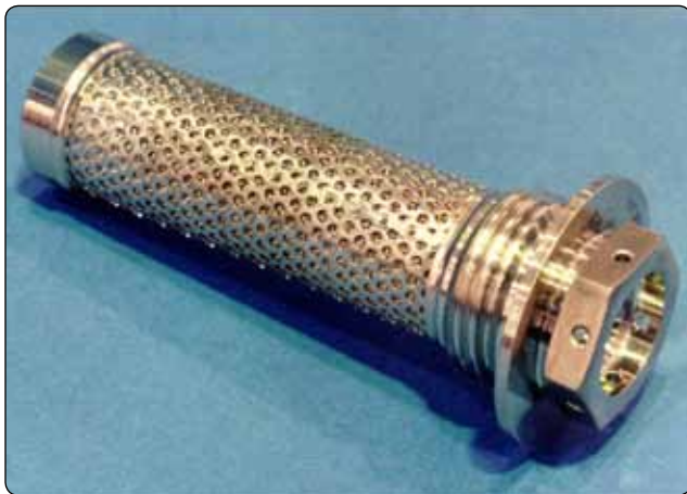
Figure 6-36. Last-chance filter before spray nozzle.
