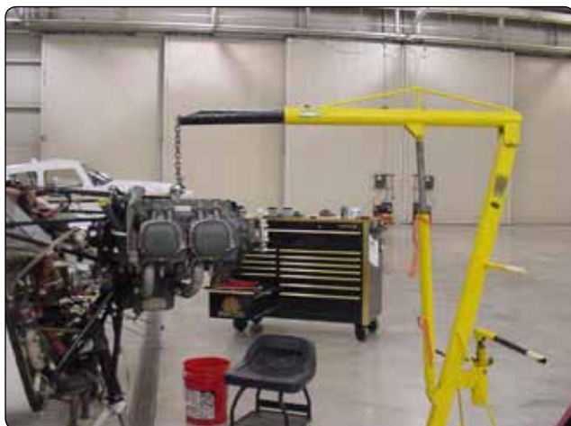
Figure 8-14. Relieve tension on engine mounts.
