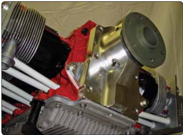
Figure 11-19. Front-end bearing on the 1000 IFB engine.
