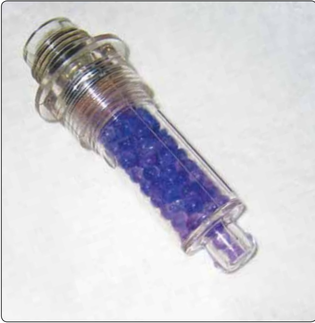
Figure 8-28. Dehydrator plug “blue” showing low humidity (Sacramento Sky Ranch).
