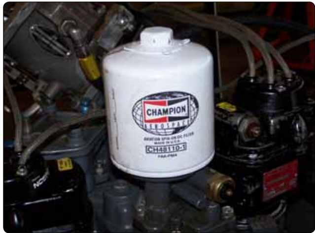
Figure 6-8. Full flow spin-on filter.
