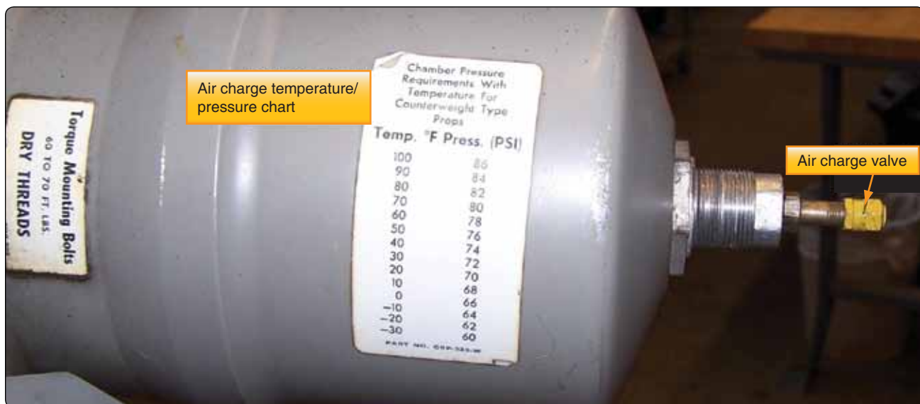
Figure 7-41. Servicing air charge in propeller.
