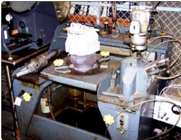
Figure 10-16. Valve seat grinding equipment.
