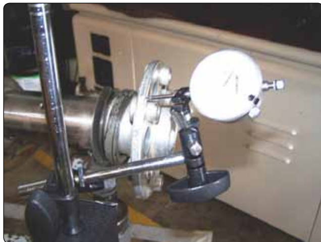
Figure 10-10. Checking crankshaft runout.
