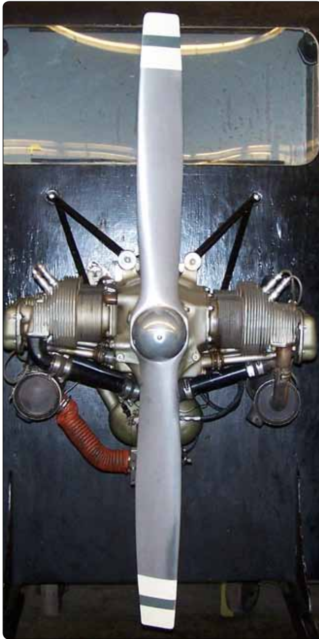
Figure 7-11. Fixed-pitch propeller.
