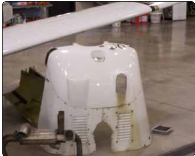
Figure 8-13. Cowling removed and stored out of the way.
