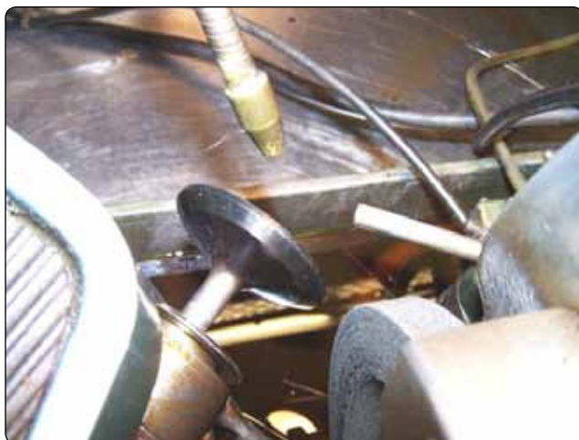
Figure 10-25. Valve in chuck ready to grind.
