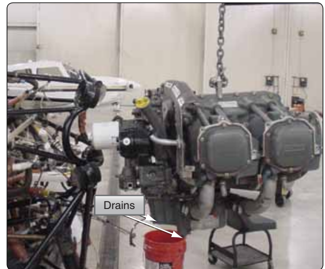
Figure 8-4. Oil system drain points.
