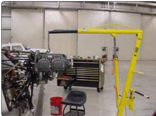
Figure 8-14. Relieve tension on engine mounts.
