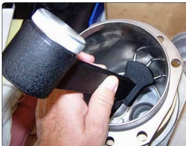
Figure 10-5. A cylinder bore gauge.
