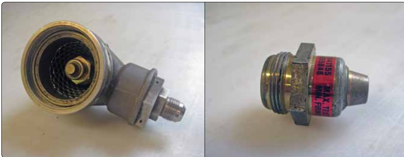
Figure 9-10. Discharge valve and cartridge (squib).
