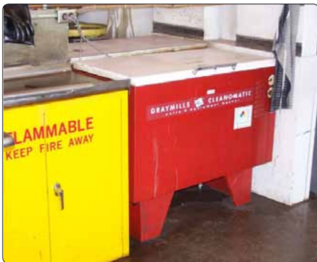
Figure 10-3. Typical solvent degreasing tank.
