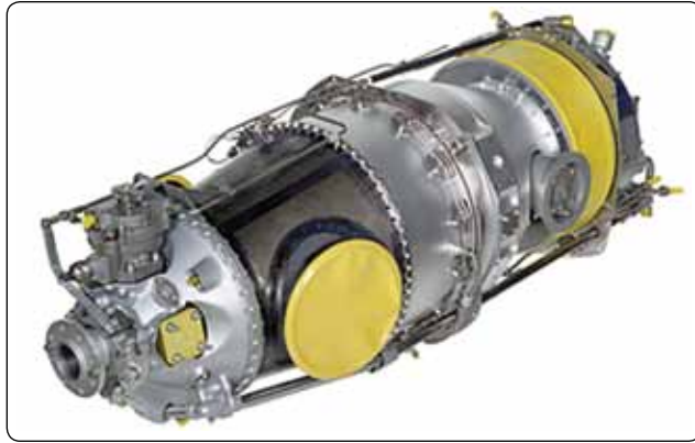
Figure 7-44. Pratt & Whitney PT6 engine.
