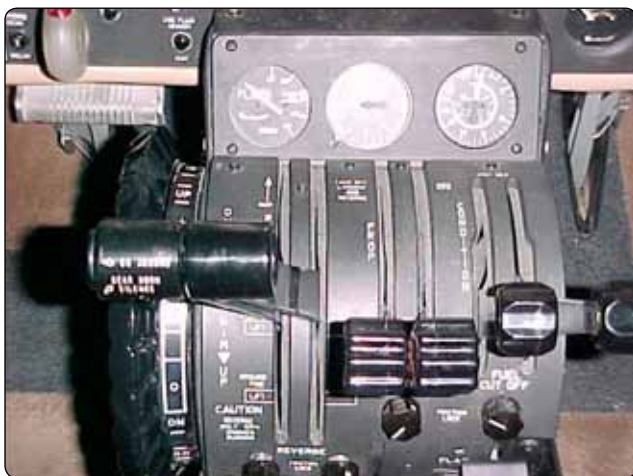
Figure 7-10. Turboprop propeller controls.
