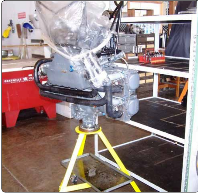
Figure 10-1. Engine mounted on an overhaul stand.
