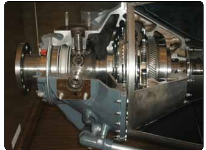
Figure 7-46. Reduction gearbox.
