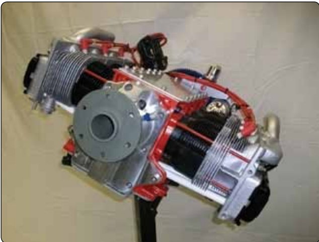
Figure 11-18. Aeromax direct drive, air-cooled, six-cylinder engine.
