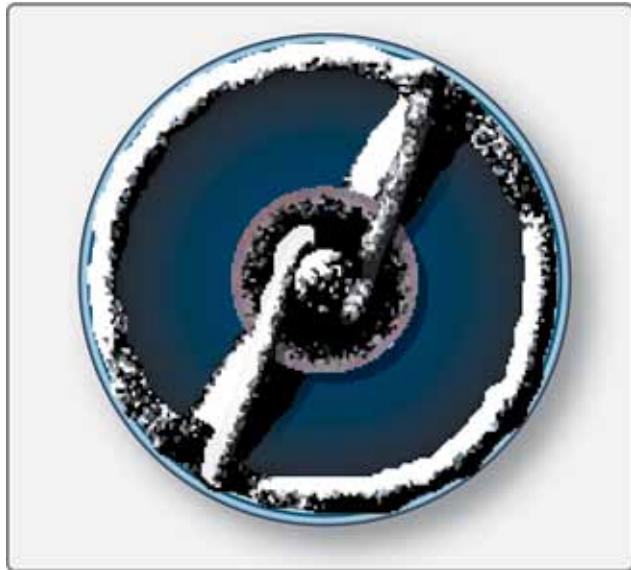
Figure 4-48. Carbon fouled spark plug.
