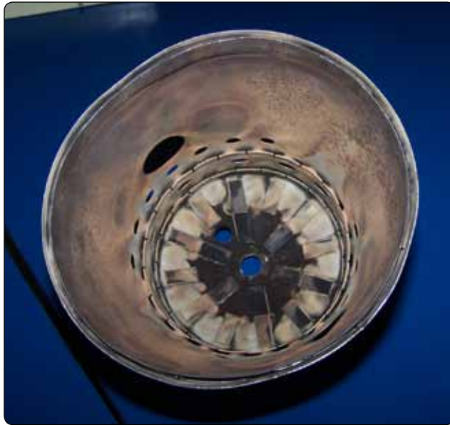
Figure 1-53. Inside view of a combustion chamber liner.
