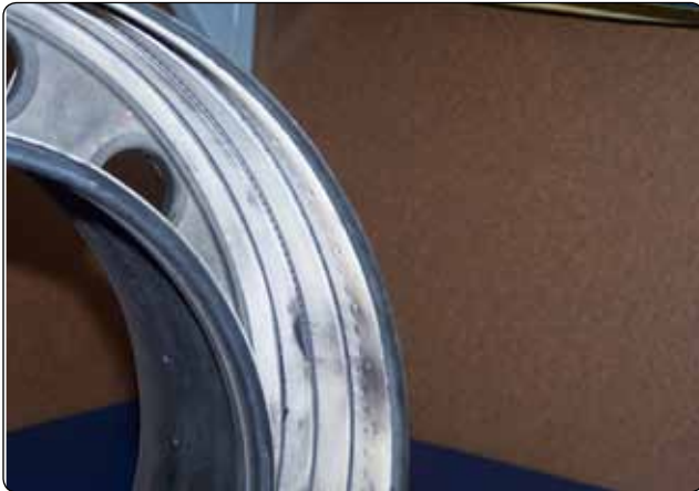
Figure 1-55. Annular combustion chamber liner.
