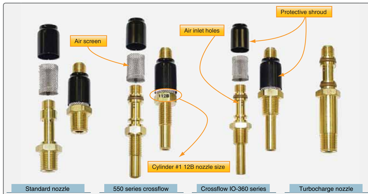
Figure 2-45. Fuel discharge nozzles.
