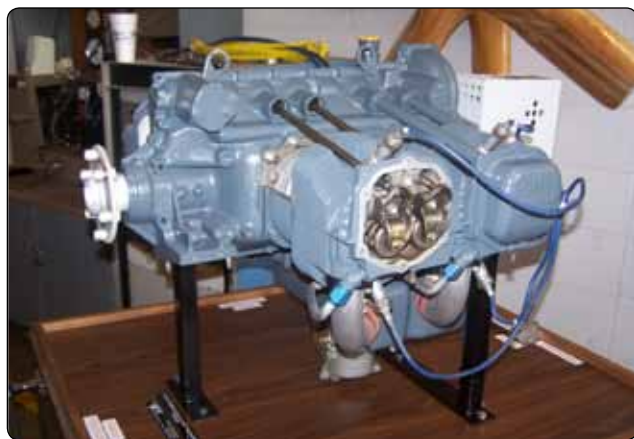
Figure 1-1. A typical four-cylinder opposed engine.
