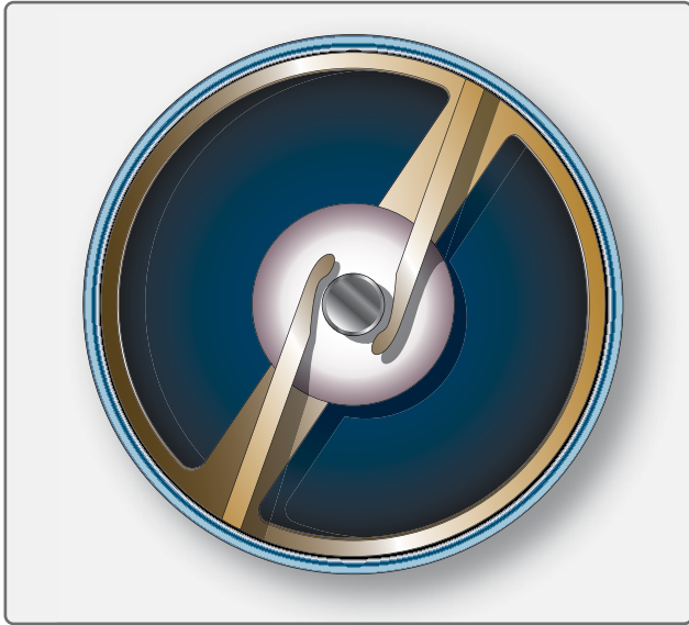
Figure 4-50. Spark plug gap erosion.
