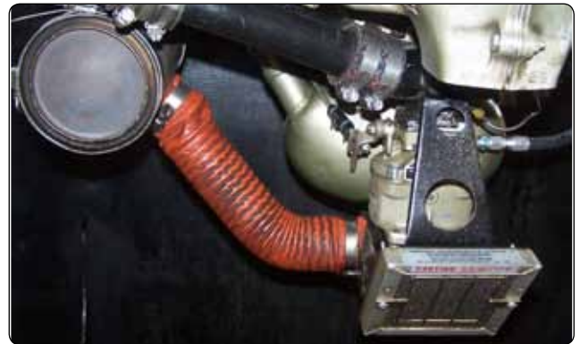
Figure 3-5. Location of a carburetor heat air valve.
