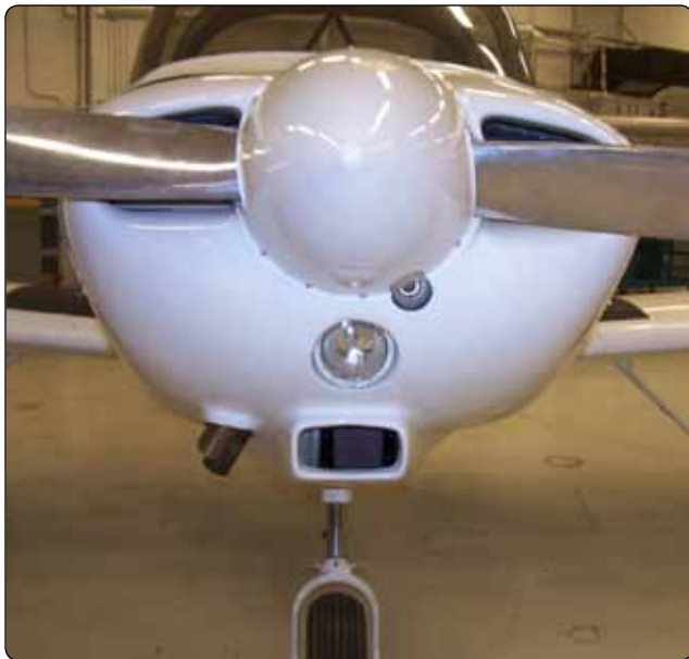
Figure 3-1. Inlet scoop in engine cowling.
