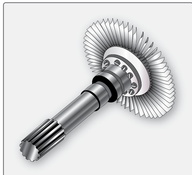
Figure 1-63. Rotor elements of the turbine assembly.
