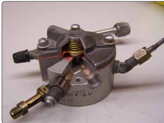
Figure 2-37. Flow divider cutaway.
