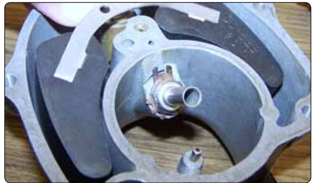
Figure 2-9. Float chamber discharge nozzle and float.
