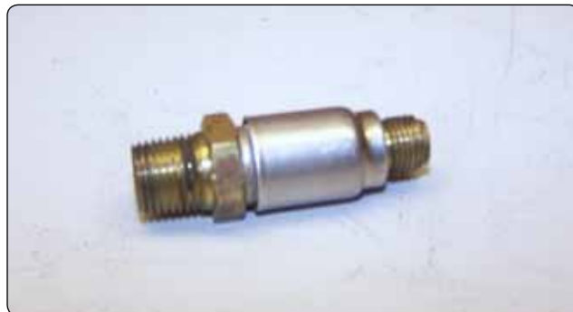
Figure 2-38. Fuel nozzle assembly.
