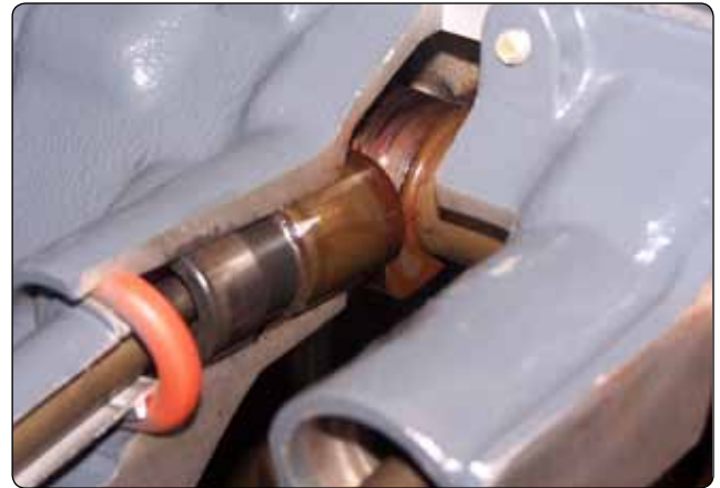
Figure 1-29. Cam load on lifter body.
