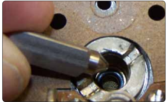
Figure 2-8. Needle valve and seat.
