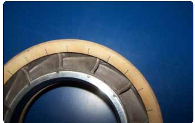
Figure 1-60. Turbine inlet guide vanes.
