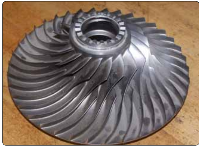
Figure 1-47. Single-entry impeller.
