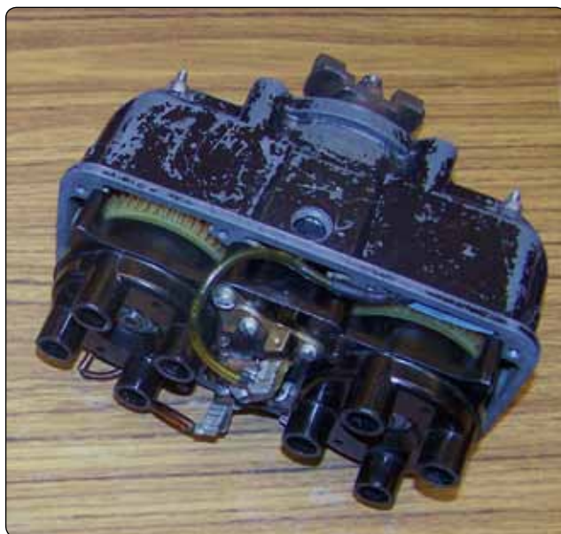
Figure 4-18. A dual magneto with two distributors.
