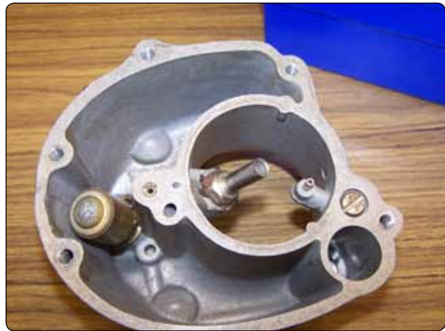
Figure 2-11. Float chamber (bowl) with float removed.
