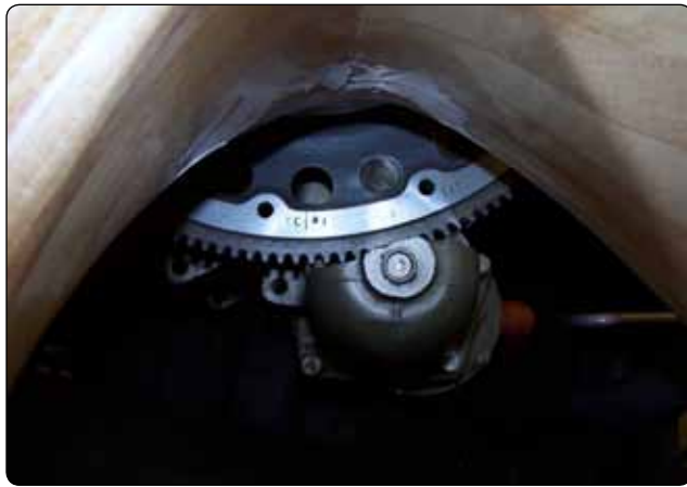
Figure 4-46. Timing marks aligned.
