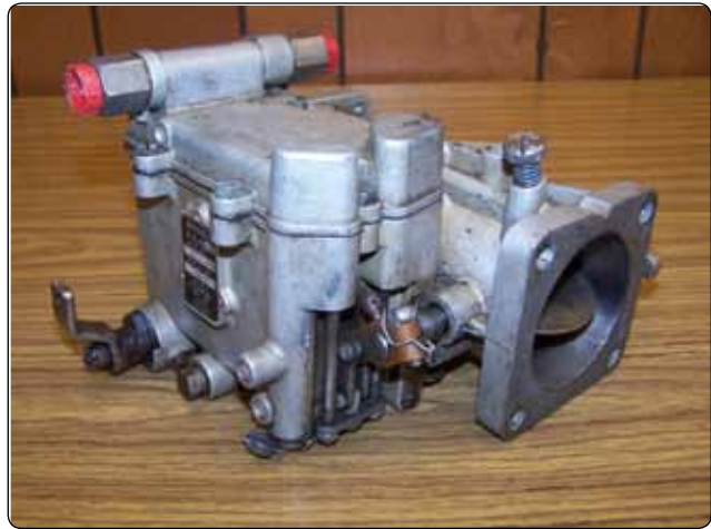
Figure 2-5. Side draft horizontal flow carburetor.
