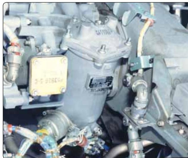
Figure 2-60. Dual element fuel pump.
