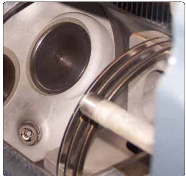
Figure 1-15. Machined rings around a piston.
