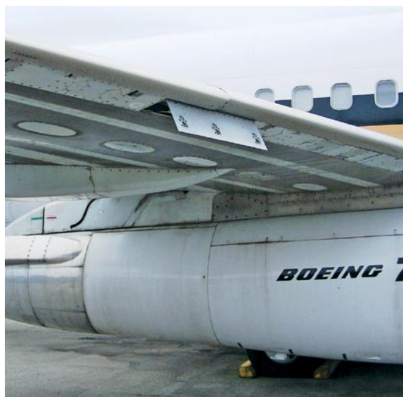
Figure 11-32. Single point refueling station of a large aircraft.
