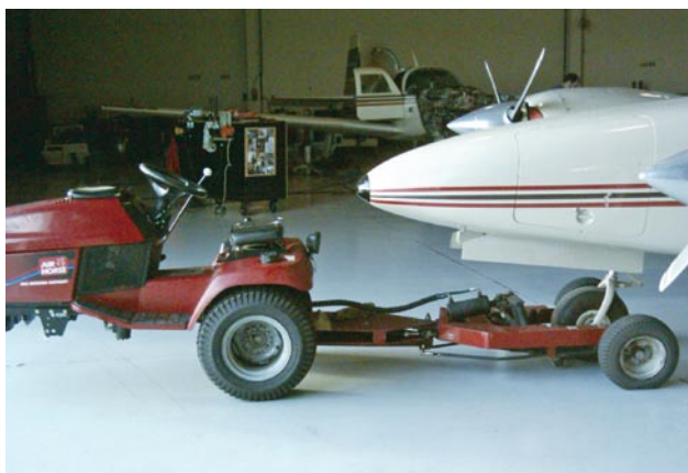
Figure 11-21. Typical smaller aircraft tow tractor.
