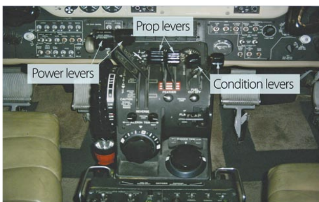
Figure 11-16. Engine controls of a turboprop aircraft.
