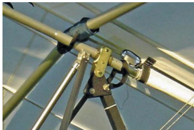
Figure 4-38. Wing attach point for a weight-shift aircraft.
