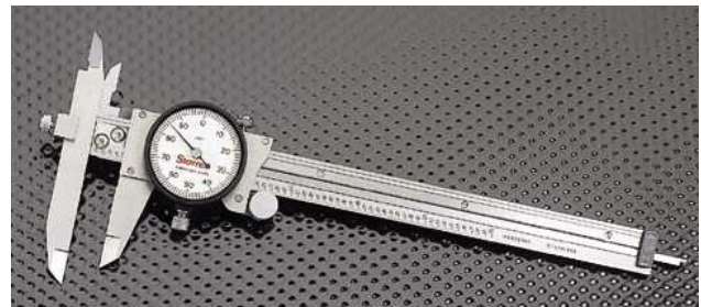
Figure 9-41. Electronic and dial indicator slide calipers.
