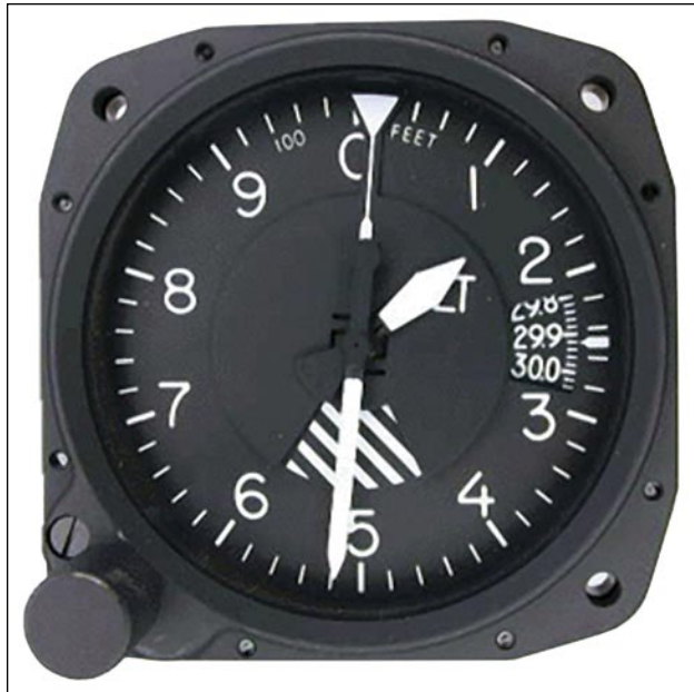
Figure 3-51. An airplane's altimeter is an aneroid barometer.
