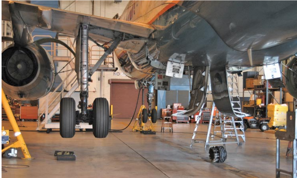
Figure 3-4. Airbus A-320 being jacked.
