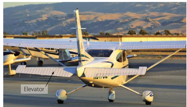
Figure 3-65. Elevator on a Cessna 182 provides pitch control.
