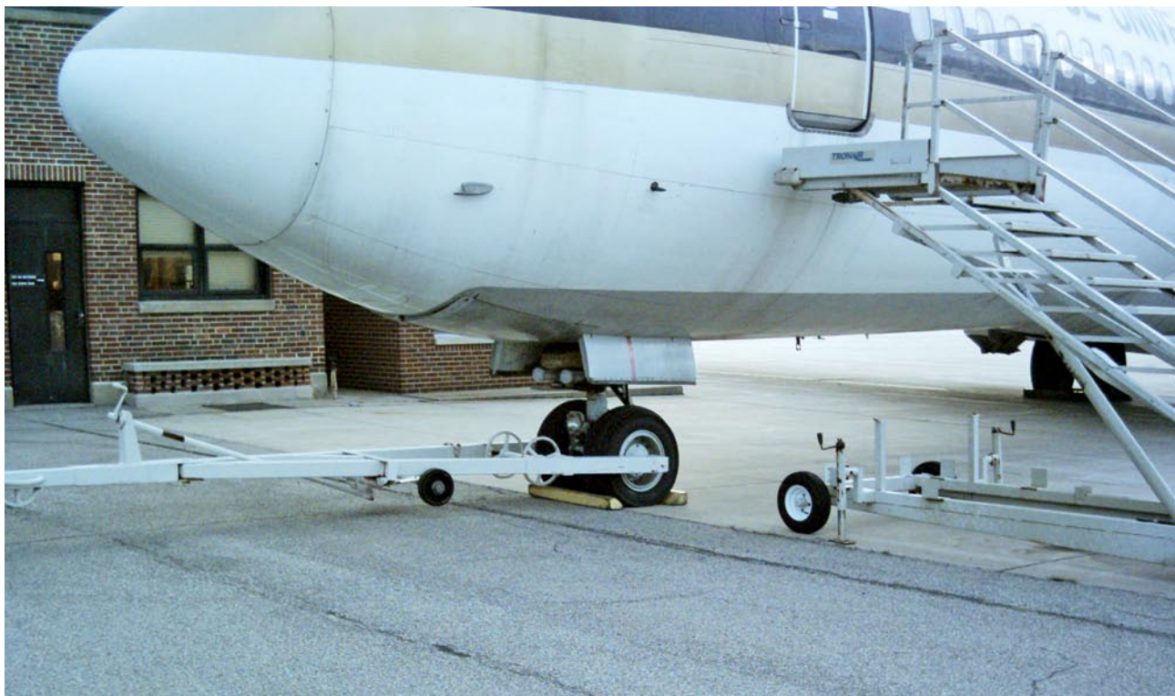
Figure 11-20. Tow bar for a large aircraft.
