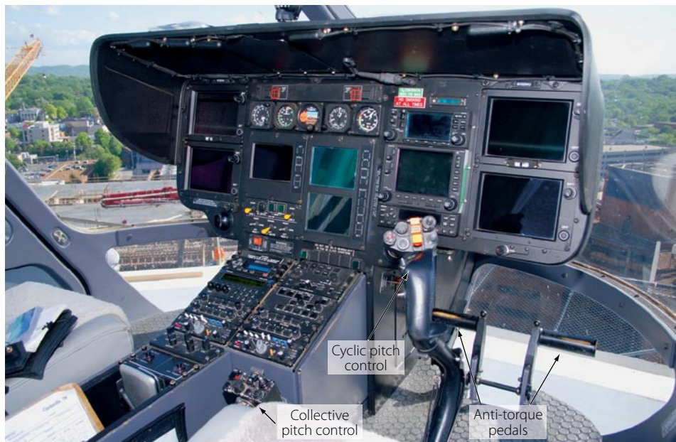
Figure 3-91. Helicopter cockpit controls.
