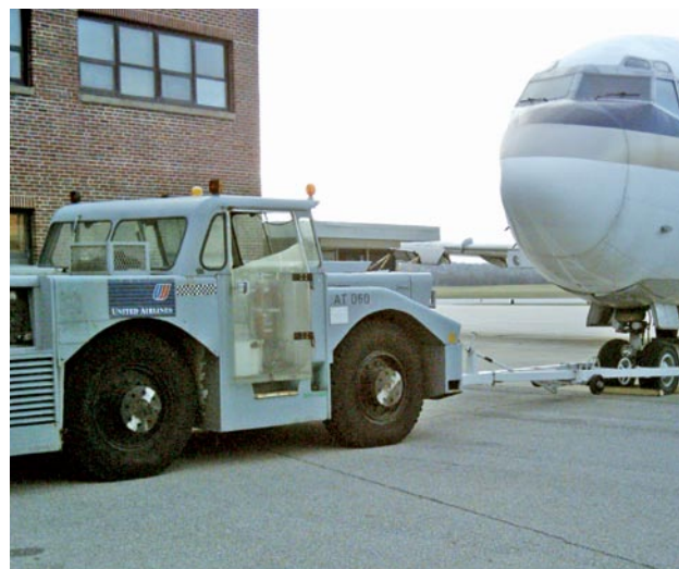
Figure 11-19. Example of a tow tractor.
