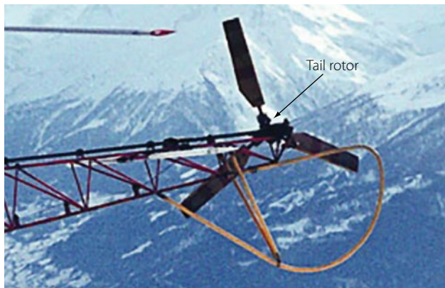
Figure 3-86. Aerospatiale helicopter tail rotor.
