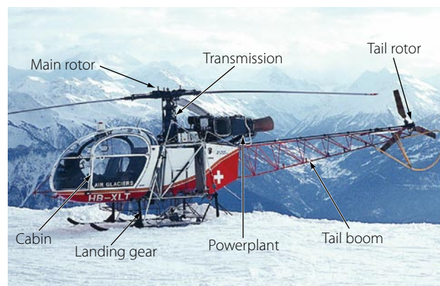
Figure 3-81. Main components of a helicopter.
