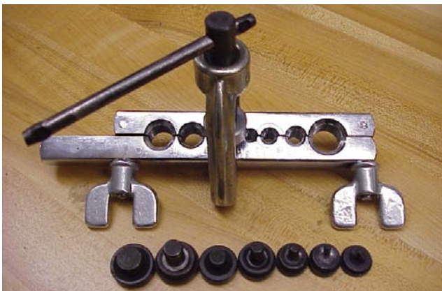
Figure 7-10. Double flare tool.
