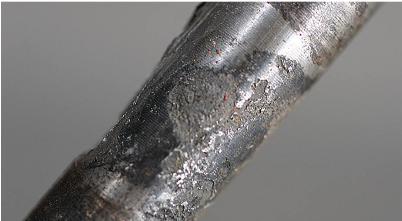
Figure 6-7. Dissimilar metal corrosion.
