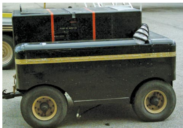
Figure 11-30. A portable compressed air cart.
