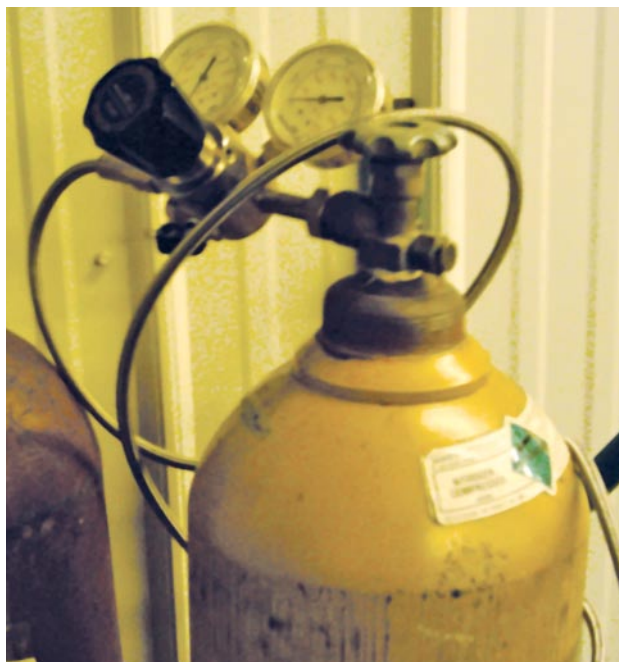
Figure 11-1. A typical nitrogen bottle.
