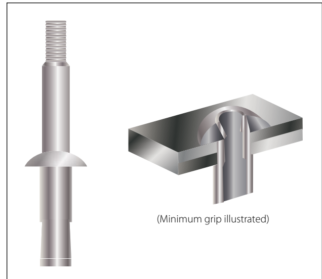
Figure 5-44. Wiredraw cherrylock rivet.
