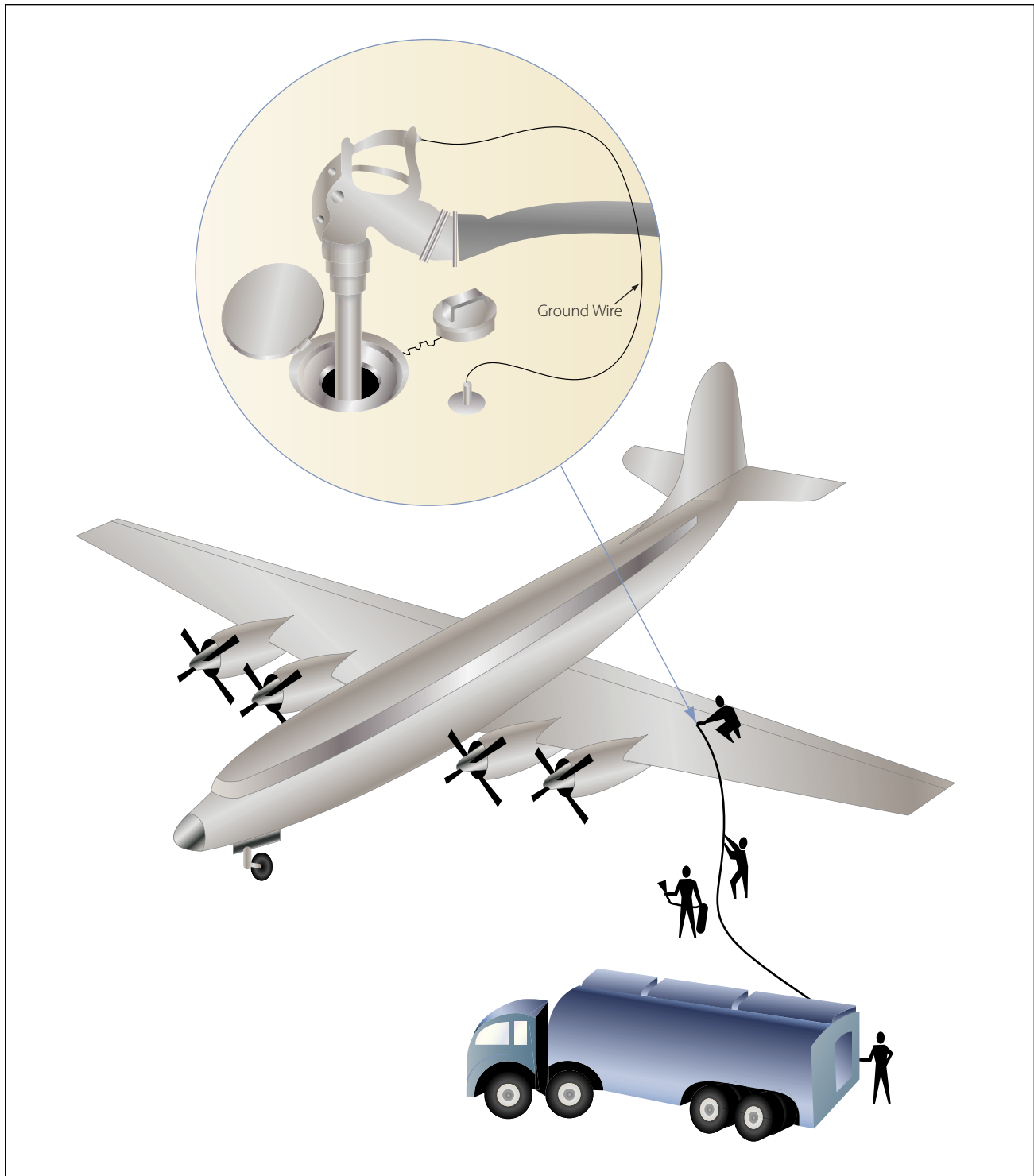
Figure 11-31. Refueling an aircraft by the over-the-wing method.
