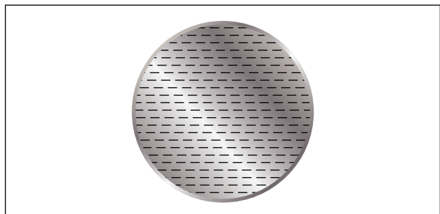
Figure 10-10. Even distribution of charge on metal disk.
