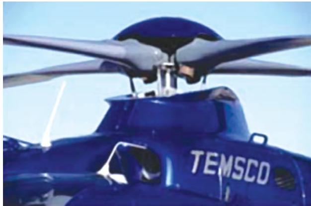
Figure 3-85. Eurocopter Model 135 rigid rotor system.
