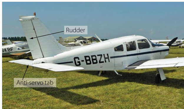
Figure 3-70. Rudder on a Piper Cherokee Arrow.
