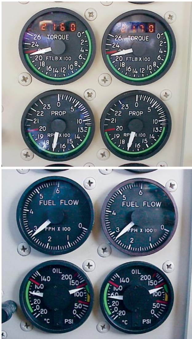
Figure 11-15. Typical examples of turboprop instruments.
