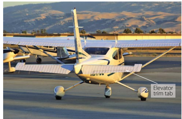
Figure 3-71. Elevator trim tab on a Cessna 182.
