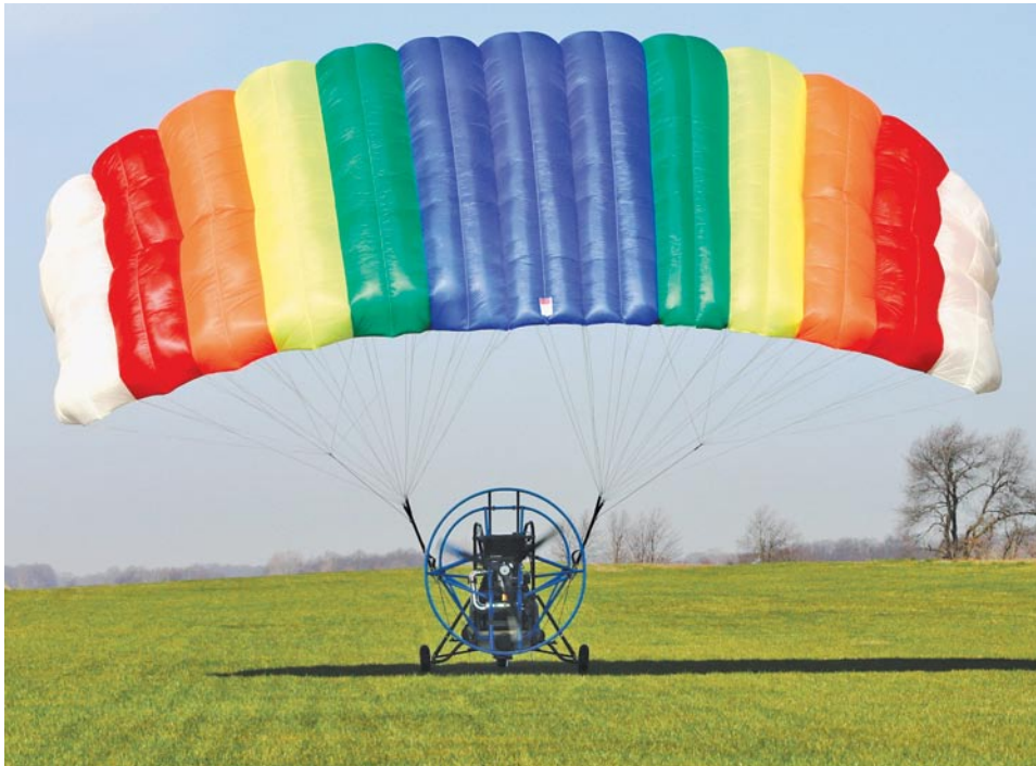
Figure 3-104. Powered parachute wing trailing edge.
