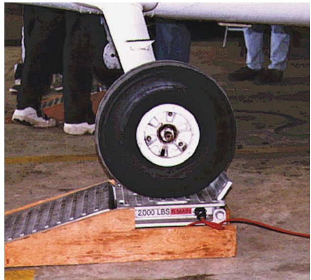
Figure 3-17. Ramp in use with a Cessna 172.
