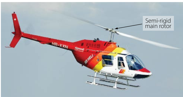
Figure 3-84. Bell Jet Ranger with semi-rigid main rotor.
