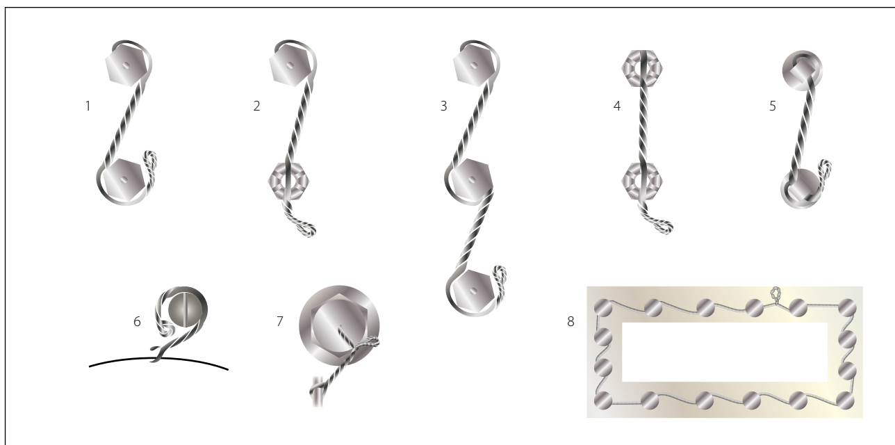
Figure 5-71. Safety wiring methods.
