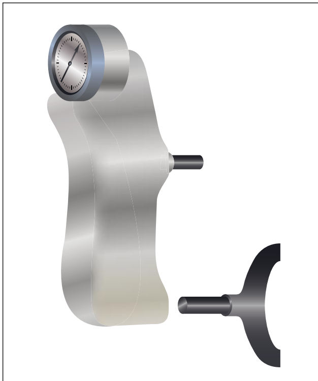
Figure 5-12. Barcol portable hardness tester.
