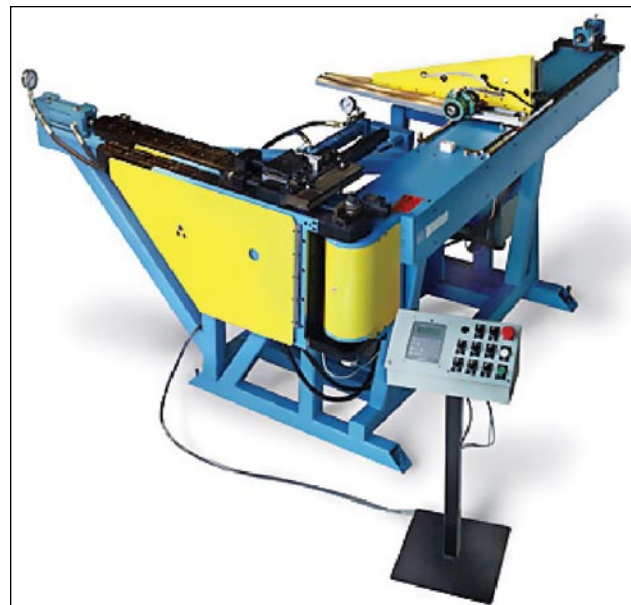
Figure 7-6. CNC tube bending machine.
