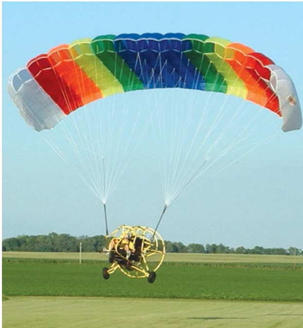
Figure 3-102. Powered parachute with the wing inflated.
