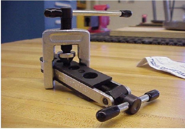
Figure 7-9. Hand flaring tool.
