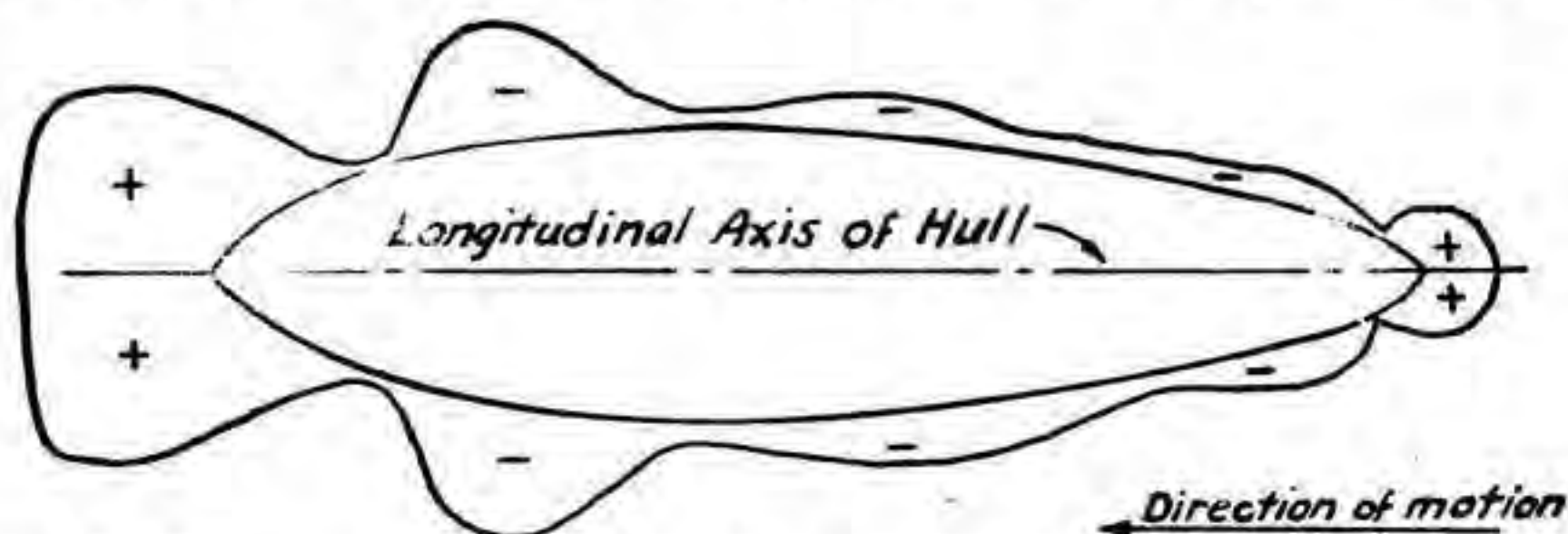
FIGURE 16.—Pressure distribution on airship hull (longitudinal axis parallel to direction of motion).
