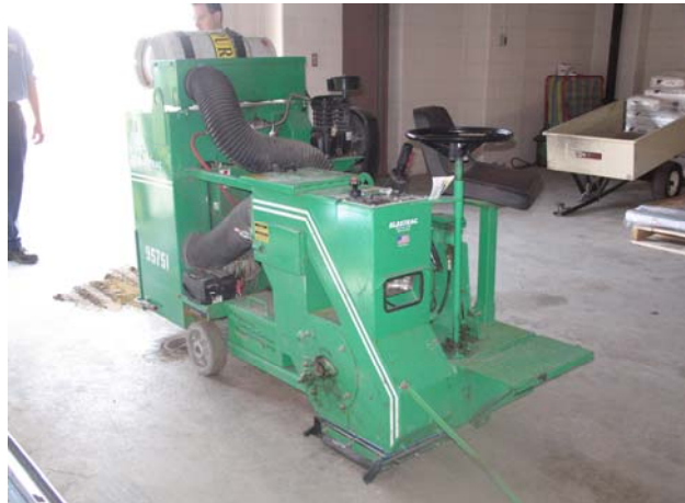
FIGURE 5-13. SHOTBLASTER WITH A 10-INCH CUT.
