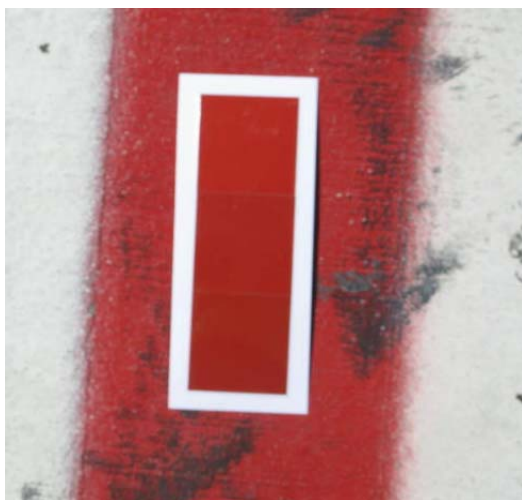
FIGURE 6-72. RED COLOR CHIP COMPARED TO RED MARKING.
