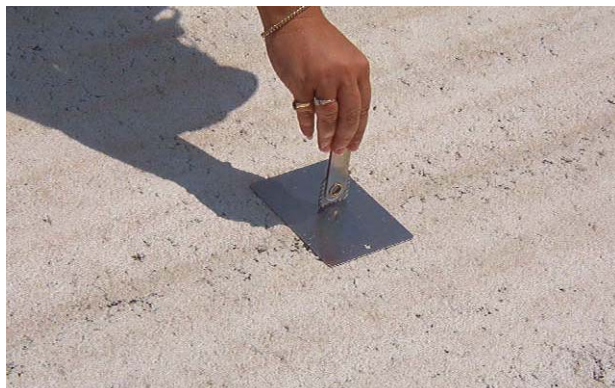
FIGURE 6-67. WET FILM GAUGE ON A METAL COUPON.
