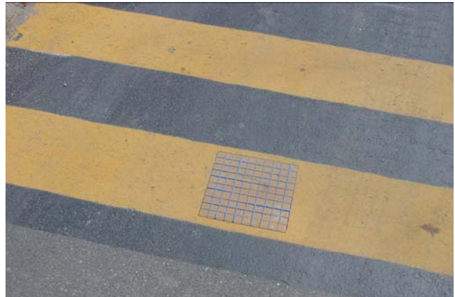
FIGURE 6-74. GRID FOR COMPLIANCE WITH DEGREE OF PAINT REMOVAL.
