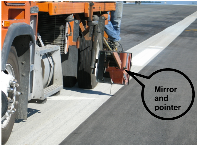
FIGURE 6-55. POINTER WITH MIRROR.
