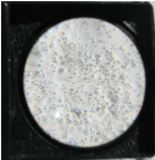
FIGURE 3-4. POOR TYPE I BEAD DISTRIBUTION; READINGS AVERAGED ONLY 135 mcd/m 2 /lux.
