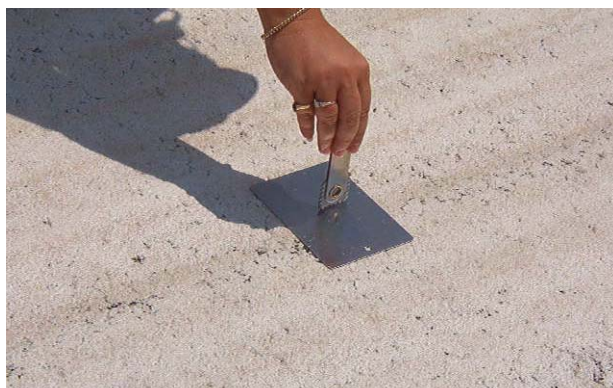
FIGURE 6-67. WET FILM GAUGE ON A METAL COUPON.
