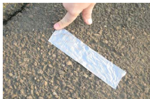
FIGURE 6-68. USE DUCT TAPE TO MEASURE WET FILM THICKNESS OF MARKING.
