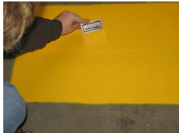
FIGURE 6-62. USE OF WET FILM GAUGE.
