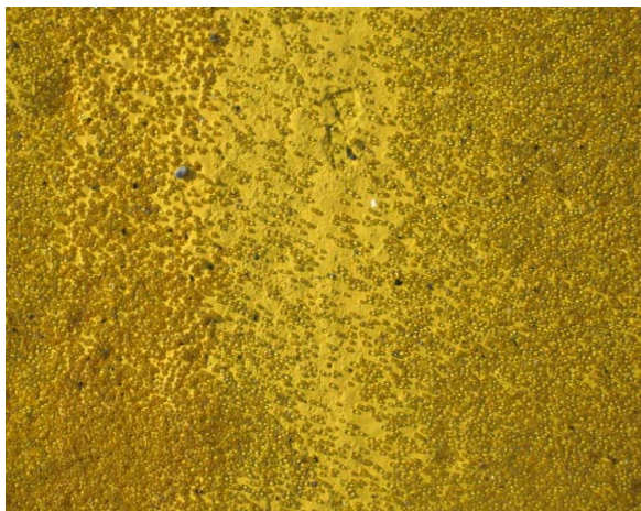
FIGURE 3-10. TYPE IV BEAD DISTRIBUTION IS EXCELLENT ON BOTH EDGES, BUT POOR IN THE MIDDLE.
