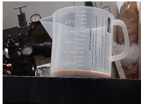
FIGURE 6-59. CALIBRATION BUCKET FOR GLASS BEADS.
