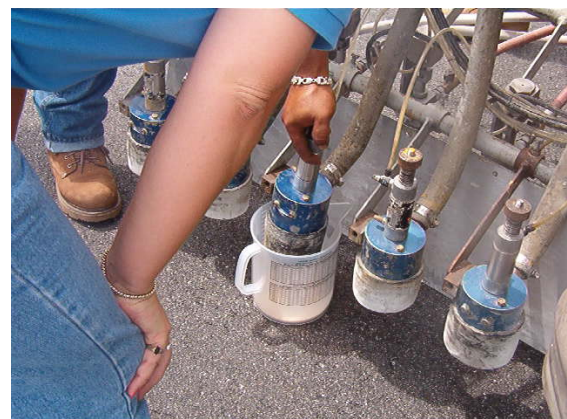
FIGURE 6-60. CALIBRATION OF GLASS BEAD GUNS.
