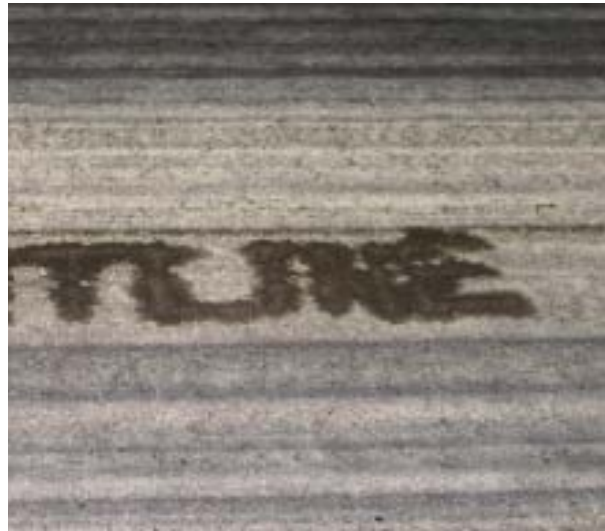
FIGURE 4-31. RUST REMOVER DAMAGED GLASS BEADS, MAKING THEM INEFFECTIVE.
