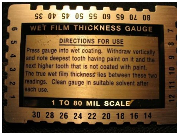
FIGURE 6-61. WET FILM GAUGE.
