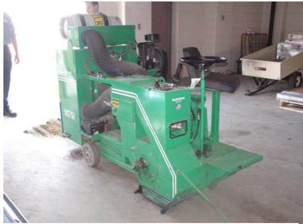
FIGURE 5-13. SHOTBLASTER WITH A 10-INCH CUT.
