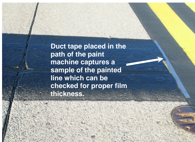
FIGURE 6-68. USE DUCT TAPE TO MEASURE WET FILM THICKNESS OF MARKING.
