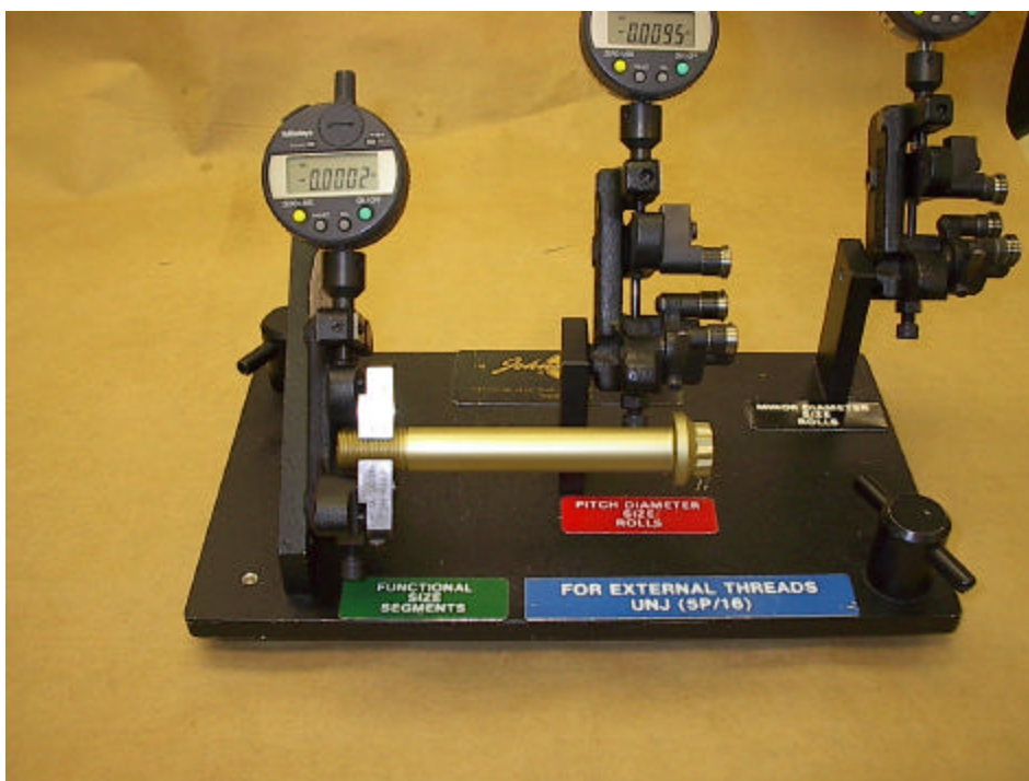
Figure 11 INSPECTION FOR FUNCTIONAL DIAMETER SIZE, FULL FORM SEGMENT INDICATING GAGE
