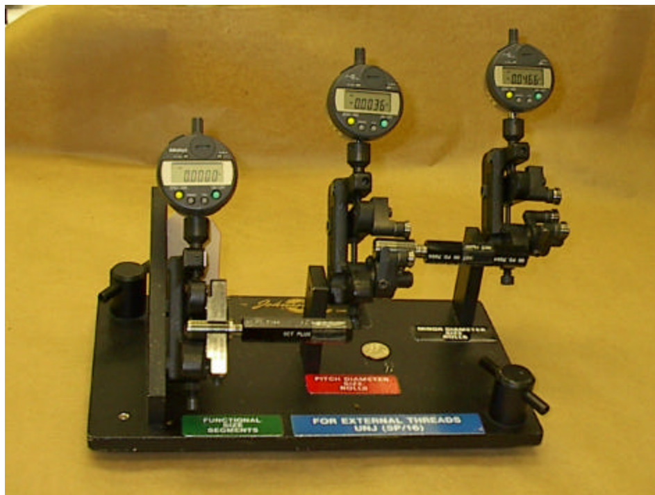
Figure 14 INSPECTION OF FAA GAGES, THREADED “W” TOLERANCE SET PLUG GAGES
