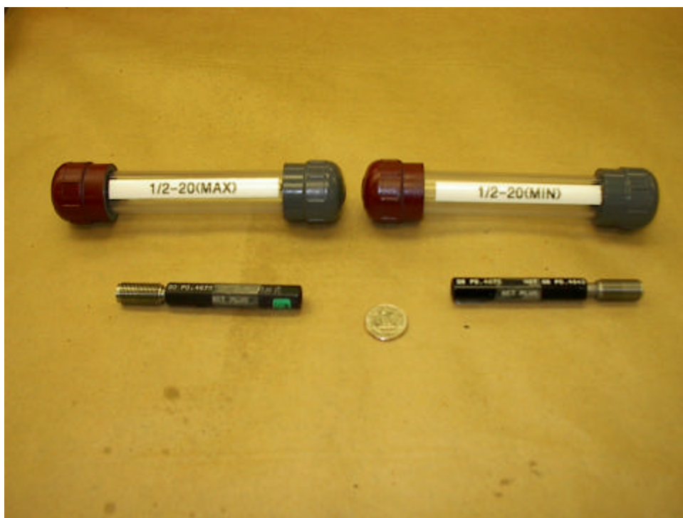
Figure 9 FAA GAGES, THREADED "W" TOLERANCE SET PLUG GAGES
