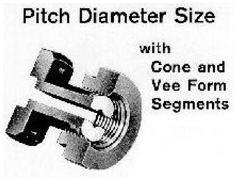
Figure 19 INSPECTION FOR PITCH DIAMETER SIZE ON INTERNAL THREADS, CONE & VEE FORM SEGMENTS
