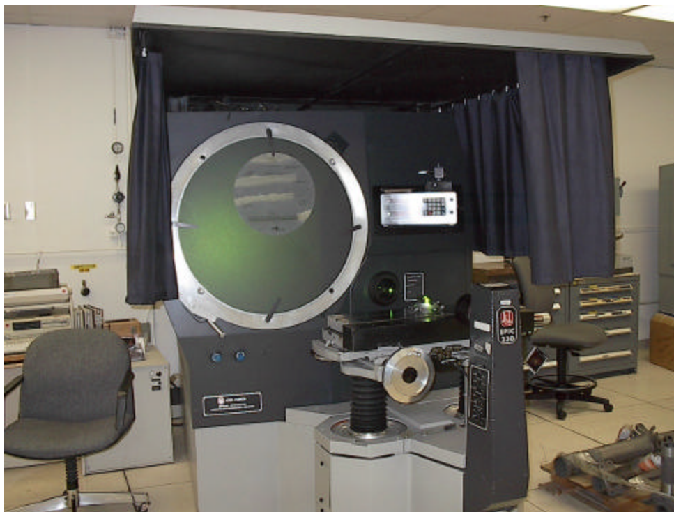
Figure 8 FAA GAGES, OPTICAL COMPARATOR WITH OVERLAY CHART
