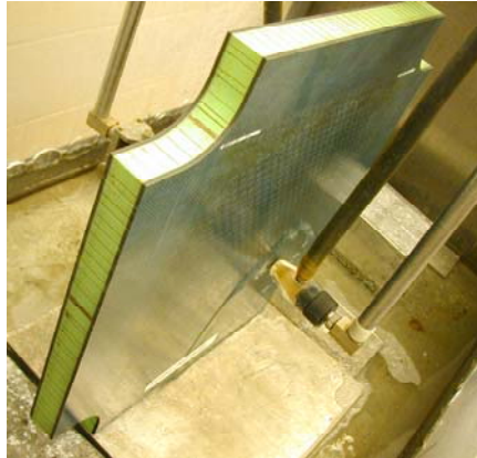
FIGURE 7. WICHITA STATE UNIVERSITY ULTRAPAC SCANNER (C-SCAN)
