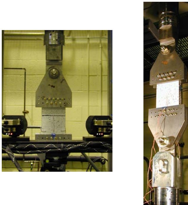
FIGURE 31. UNIDIRECTIONAL TENSION COUPON TEST SETUP
