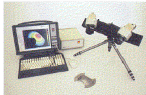
FIGURE 21. ARAMIS HR SETUP
