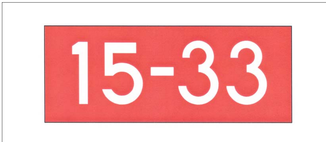
FIG 2-3-24 Runway Holding Position Sign
