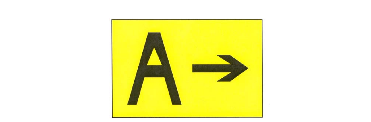
FIG 2-3-36 Direction Sign for Runway Exit
