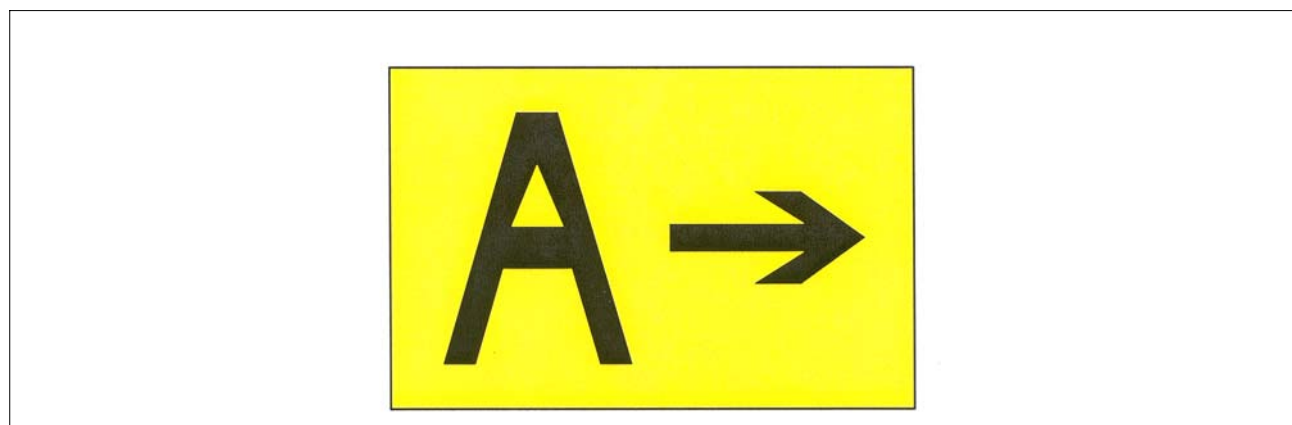
FIG 2-3-36 Direction Sign for Runway Exit
