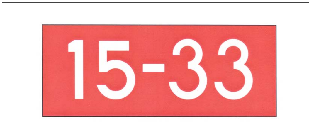
FIG 2-3-24 Runway Holding Position Sign
