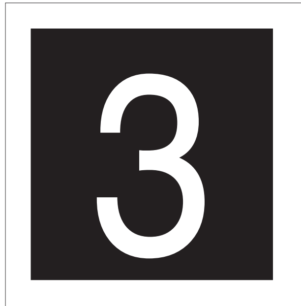
FIG 2-3-41 Runway Distance Remaining Sign Indicating 3,000 feet of Runway Remaining
