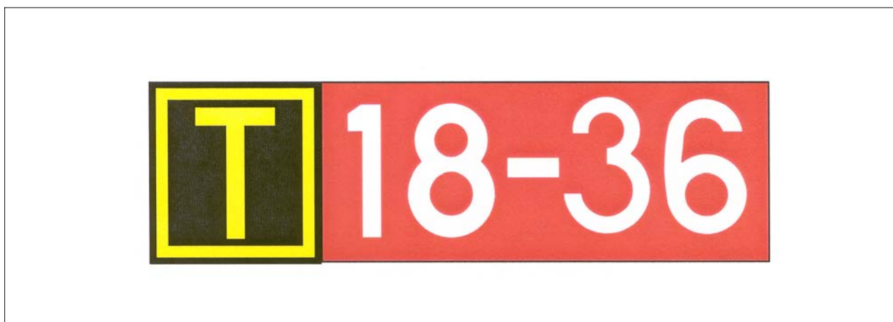
FIG 2-3-31 Taxiway Location Sign Collocated with Runway Holding Position Sign
