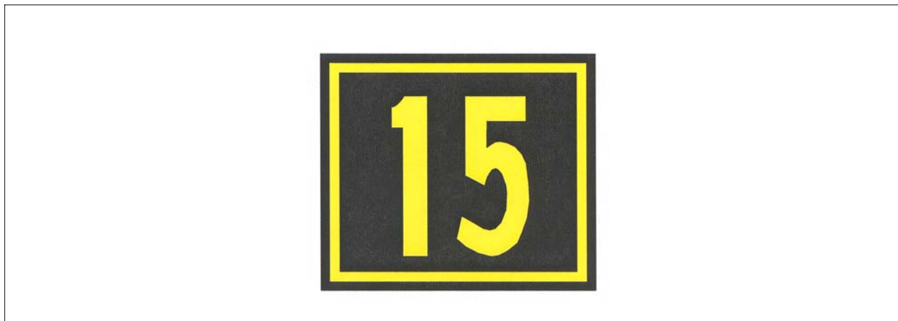
FIG 2-3-32 Runway Location Sign
