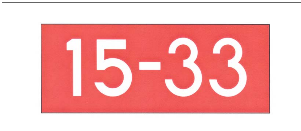
FIG 2-3-24 Runway Holding Position Sign
