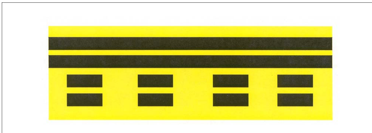
FIG 2-3-33 Runway Boundary Sign
