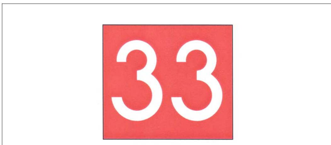
FIG 2-3-25 Holding Position Sign at Beginning of Takeoff Runway
