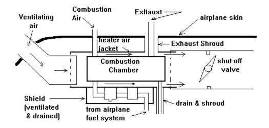
1 The shut-off valve shown in the sketch should be provided if there are fuel system components within the ventilating air shroud which may be subject to leakage or failure. In such cases, that portion of the ventilating air duct up to the valve, as well as the valve itself, should be of fire resistant construction and the valve should provide as flame tight a seal as possible. If the fuel system is so arranged that there are no fittings or connections within the
