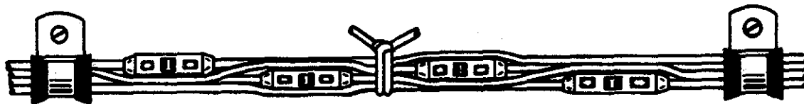
FIGURE 11-14. Staggered splices in a wire bundle.
