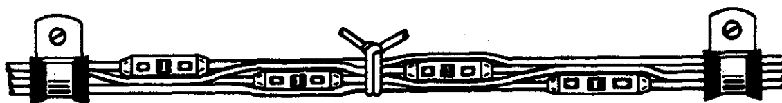
FIGURE 11-14. Staggered splices in a wire bundle.
