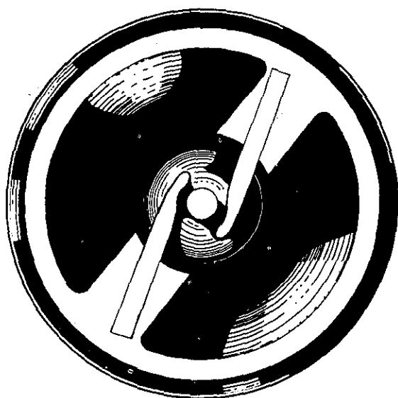
FIGURE 4-54. Spark plug gap erosion.
