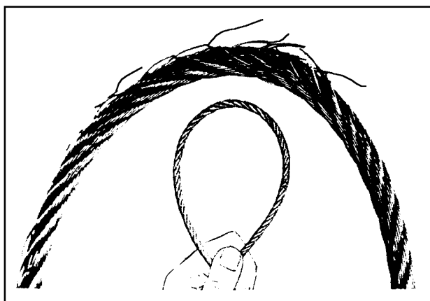
FIGURE 7-16. Cable inspection technique.
