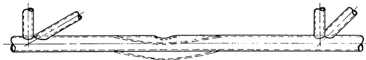
DENTED OR BENT TUBE
