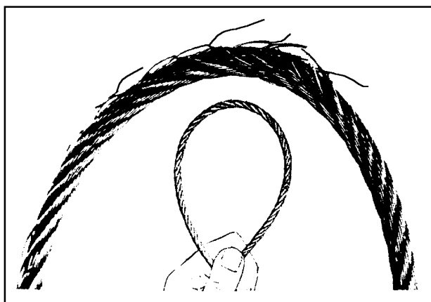
FIGURE 7-16. Cable inspection technique.
