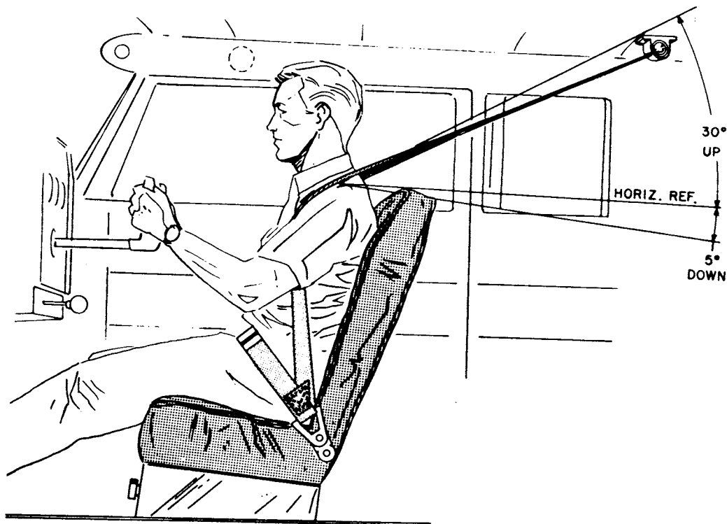
FIGURE 9.6.—Ceiling mounted inertia reel—double over-the-shoulder type harness.
