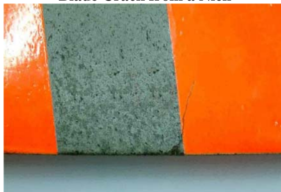
FIGURE 1-9. Blade Crack from a Nick
