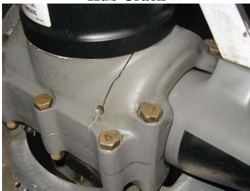
FIGURE 1-8. Hub Crack
