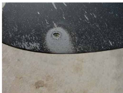
FIGURE 1-12. Lightning Strike on a Composite Surface
