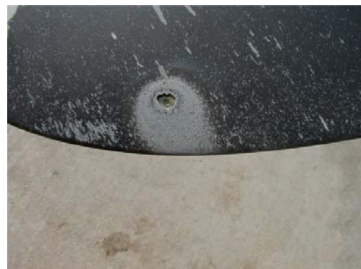
FIGURE 1-12. Lightning Strike on a Composite Surface
