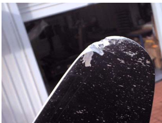
FIGURE 1-13. Propeller Blade Struck by a Foreign Object
