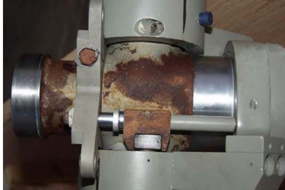
FIGURE 1-1. Hub Surface Corrosion
