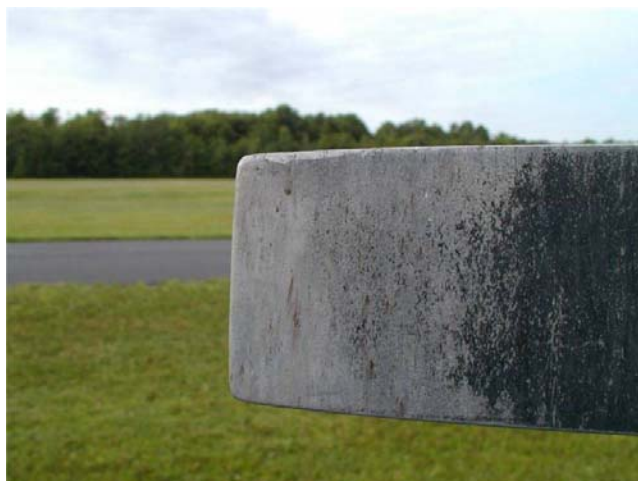
FIGURE 1-7. Erosion on a Metal Blade
