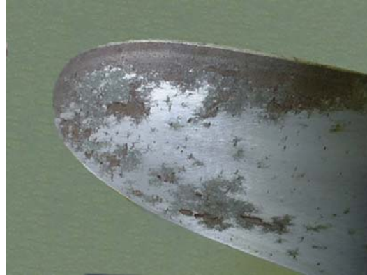
FIGURE 1-2. Polished Blade Surface Corrosion
