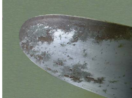
FIGURE 1-2. Polished Blade Surface Corrosion
