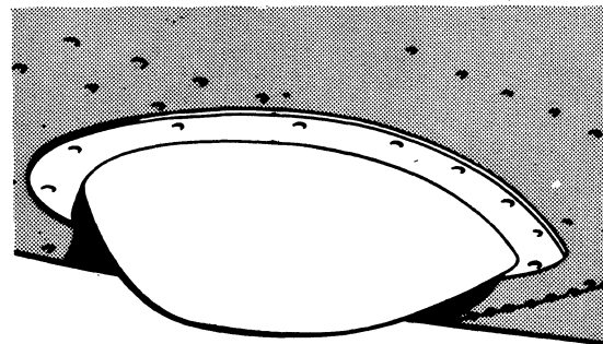
FIGURE 8-8. ADF antenna—fixed loop.
