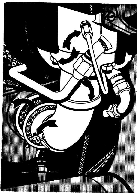
FIGURE 3-6. Intake manifold checkpoints.
