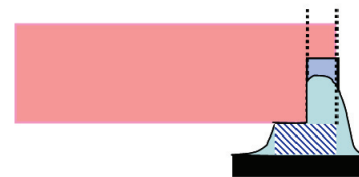
Castellated chip carrier device
