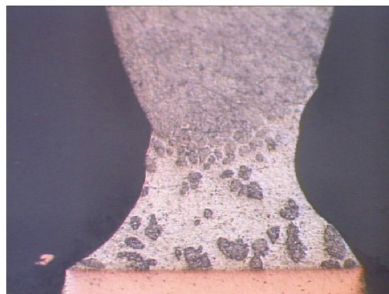
Figure 47: Microsection of CGA mounted on PCB showing minimum solder: Acceptable
