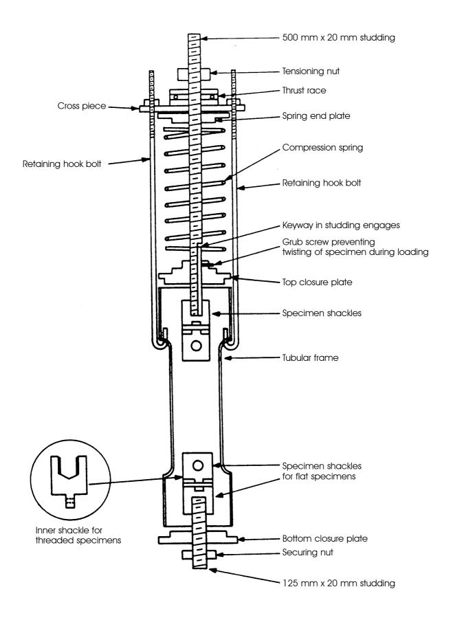
Figure B-1: Cross-section of stress-corrosion jig
