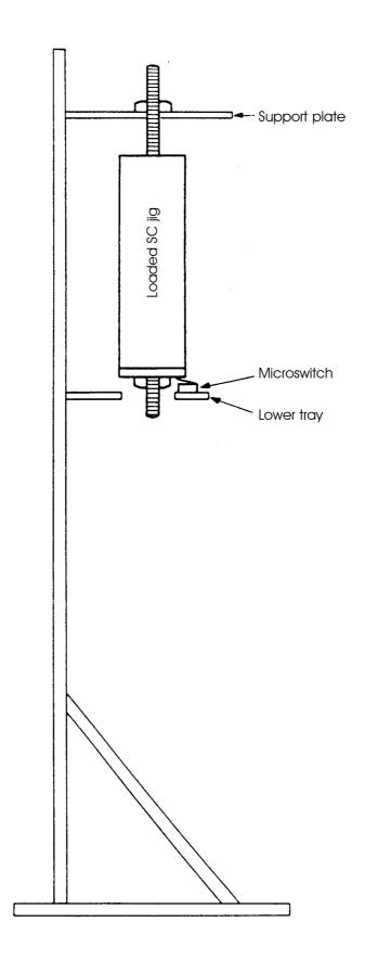
Figure B-2: Support frame for stress-corrosion jig
