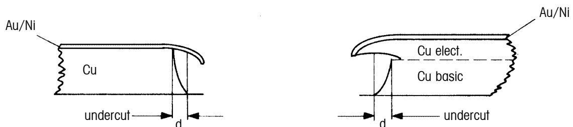
Figure 26: Undercut for PCBs with Au/Ni or Au finish
