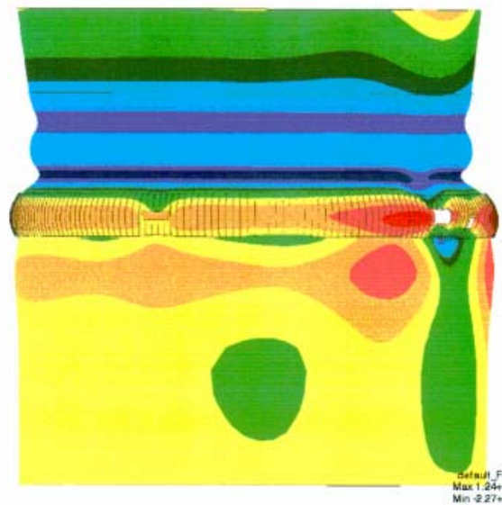
Figure 19-11: Collapse due to LC1 without geometrical imperfection
