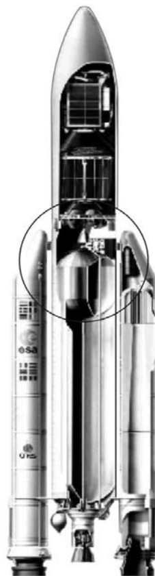
Figure 21-1: Position of the Front Skirt (JAVE) within ARIANE 5 Launcher
