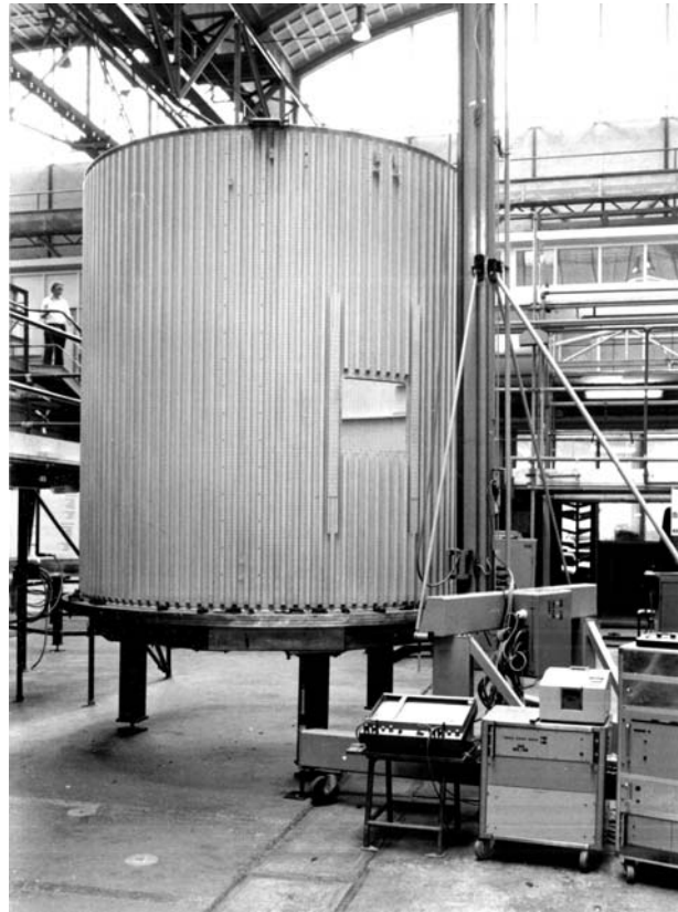
Figure 9-13: Initial imperfection survey system from the TU Delft
