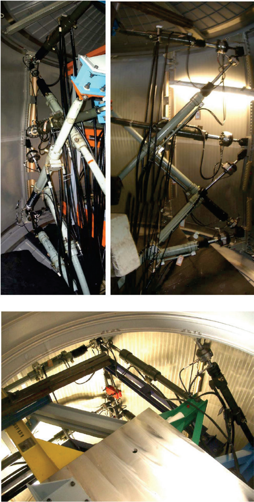
Figure 7-6: ATV static test: internal loading jacks details
