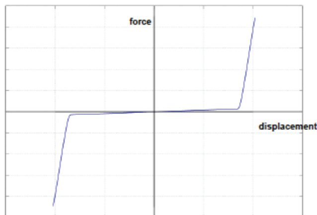
Figure 15-5: Nonlinear stiffness due to mechanical stop
