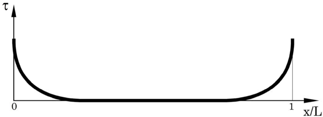
Figure 10.11-8 - Shear stress distribution for large overlap lengths
