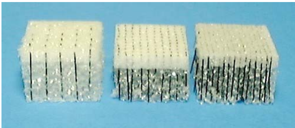
Figure 6.40-1 - Z-Fiber® preforms containing 0.28mm diameter pins at densities of 0.5%, 2% and 4%
