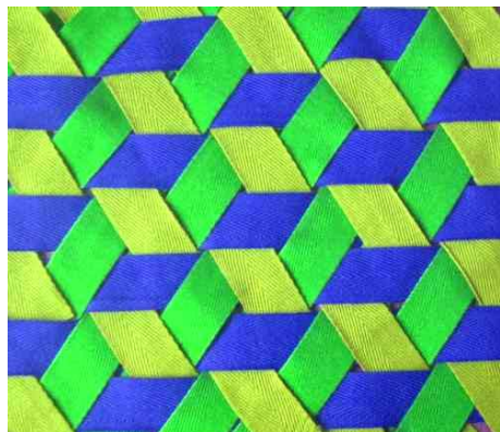
Figure 2.6-1 – Triaxial woven fabric: Weave types
