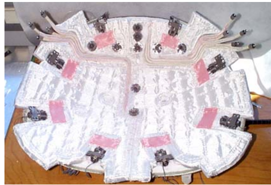
HTI and IFI integration in nose cap area completed
