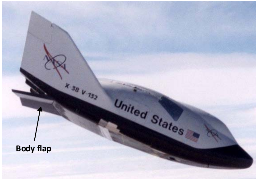
Figure 70.23-1 – X-38: Test vehicle
