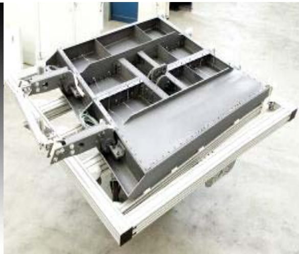
Body flap assembly (4 boxes), using C/SiC fasteners.
