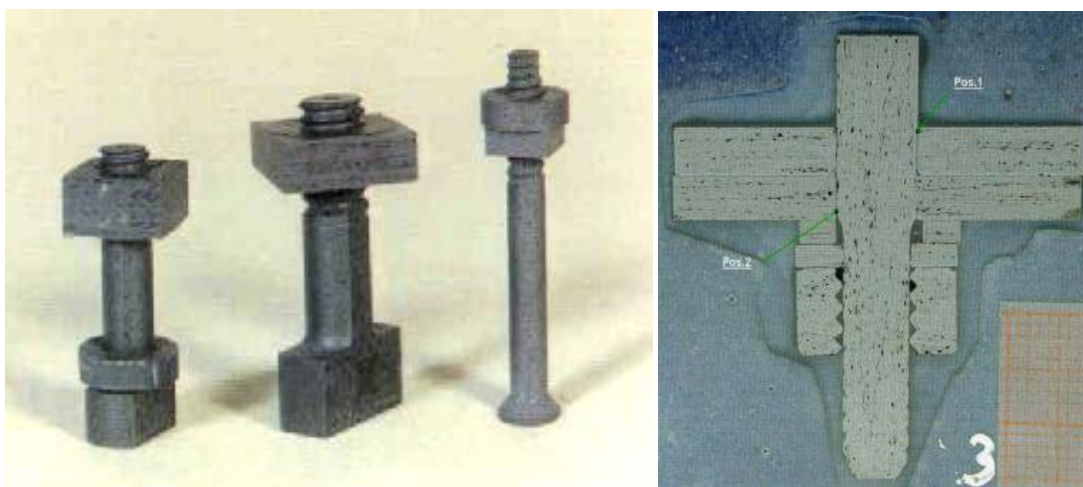
Figure 70.23-3 – X-38 body flap: Mechanical fasteners
