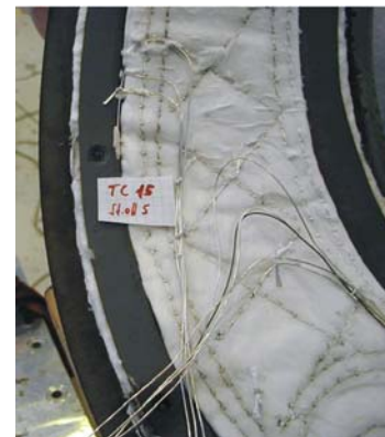
HTI in 'Side Panel' (after qualification test and disassembly)
