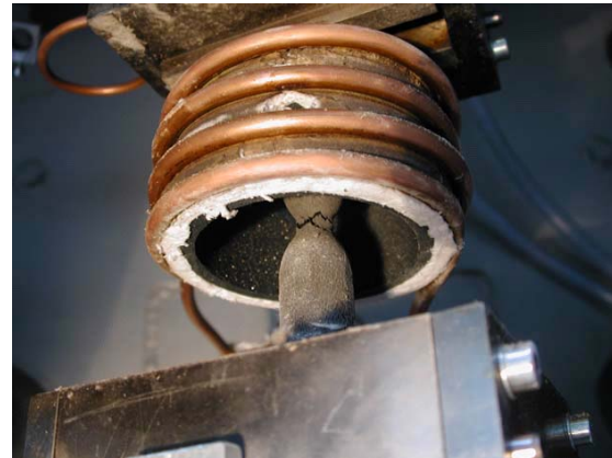
Fractured 'hour-glass' test specimen in high-temperature test rig
