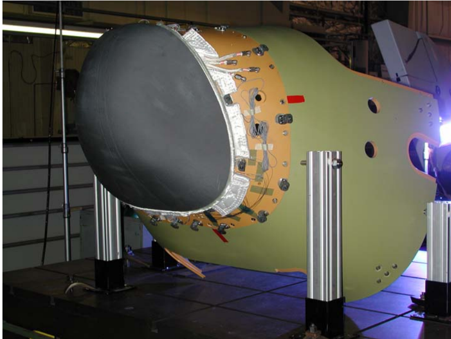
Figure 70.24-5 – X-38 Nose cap with insulation mounted on vehicle nose structure
