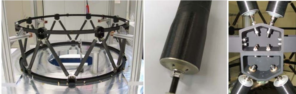
Figure 30.10-5 – ALADIN: IEB middle cylinder (left), CFRP IEB strut end fitting (centre) and typical IEB node (right)
