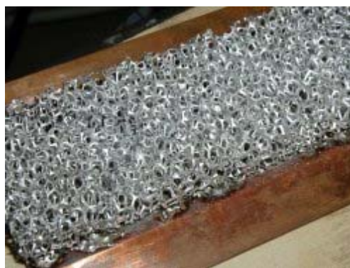
Figure 26.3-5 – Metal foam: Example of aluminium foam
