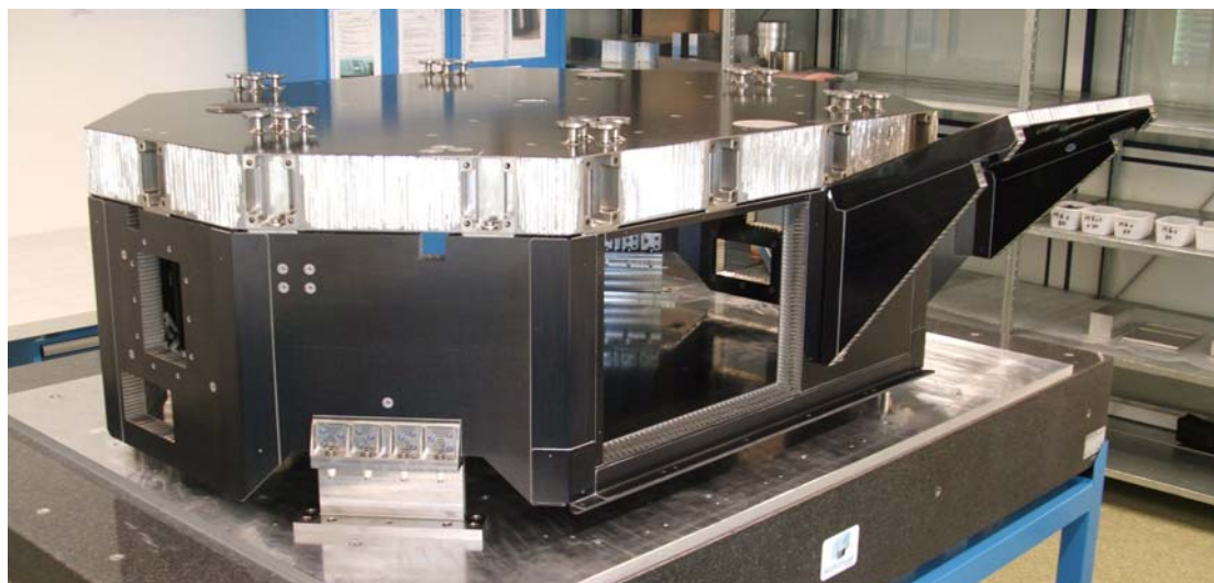
Figure 30.10-4 – ALADIN: Primary structure, proto-flight model (PFM)
