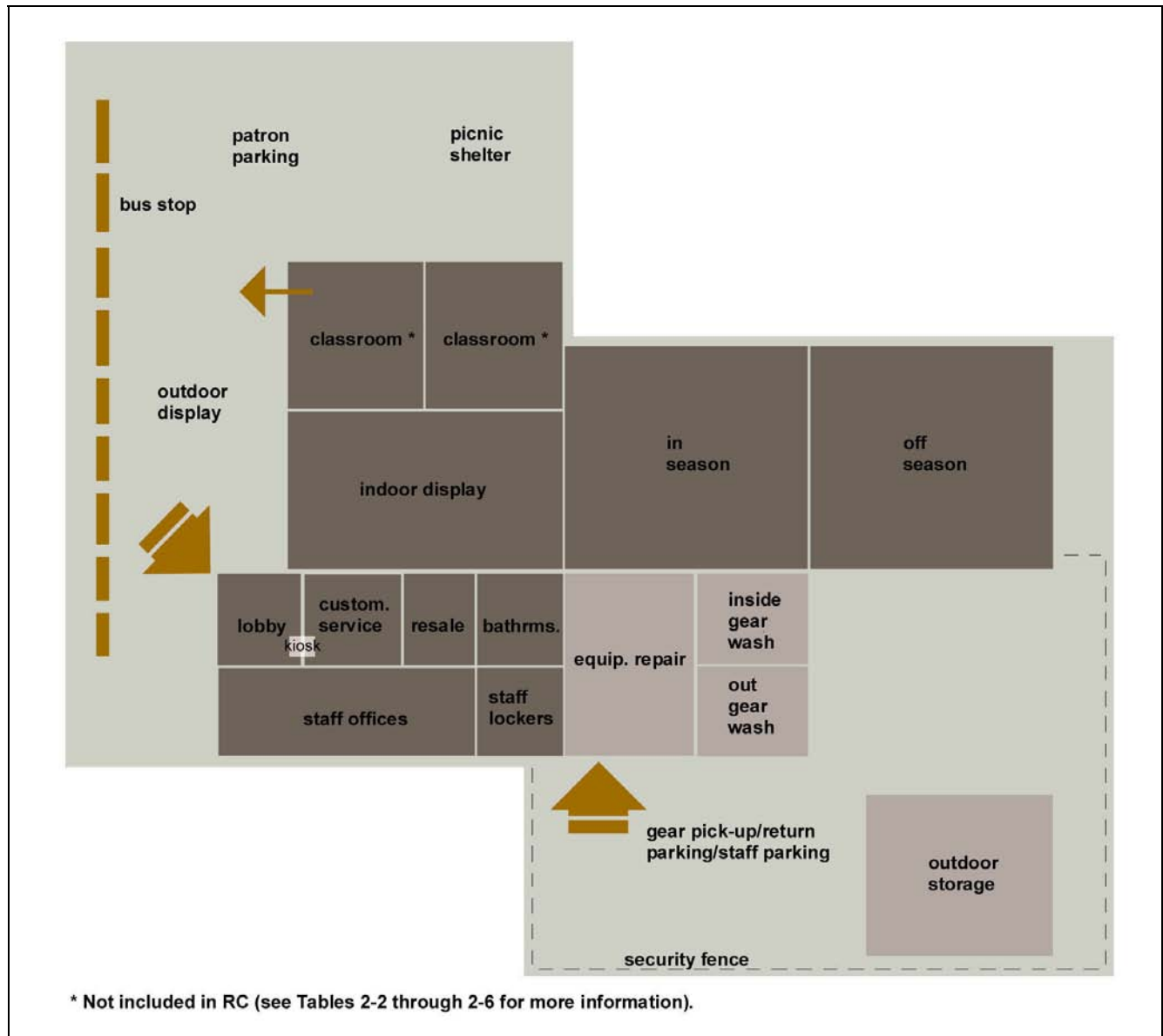
FIGURE 2-1. OAC AND RC FUNCTIONAL RELATIONSHIP BUBBLE DIAGRAM
