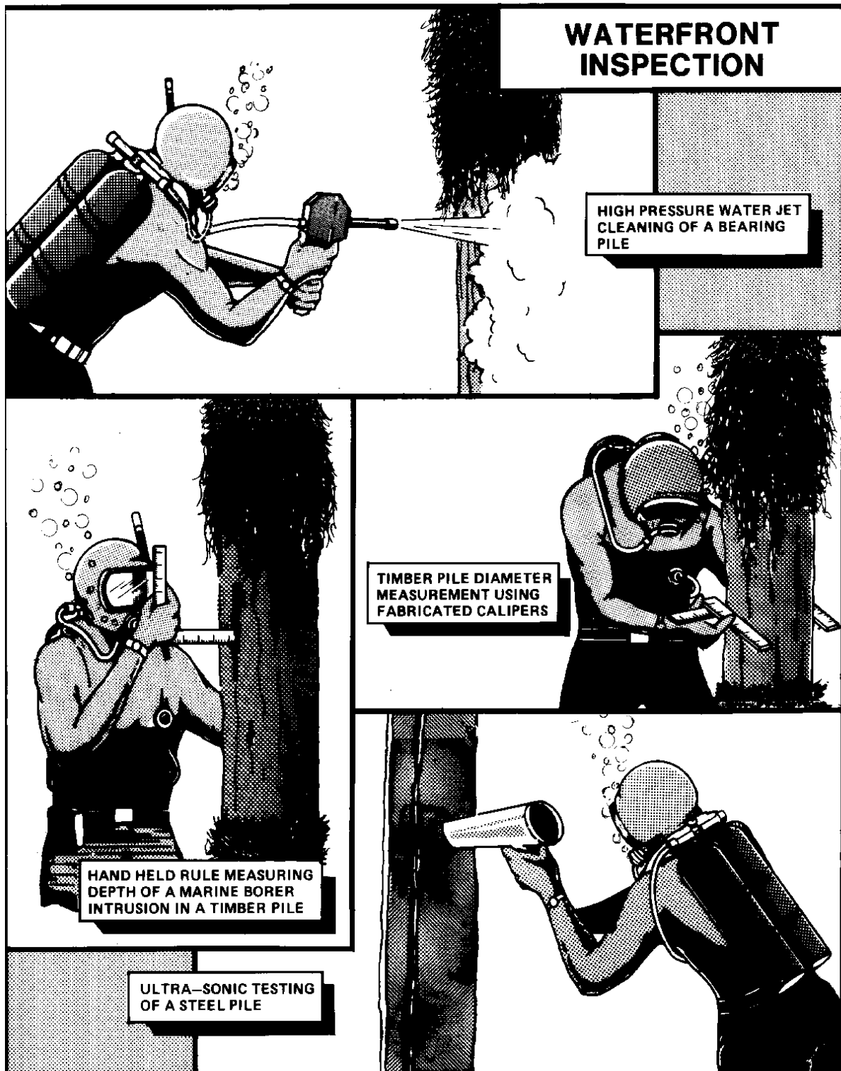
Figure 5-2 Tools and Equipment Used for Waterfront Inspection
