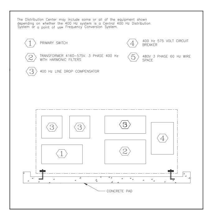
Figure 10 Feeder Distribution Center
