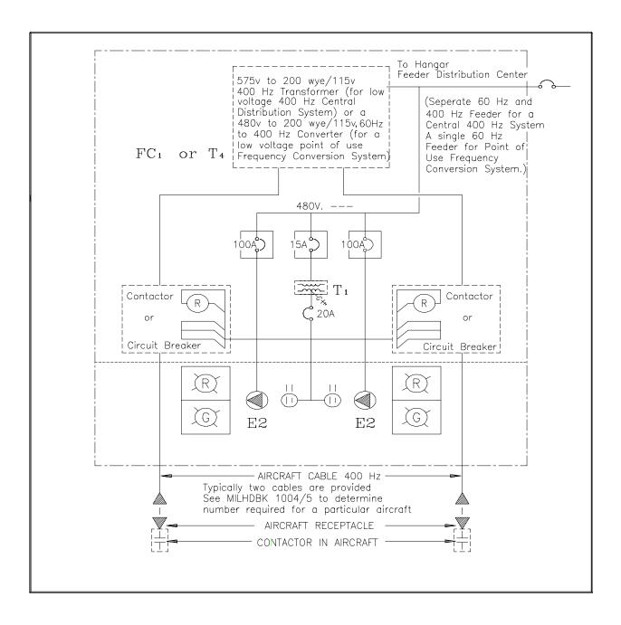
Figure 9 Typical Hangar Service Point Electrical One-Line Diagram
