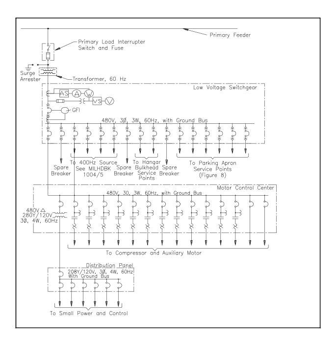
Figure 7 Typical One Line Diagram Central Facilities Air Start System
