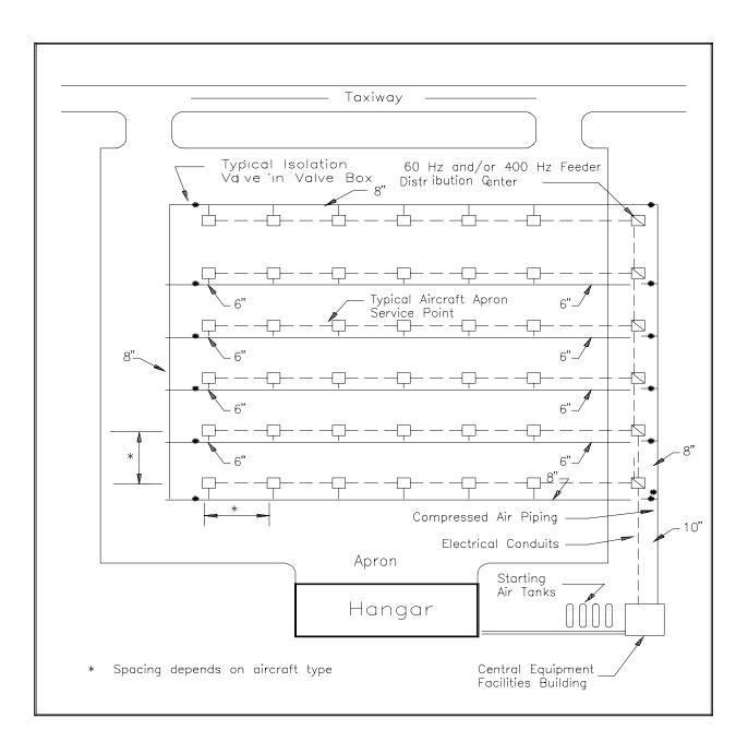
Figure 1 Typical FPUS Site Plan
