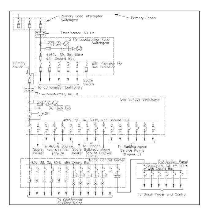
Figure 6 Typical One Line Diagram Central Facilities - ECS System
