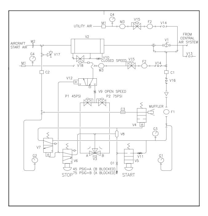
Figure 13 Aircraft Service Console Mechanical Schematic
