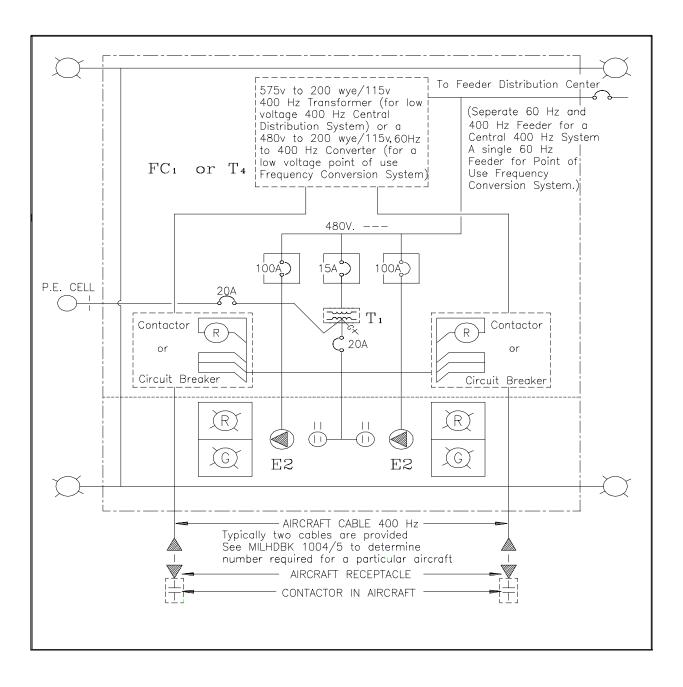
Figure 8 Typical Parking Apron Service Point Electrical One-Line Diagram
