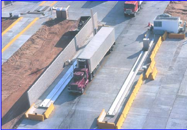
Figure 7-4 VACIS II - Gamma Ray Imaging System
