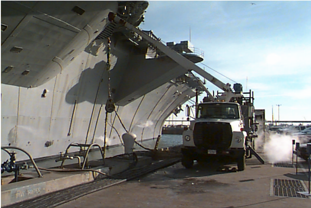
Picture K. A cable being reeled by a boom truck.
