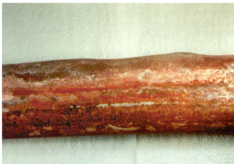
Figure 3-7. Metal Fatigue on Boiler Tube
