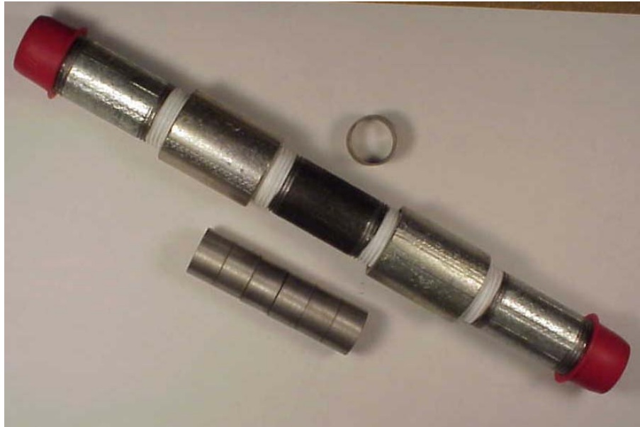
Figure D-1. Condensate Corrosion Tester
