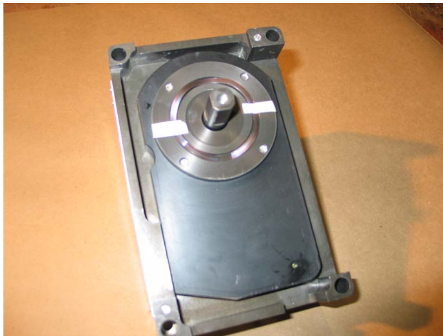
Figure D-6. Installation of ILD shutter plate wave spring
