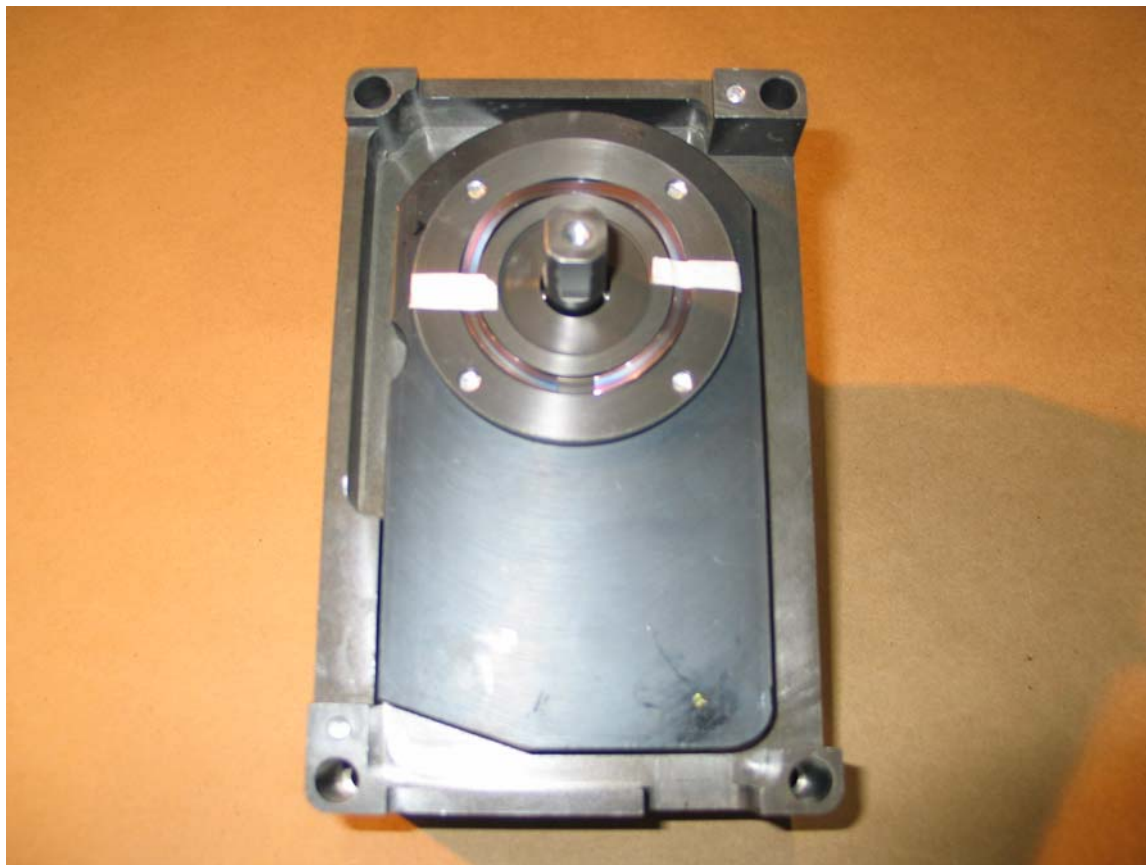
Figure D-11. Installation of ILD shutter plate wave spring
