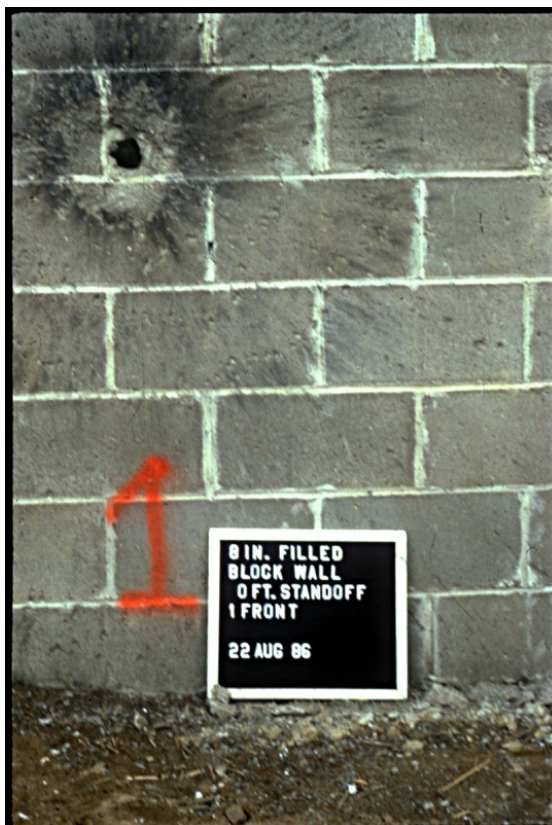
Figure 2-3. Shaped Charge Penetration of Masonry
