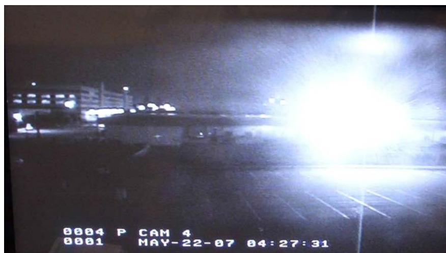
Figure 4-3. Effect of Glare on CCTV Camera Image Quality.
