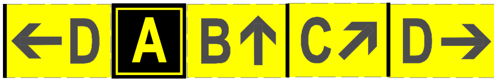
POSITION OF A LOCATION SIGN IN AN ARRAY OF DIRECTION SIGNS
