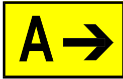
RUNWAY EXIT SIGN
