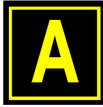
TAXIWAY LOCATION SIGN
