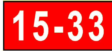
RUNWAY HOLD SIGN (AT INTERMEDIATE INTERSECTION)
