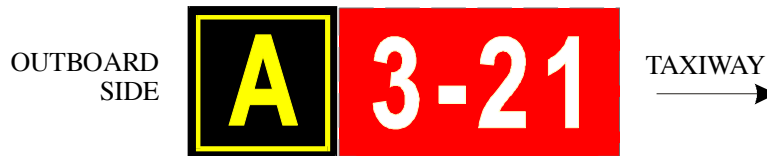
LOCATION SIGN COLLOCATED WITH A RUNWAY HOLD SIGN
