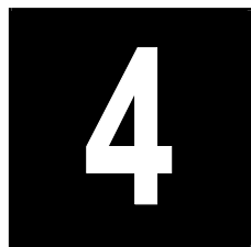
RUNWAY DISTANCE REMAINING MARKER (RDM)
