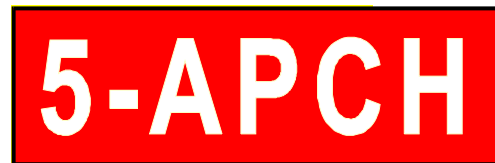
APPROACH HOLD SIGN (ON INTERSECTING TAXIWAY INTERSECTION)
