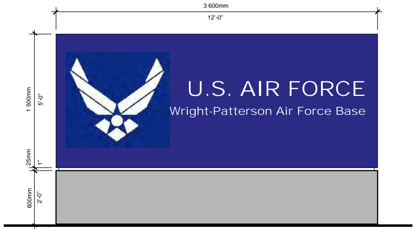
Figure 4.4. Main Entrance Sign Type A1 Dimensions.
