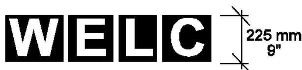
Figure 7.6. Changeable Letter Tile Dimensions.
