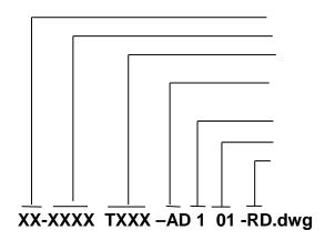
Fiscal Year of Construction Contract Construction Contract Number Task Order Number (if Applicable) Discipline Designator w/optional Level 2 Designator Sheet Type Sheet Sequence Identifier Record Drawing Suffix
