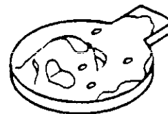
FIGURE 22. Plated-through holes - clinched lead and wires (see 5.7.19).
