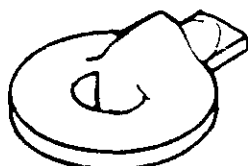
FIGURE 23. Nonplated-through hole - clinched leads and wires (see 5.7.19).
