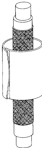
FIGURE 3 INSTALLING REPAIR SLEEVE (STEP 3)
